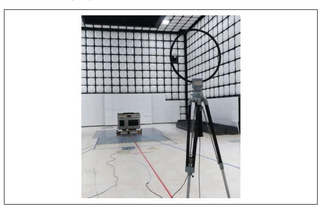
◆ Radiated Test Picture (Back): Below 30 MHz
