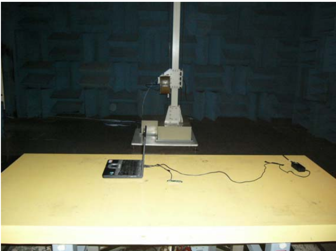
SIDE VIEW OF RADIATED MEASUREMENT
