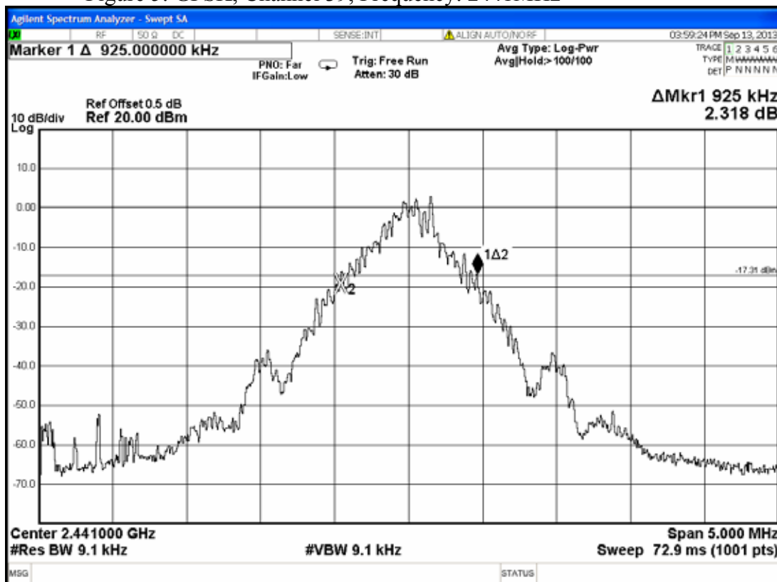
Figure 5: GFSK, Channel 39, Frequency: 2441MHz
