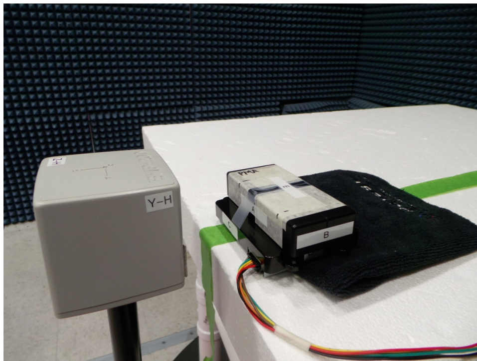
Figure 13. E-Field Measurement (Position C)
