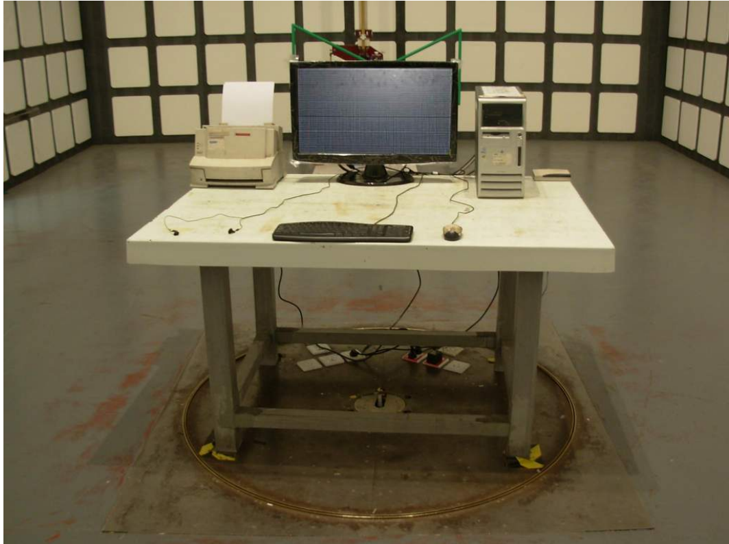
FRONT VIEW OF RADIATED EMISSION TEST
