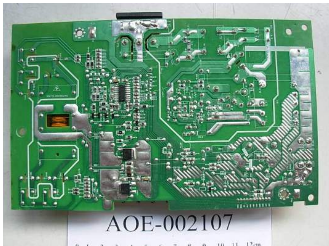
FIGURE 12 LCD MONITOR (M/N: W2361VV) POWER BOARD (SOLDERED SIDE)
