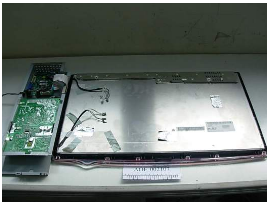
FIGURE 3 LCD MONITOR (M/N: W2361VV) BOARDS REMOVED
