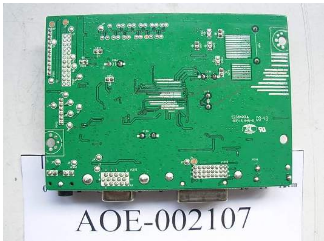
FIGURE 9 LCD MONITOR (M/N: W2361VV) MAIN BOARD (SOLDERED SIDE)
