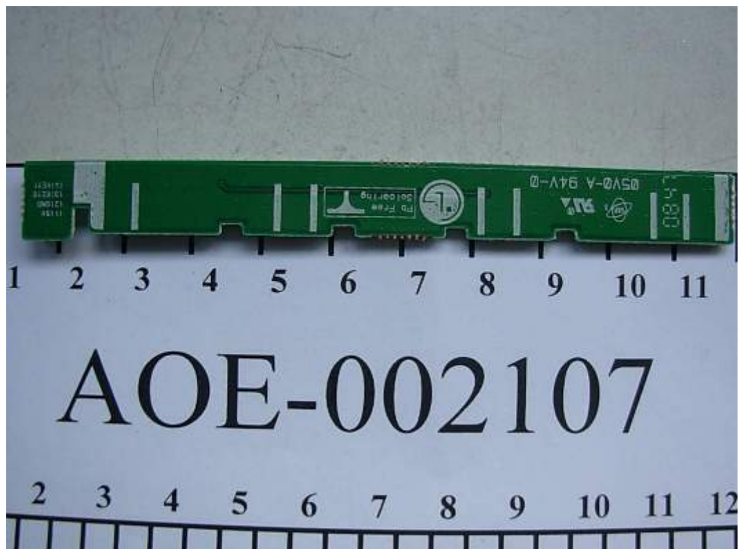
FIGURE 5 LCD MONITOR (M/N: W2361VV) KEYBOARD (SOLDERED SIDE)
