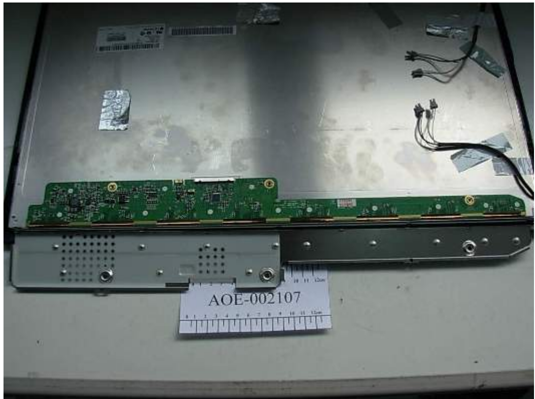
FIGURE 14 LCD MONITOR (M/N: W2361VV) LCD PANEL MAIN BOARD (COMPONENT SIDE)
