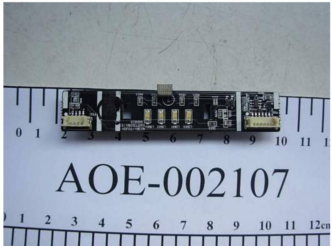
FIGURE 6 LCD MONITOR (M/N: W2361VV) LED BOARD (COMPONENT SIDE)
