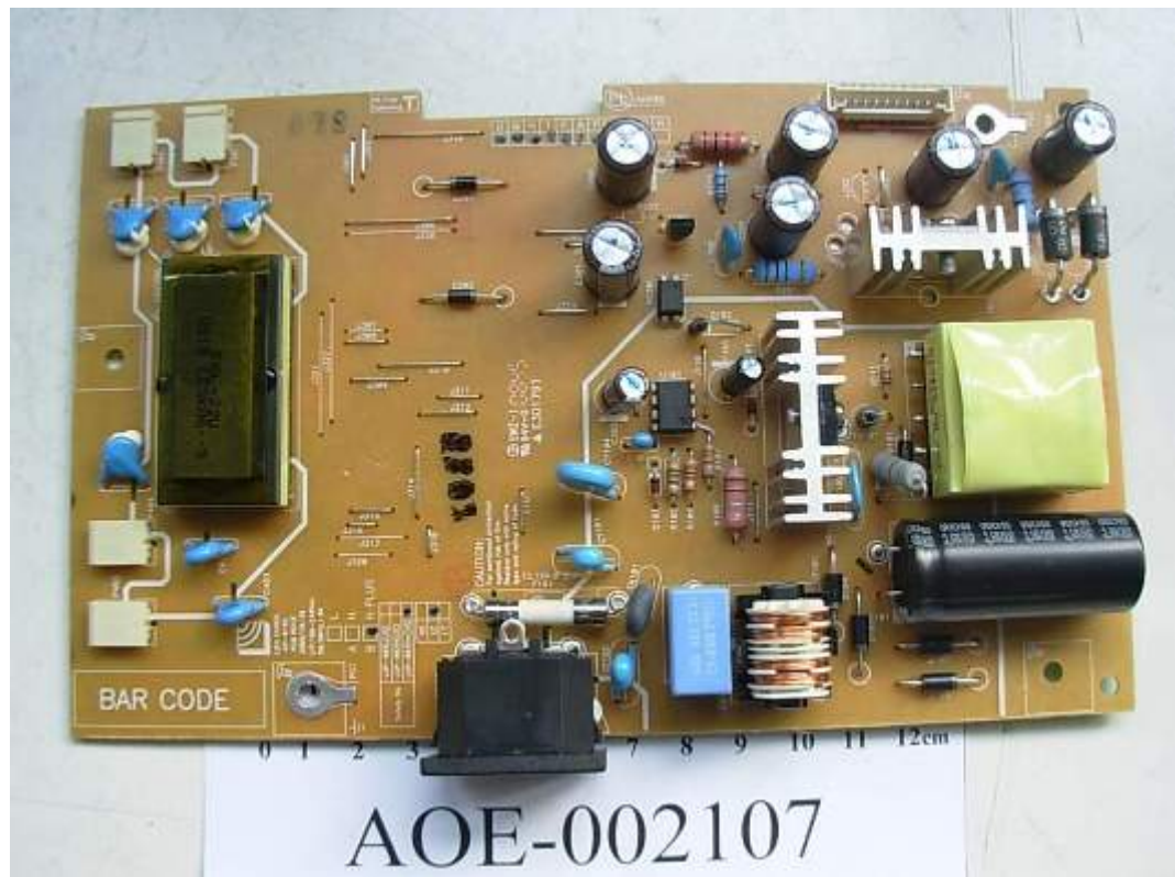
FIGURE 11 LCD MONITOR (M/N: W2361VV) POWER BOARD (COMPONENT SIDE)
