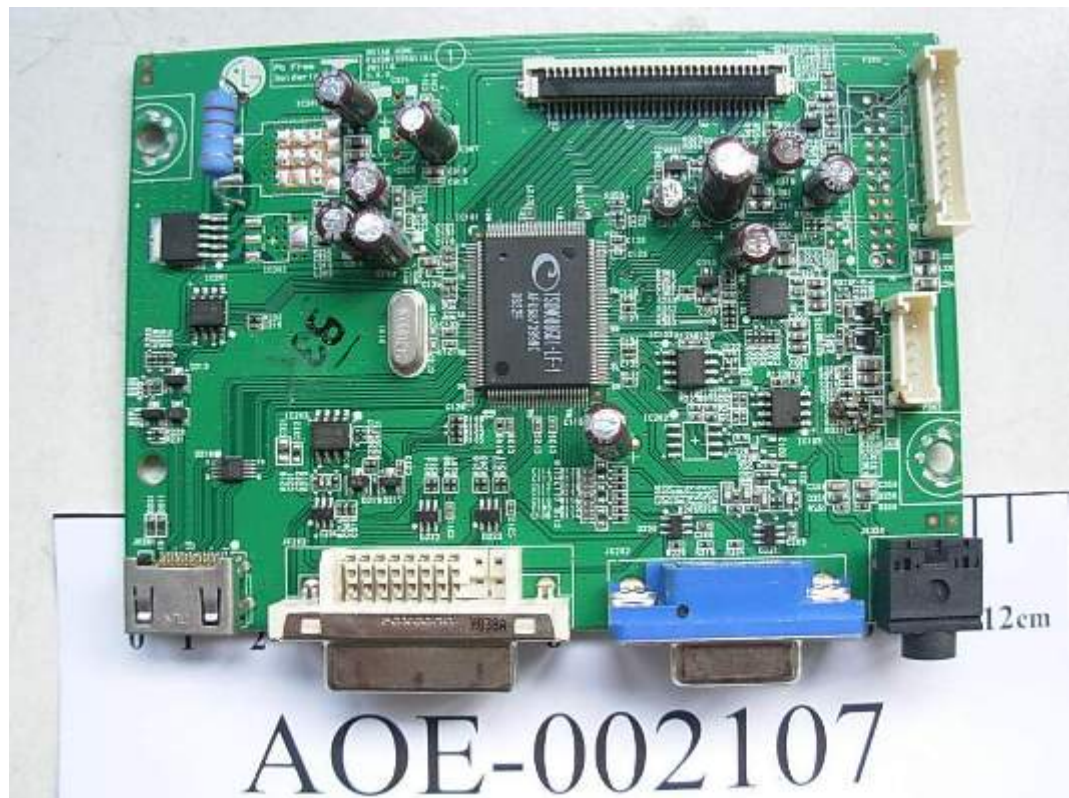
FIGURE 8 LCD MONITOR (M/N: W2361VV) MAIN BOARD (COMPONENT SIDE)
