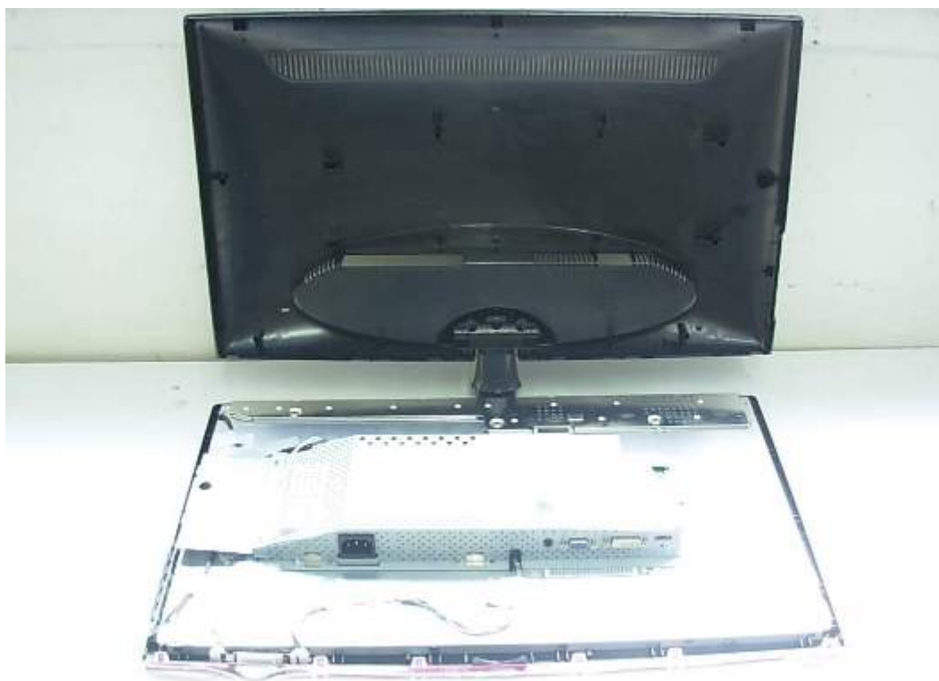
FIGURE 1 LCD MONITOR (M/N: W2361VV) COVER REMOVED
