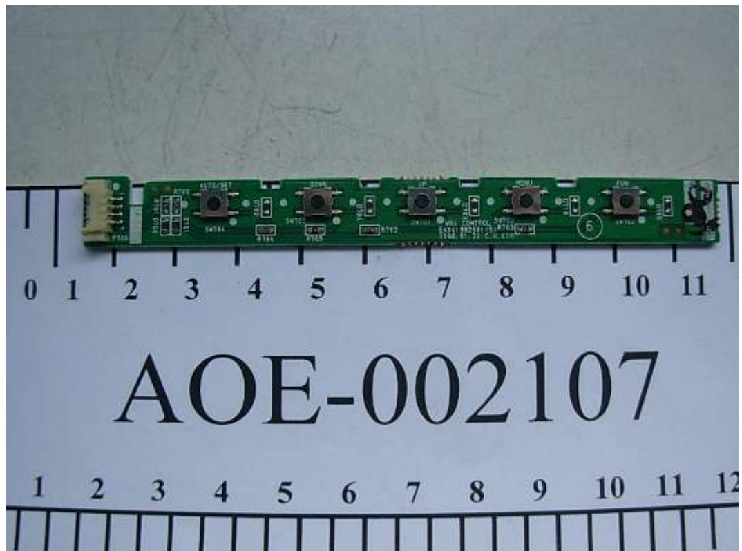
FIGURE 4 LCD MONITOR (M/N: W2361VV) KEYBOARD (COMPONENT SIDE)
