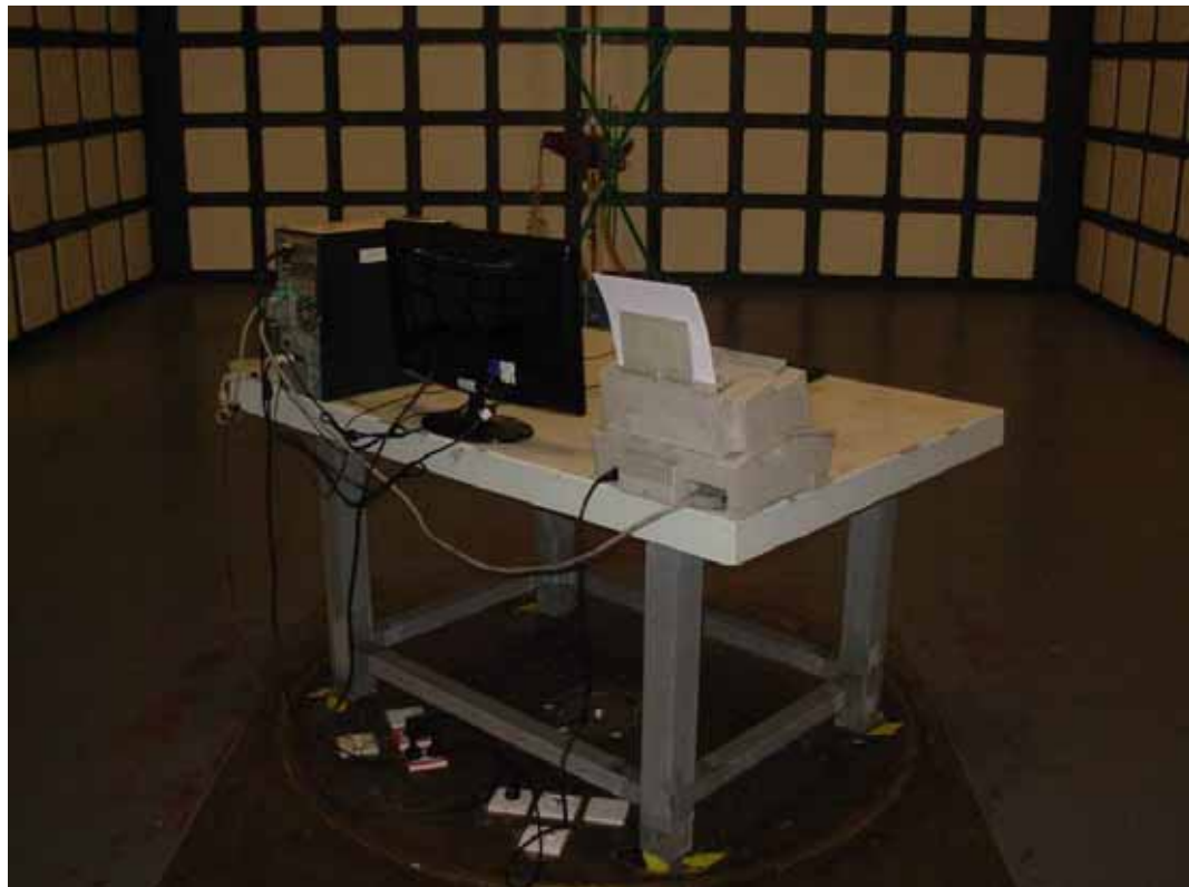
SETUP WITH MAXIMUM DETECTED EMISSION AT VERTICAL POLARIZATION (DVI 1920*1080@60Hz)
