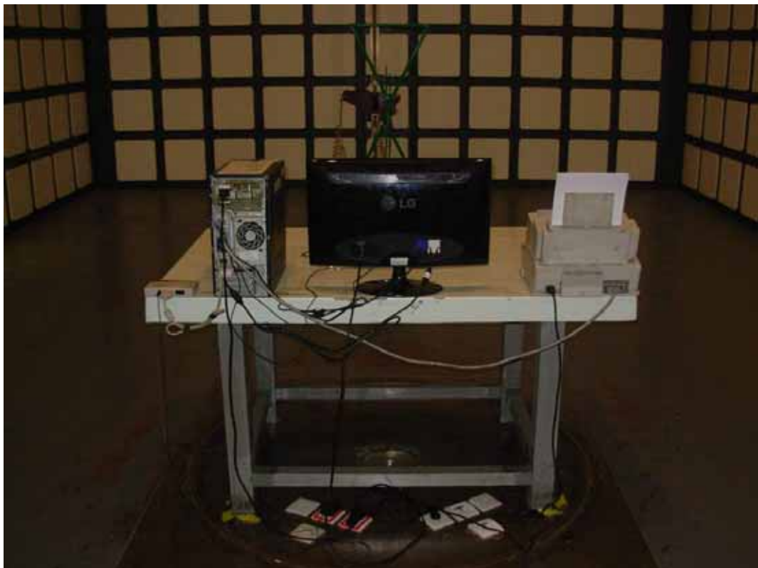
BACK VIEW OF RADIATED EMISSION TEST
