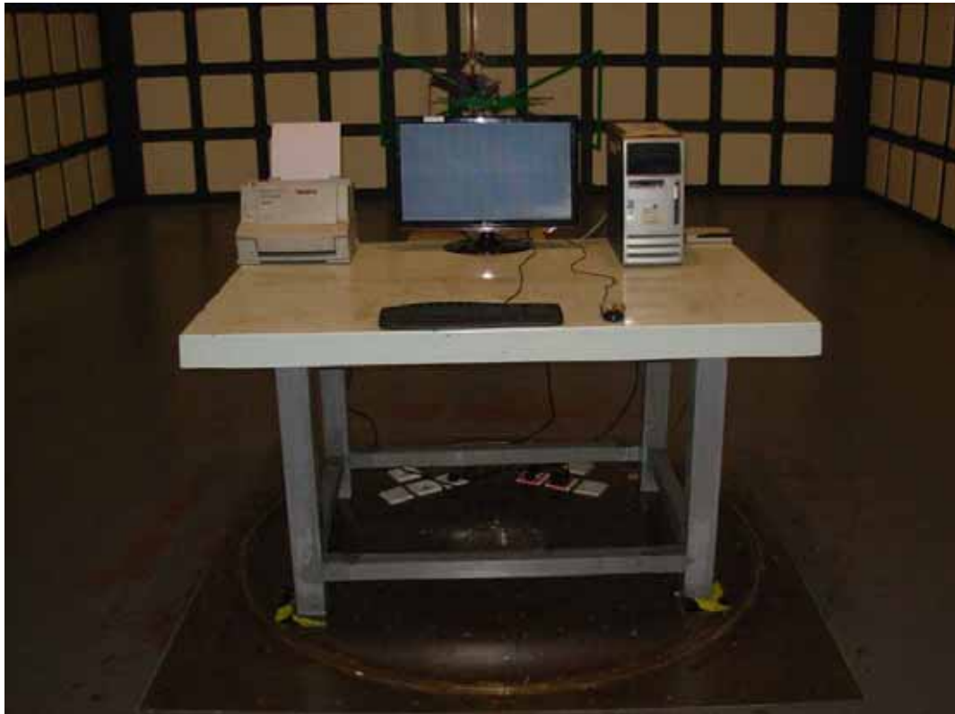
FRONT VIEW OF RADIATED EMISSION TEST
