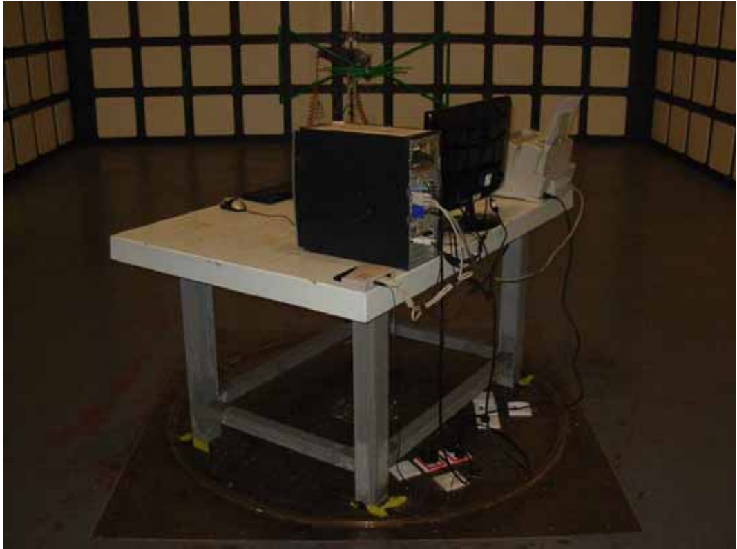
SETUP WITH MAXIMUM DETECTED EMISSION AT HORIZONTAL POLARIZATION (DVI 1920*1080@60Hz)
