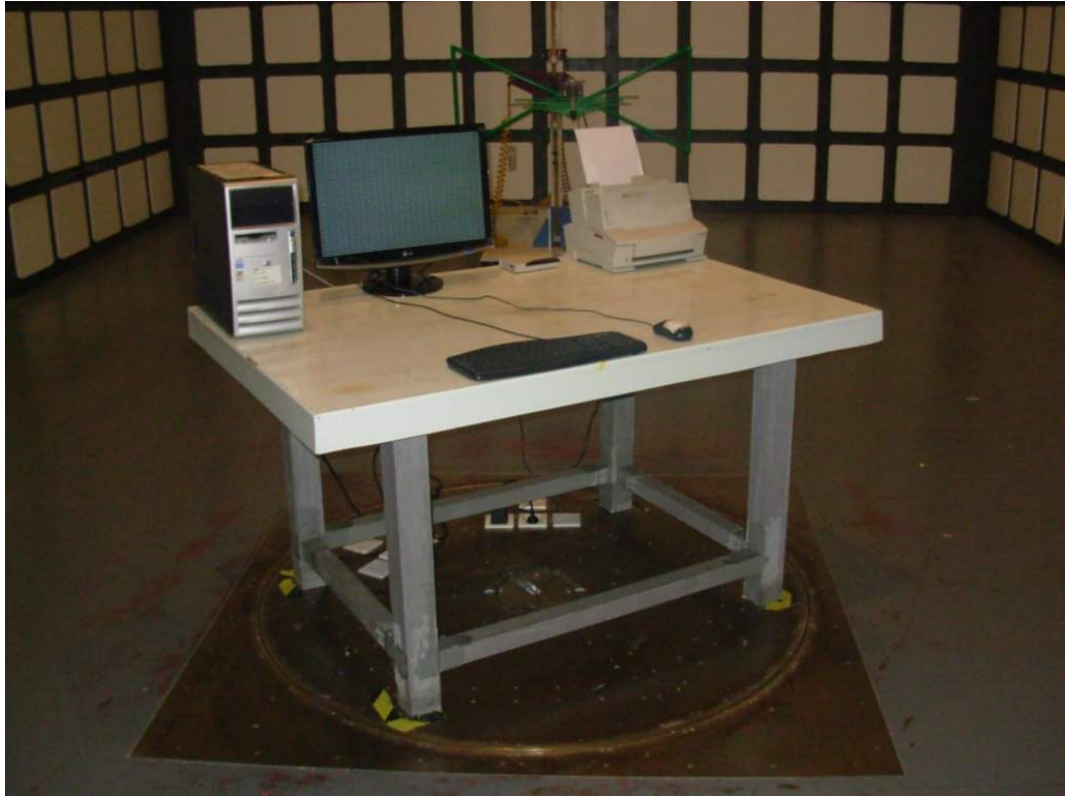
SETUP WITH MAXIMUM DETECTED EMISSION AT HORIZONTAL POLARIZATION (VGA 1024*768@60Hz)
