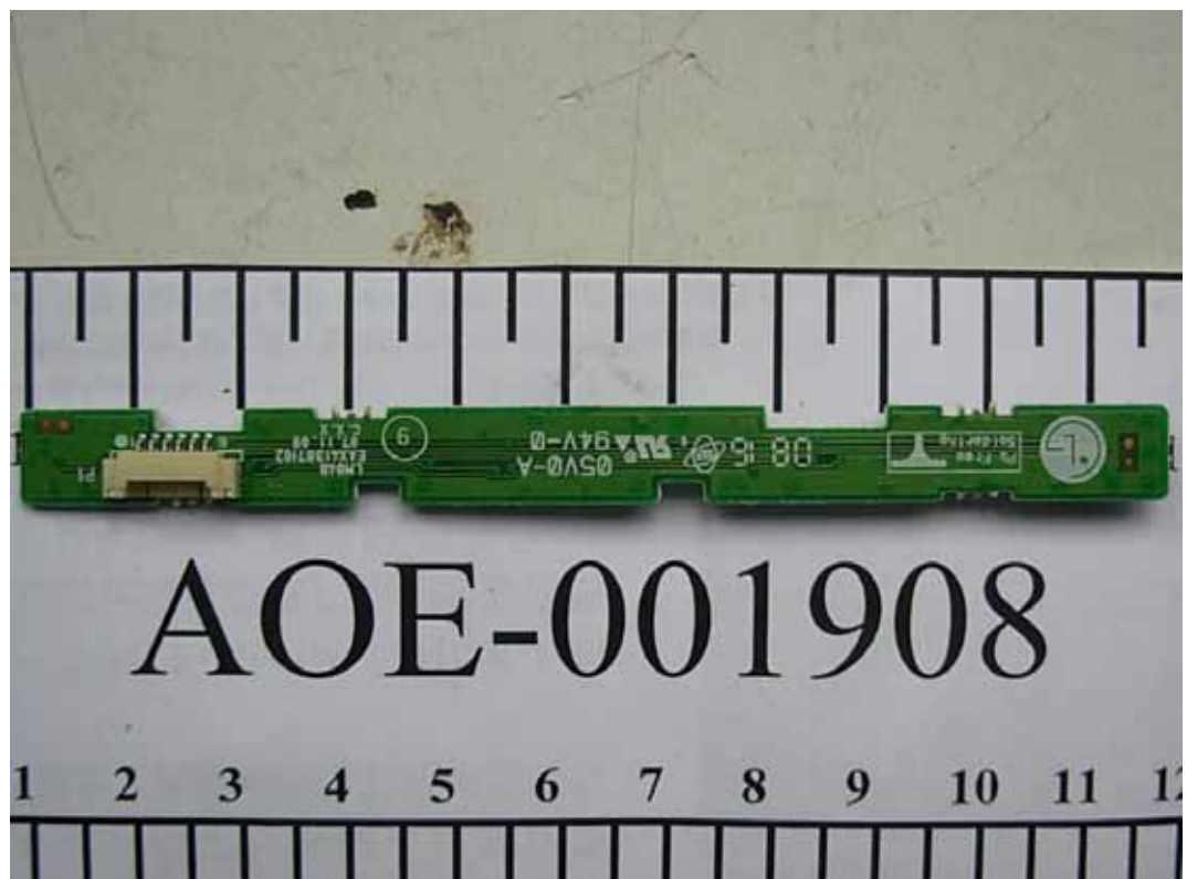
FIGURE 20 LCD MONITOR (M/N: W2252TET) KEY BOARD (SOLDERED SIDE)
