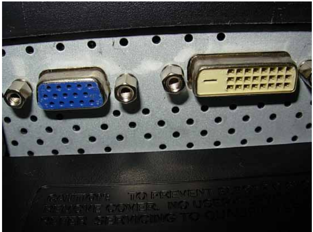
FIGURE 5 LCD MONITOR (M/N: W2244TV) SIGNAL PORT
