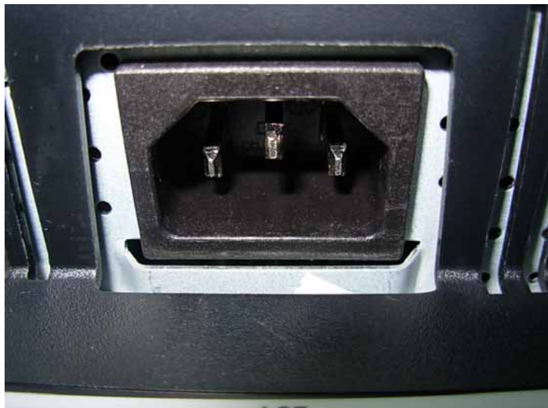
FIGURE 4 LCD MONITOR (M/N: W2244TV) POWER PORT
