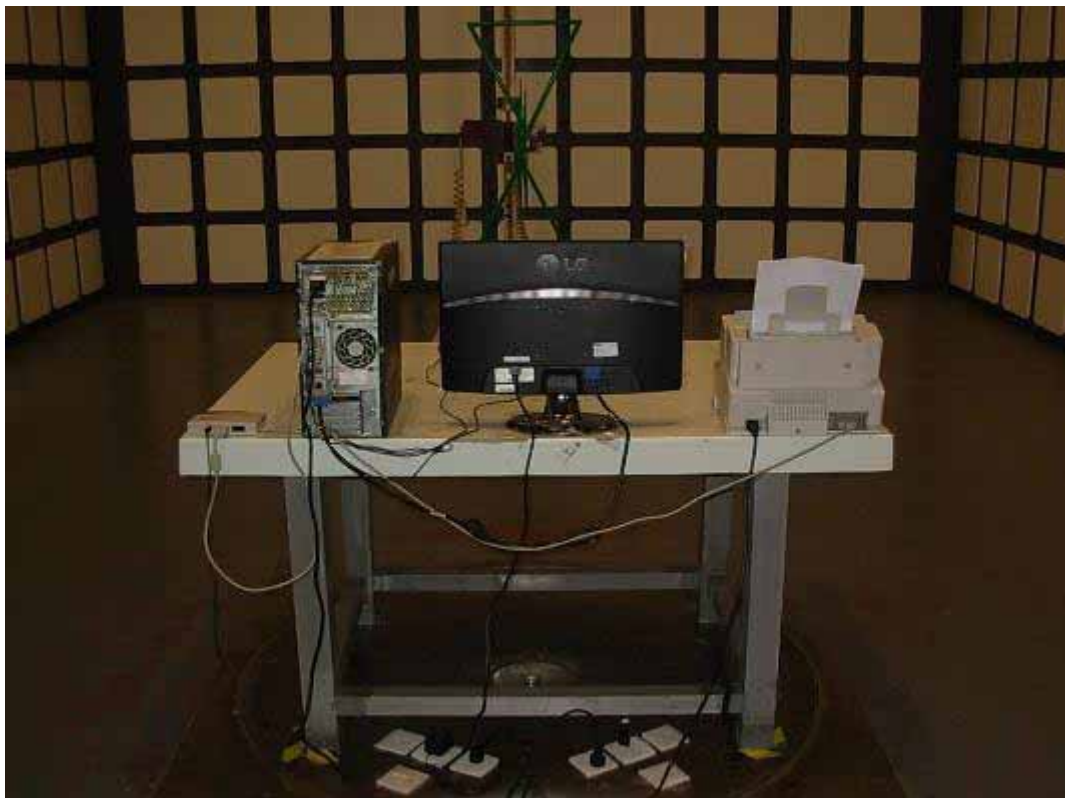
BACK VIEW OF RADIATED EMISSION TEST
