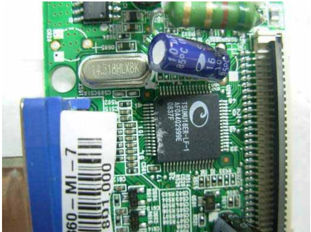
FIGURE 7 LCD MONITOR (M/N: W2243SV) CHIP & CRYSTAL ON MAIN BOARD
