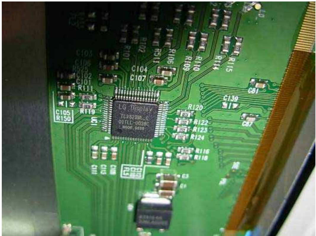
FIGURE 14 LCD MONITOR (M/N: W2243SV) CHIP ON LCD PANEL MAIN BOARD
