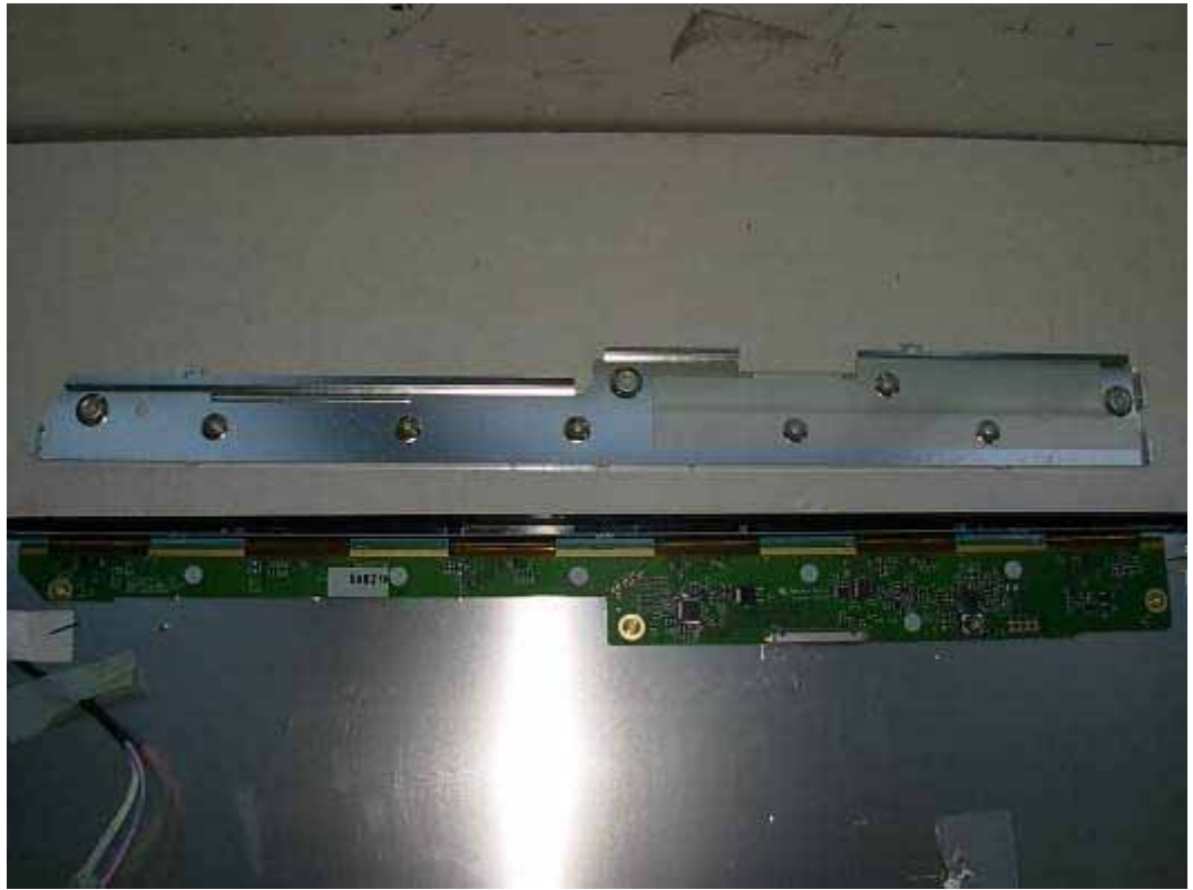
FIGURE 12 LCD MONITOR (M/N: W2243SV) LCD PANEL MAIN BOARD (COMPONENT SIDE)
