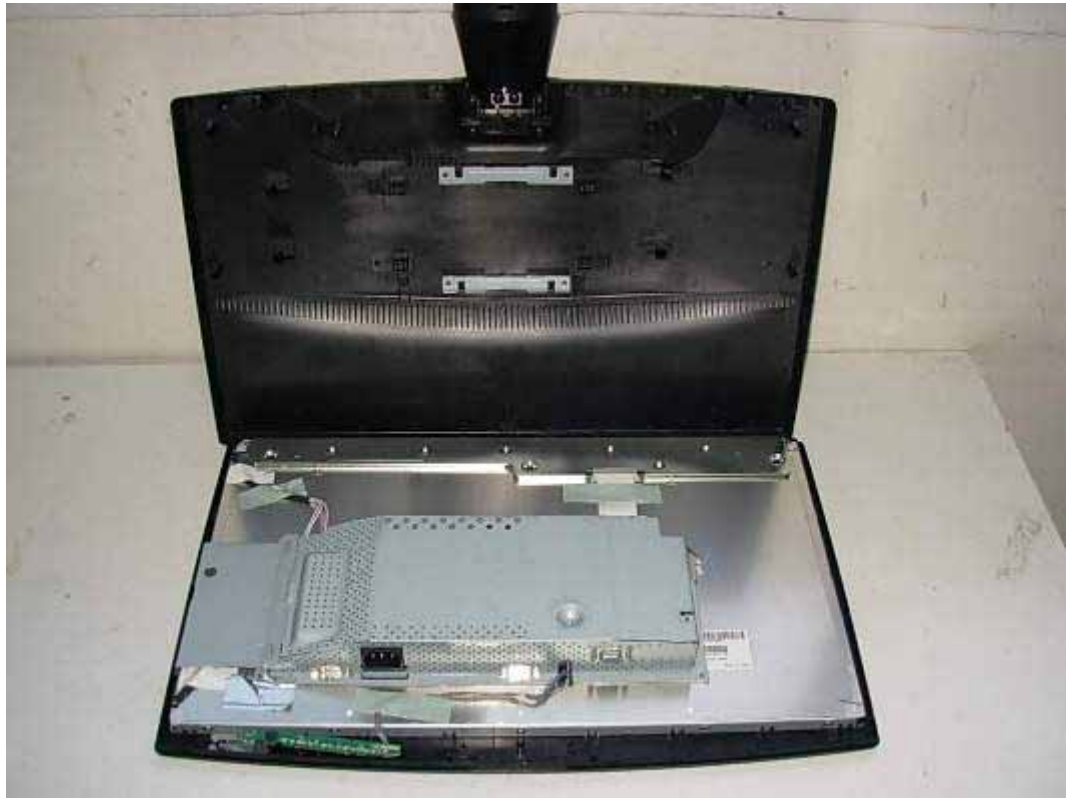
FIGURE 1 LCD MONITOR (M/N: W2243SV) COVER REMOVED
