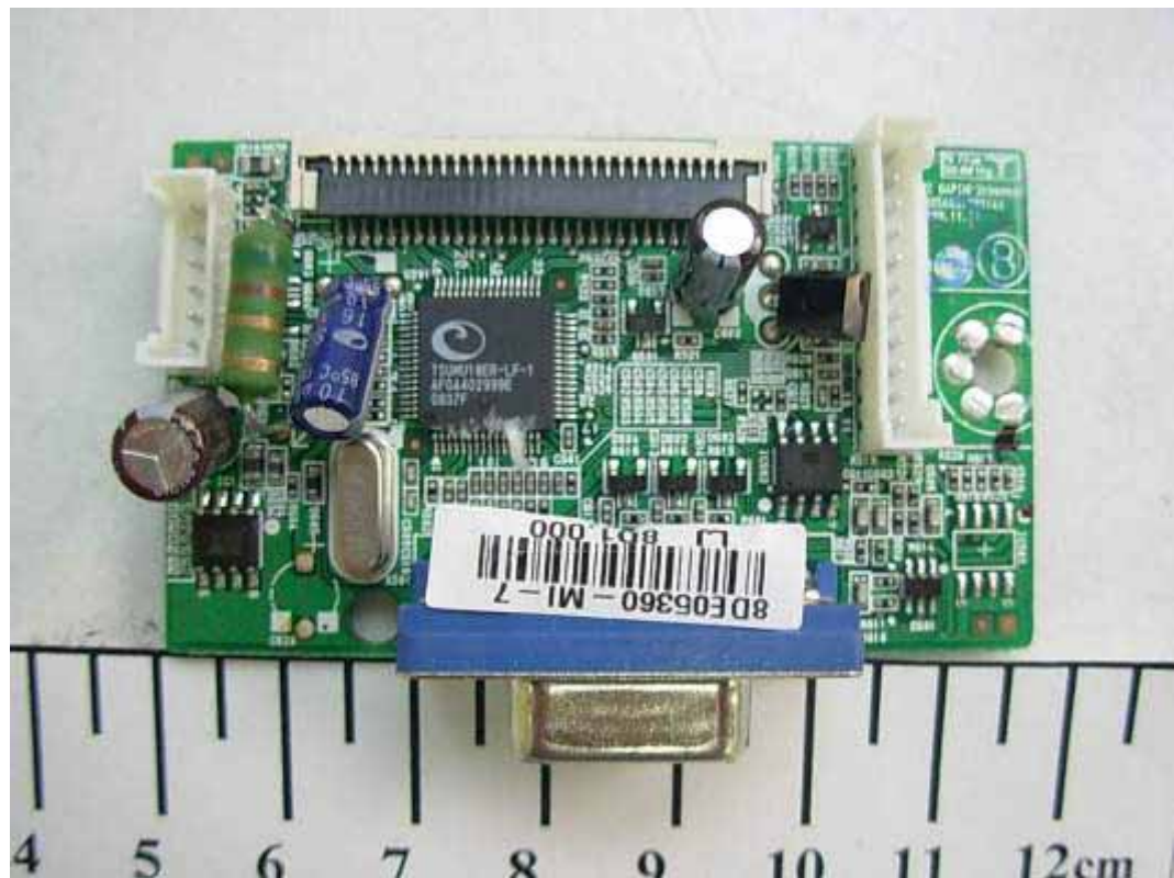
FIGURE 5 LCD MONITOR (M/N: W2243SV) MAIN BOARD (COMPONENT SIDE)
