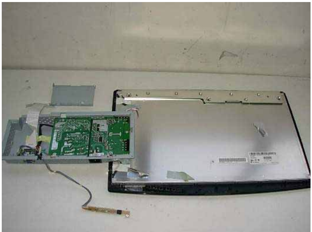
FIGURE 2 LCD MONITOR (M/N: W2243SV) BOARDS REMOVED
