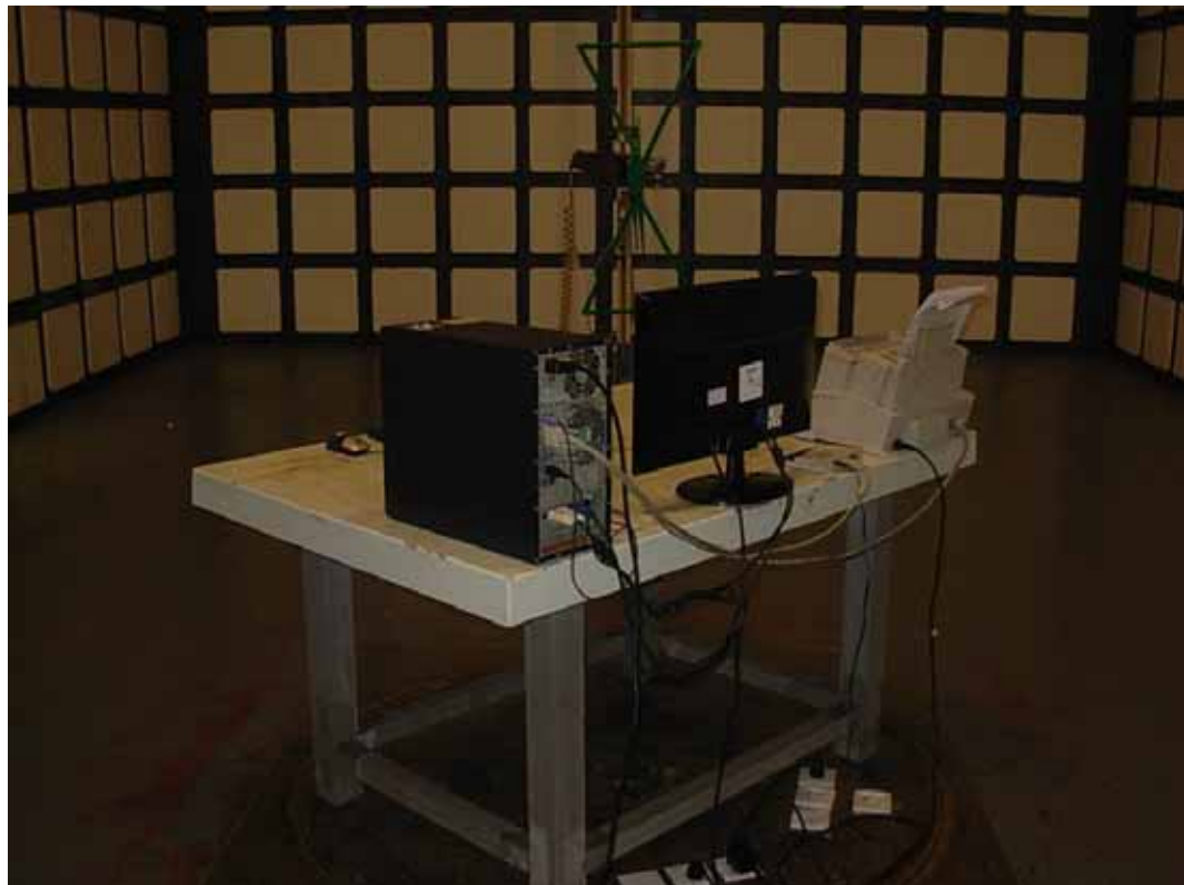
SETUP WITH MAXIMUM DETECTED EMISSION AT VERTICAL POLARIZATION (TEST MODE: DVI 1680*1050@60Hz)
