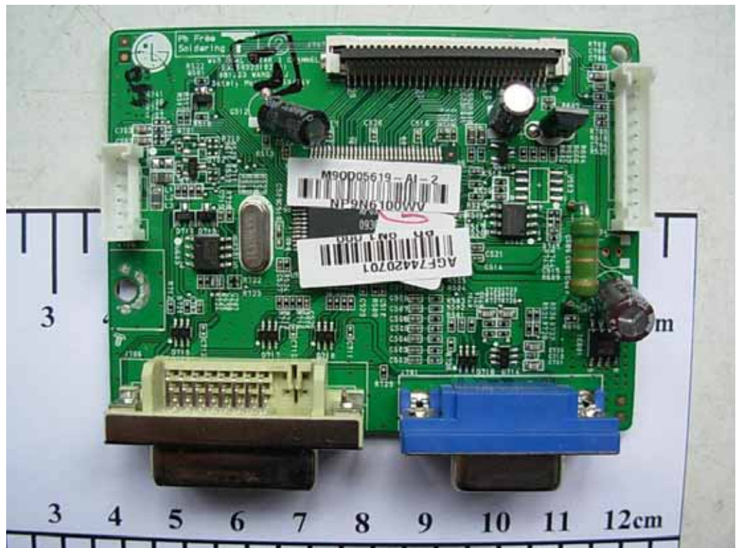
FIGURE 7 LCD MONITOR (M/N: W2240TV) MAIN BOARD (COMPONENT SIDE)
