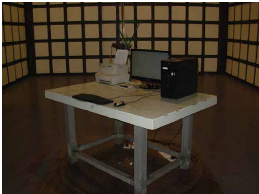
SETUP WITH MAXIMUM DETECTED EMISSION AT VERTICAL POLARIZATION (D-SUB 1600*900@60Hz)
