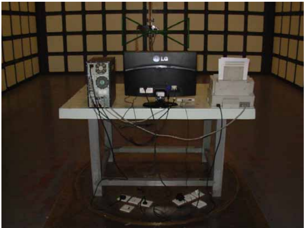
BACK VIEW OF RADIATED EMISSION TEST
