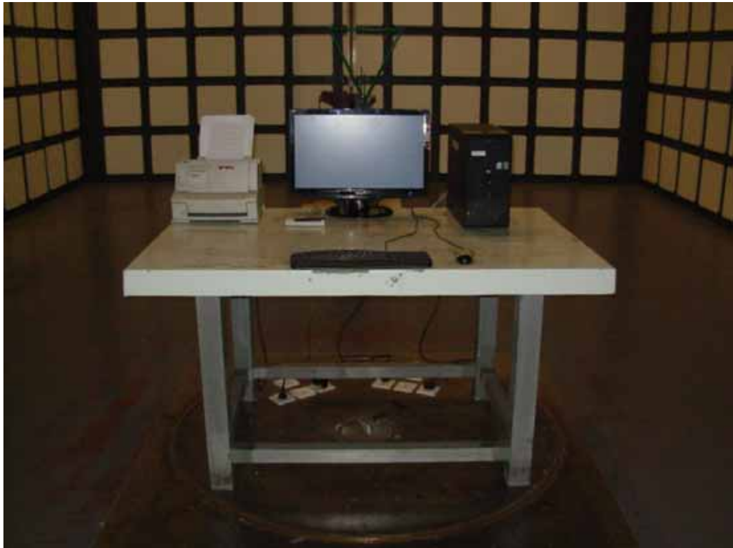
FRONT VIEW OF RADIATED EMISSION TEST
