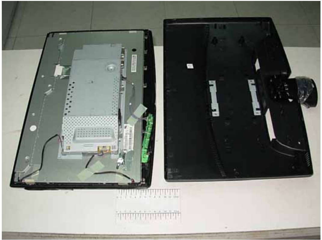
FIGURE 1 LCD MONITOR (M/N: W2044TV) COVER REMOVED
