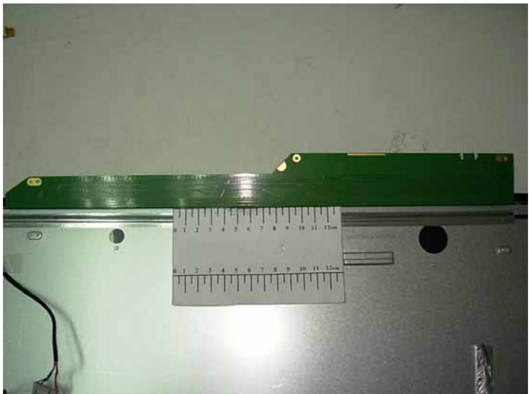
FIGURE 11 LCD MONITOR (M/N: W2044TV) LCD PANEL MAIN BOARD (SOLDERED SIDE)
