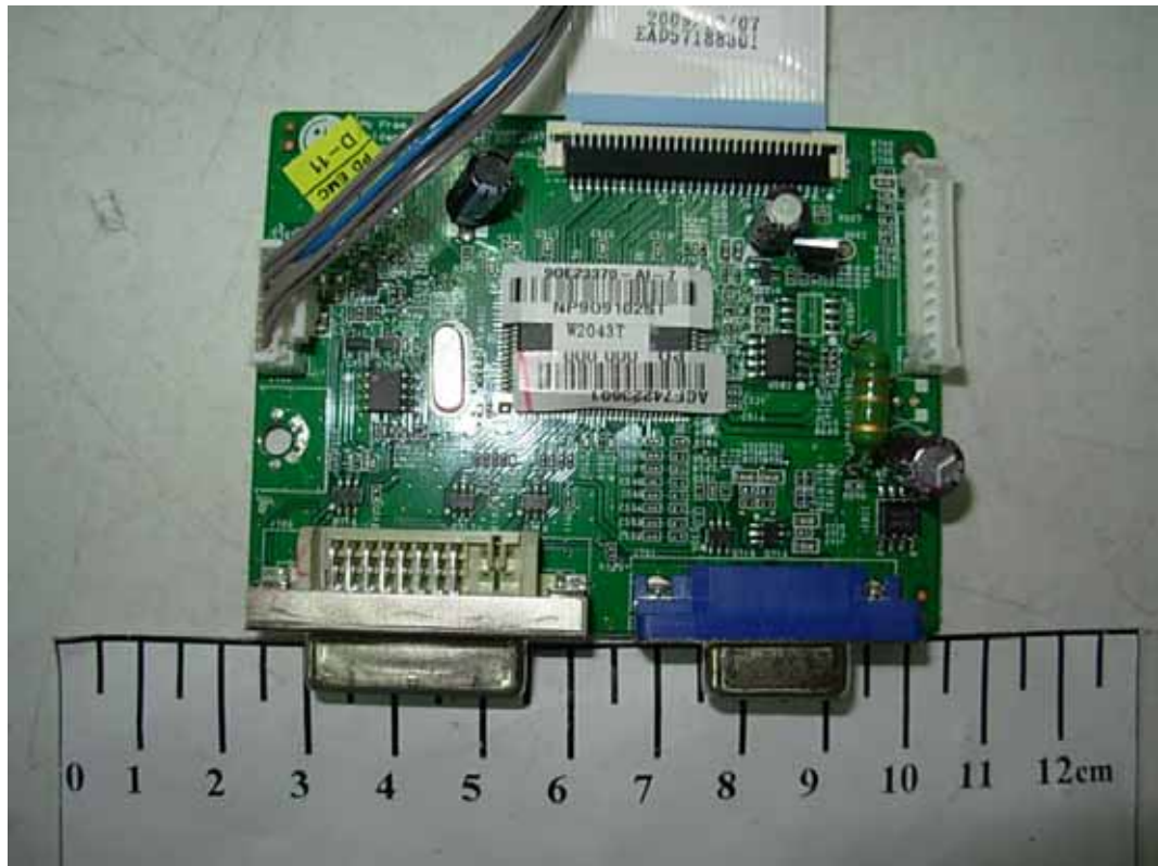
FIGURE 4 LCD MONITOR (M/N: W2044TV) MAIN BOARD (COMPONENT SIDE)
