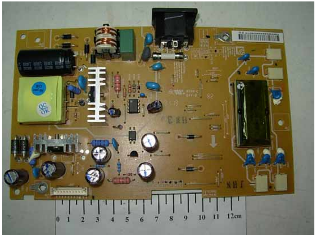
FIGURE 8 LCD MONITOR (M/N: W2044TV) POWER BOARD (COMPONENT SIDE)
