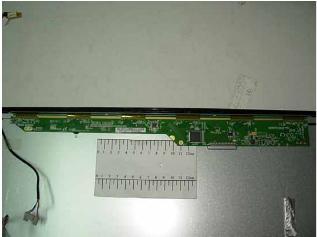
FIGURE 10 LCD MONITOR (M/N: W2044TV) LCD PANEL MAIN BOARD (COMPONENT SIDE)
