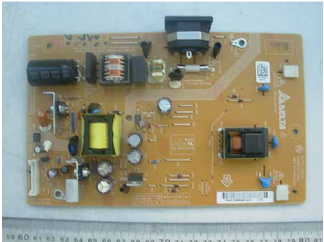
FIGURE 6 LCD MONITOR (M/N: W2043SEV) POWER BOARD (COMPONENT SIDE)
