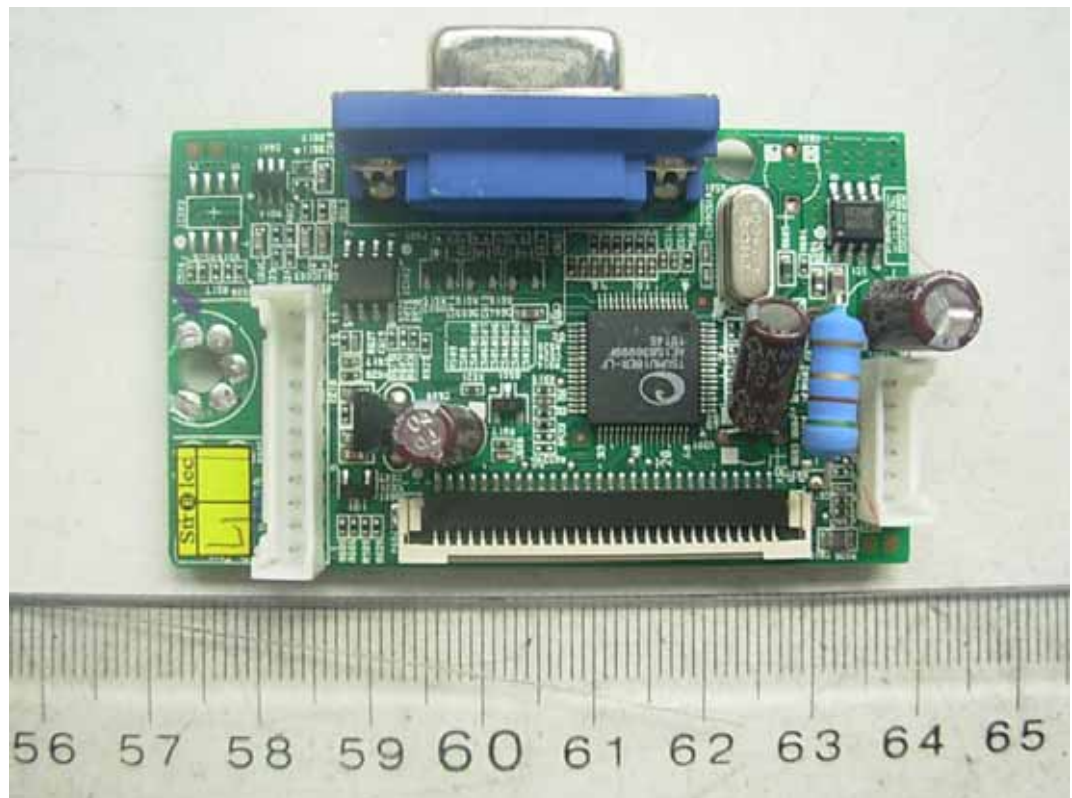
FIGURE 3 LCD MONITOR (M/N: W2043SEV) MAIN BOARD (COMPONENT SIDE)
