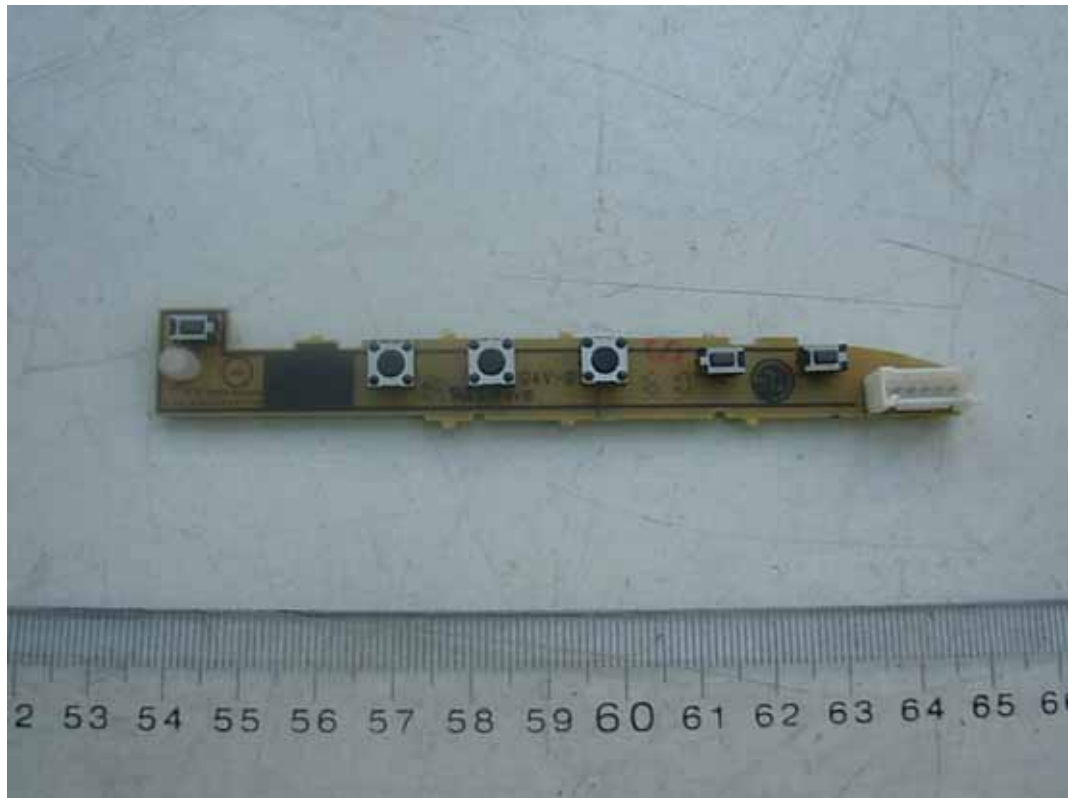
FIGURE 1 LCD MONITOR (M/N: W2043SEV) KEY BOARD (COMPONENT SIDE)
