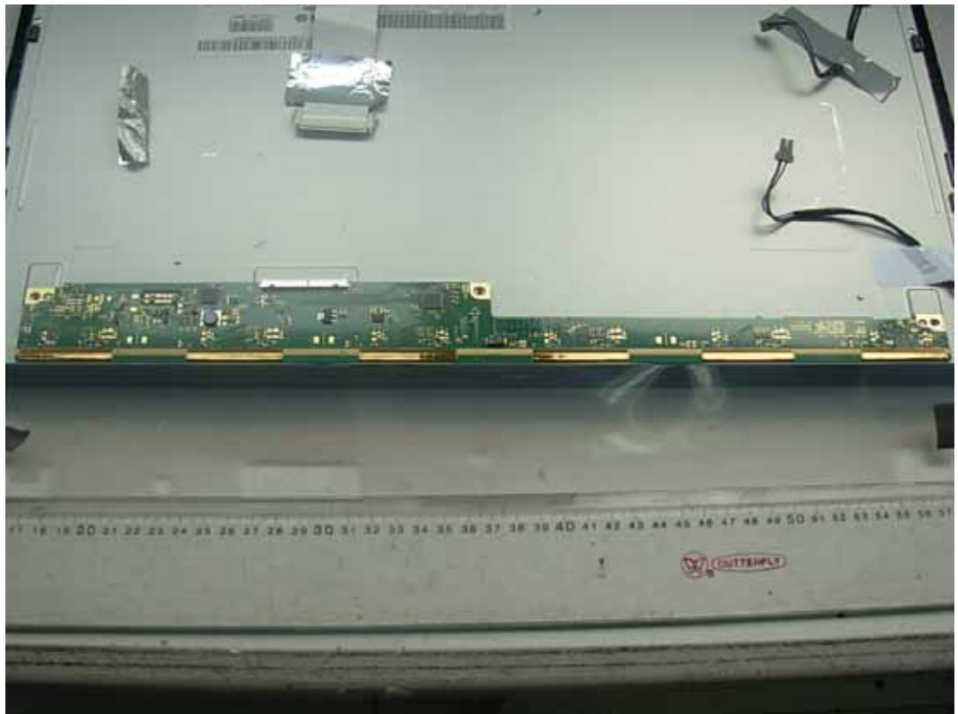
FIGURE 9 LCD MONITOR (M/N: W2043SEV) LCD PANEL MAIN BOARD (COMPONENT SIDE)
