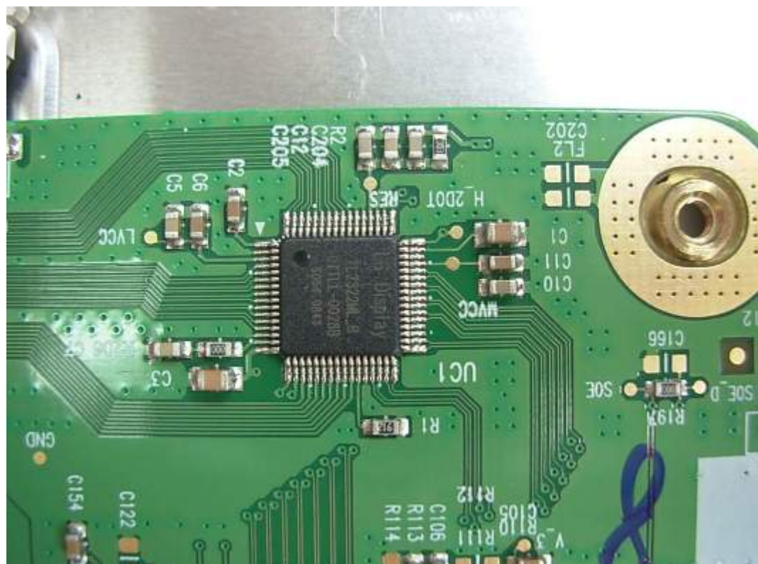
FIGURE 13 LCD MONITOR (M/N: W1954SQV) CHIP ON LCD PANEL MAIN BOARD
