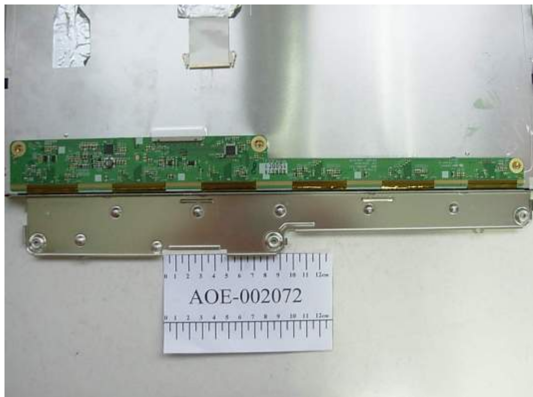
FIGURE 11 LCD MONITOR (M/N: W1954SQV) LCD PANEL MAIN BOARD SHIELDED SHELL REMOVED
