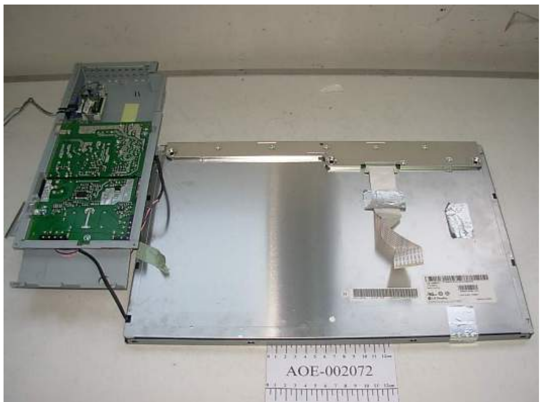
FIGURE 2 LCD MONITOR (M/N: W1954SQV) BOARDS REMOVED
