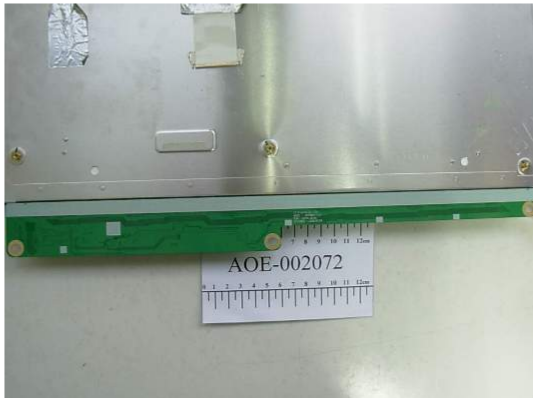
FIGURE 12 LCD MONITOR (M/N: W1954SQV) LCD PANEL MAIN BOARD (SOLDERED SIDE)
