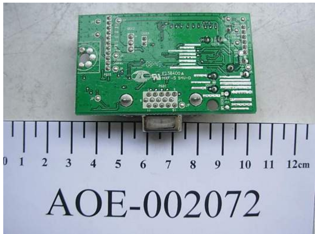
FIGURE 6 LCD MONITOR (M/N: W1954SQV) MAIN BOARD (SOLDERED SIDE)
