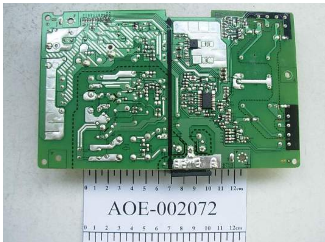
FIGURE 9 LCD MONITOR (M/N: W1954SQV) POWER BOARD (SOLDERED SIDE)
