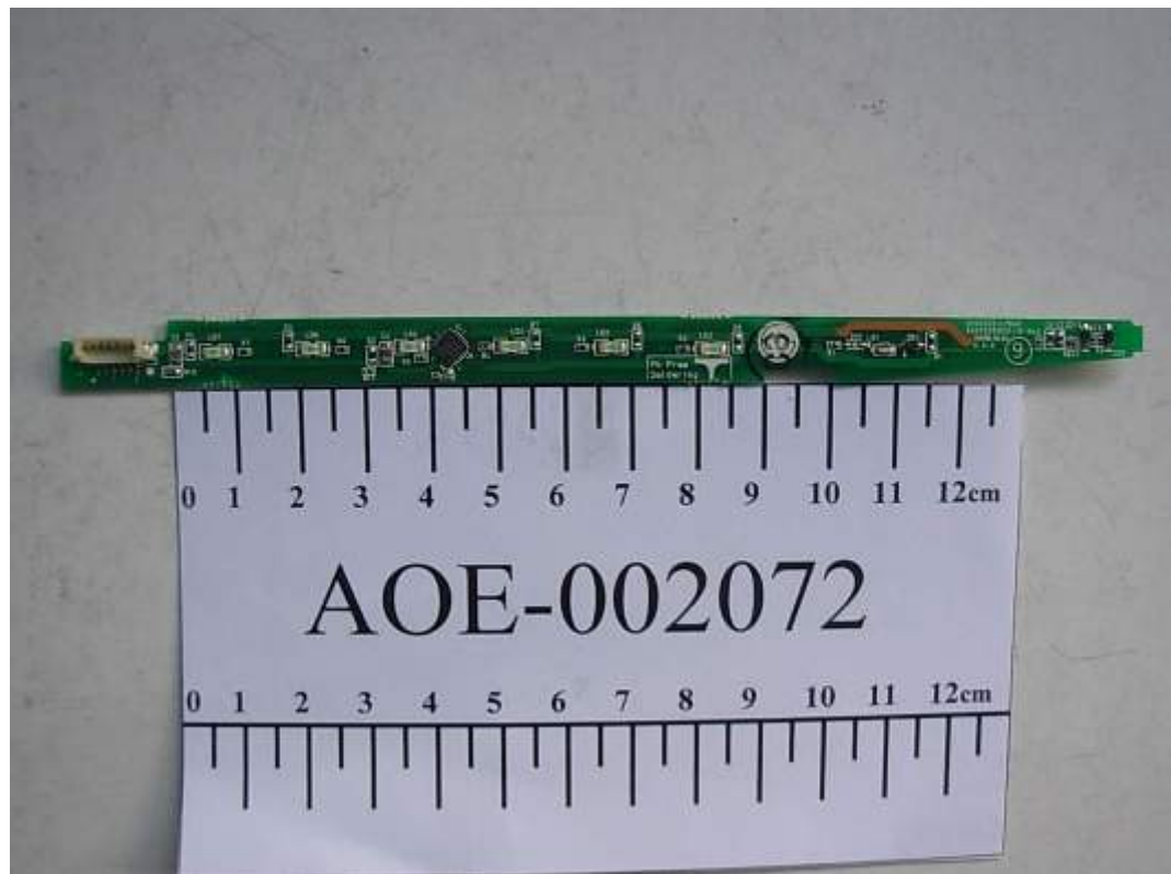
FIGURE 3 LCD MONITOR (M/N: W1954SQV) KEYBOARD (COMPONENT SIDE)
