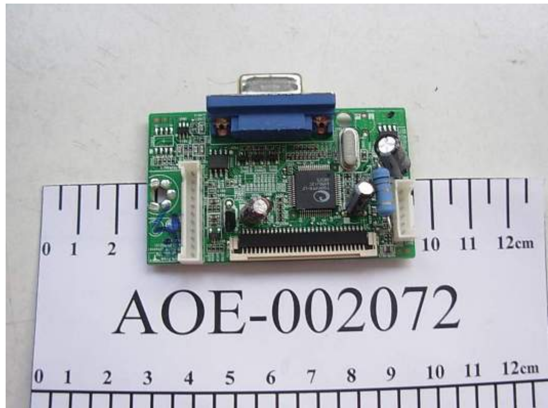
FIGURE 5 LCD MONITOR (M/N: W1954SQV) MAIN BOARD (COMPONENT SIDE)
