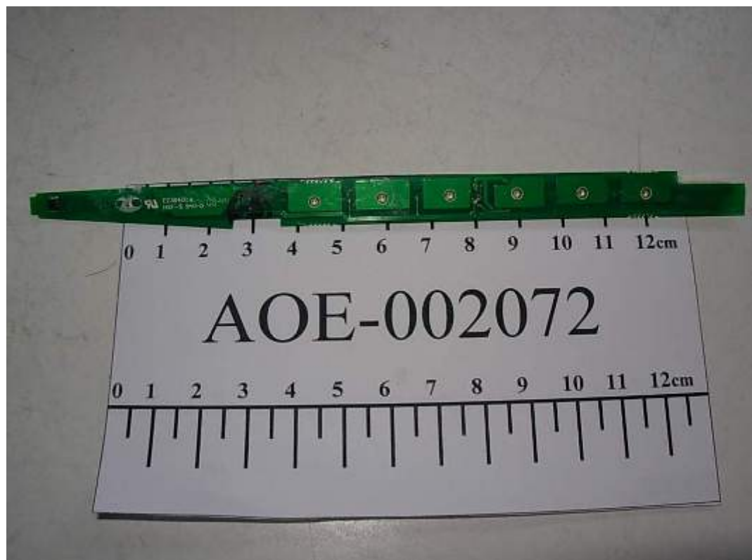
FIGURE 4 LCD MONITOR (M/N: W1954SQV) KEYBOARD (SOLDERED SIDE)
