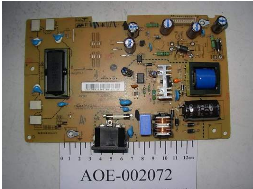
FIGURE 8 LCD MONITOR (M/N: W1954SQV) POWER BOARD (COMPONENT SIDE)
