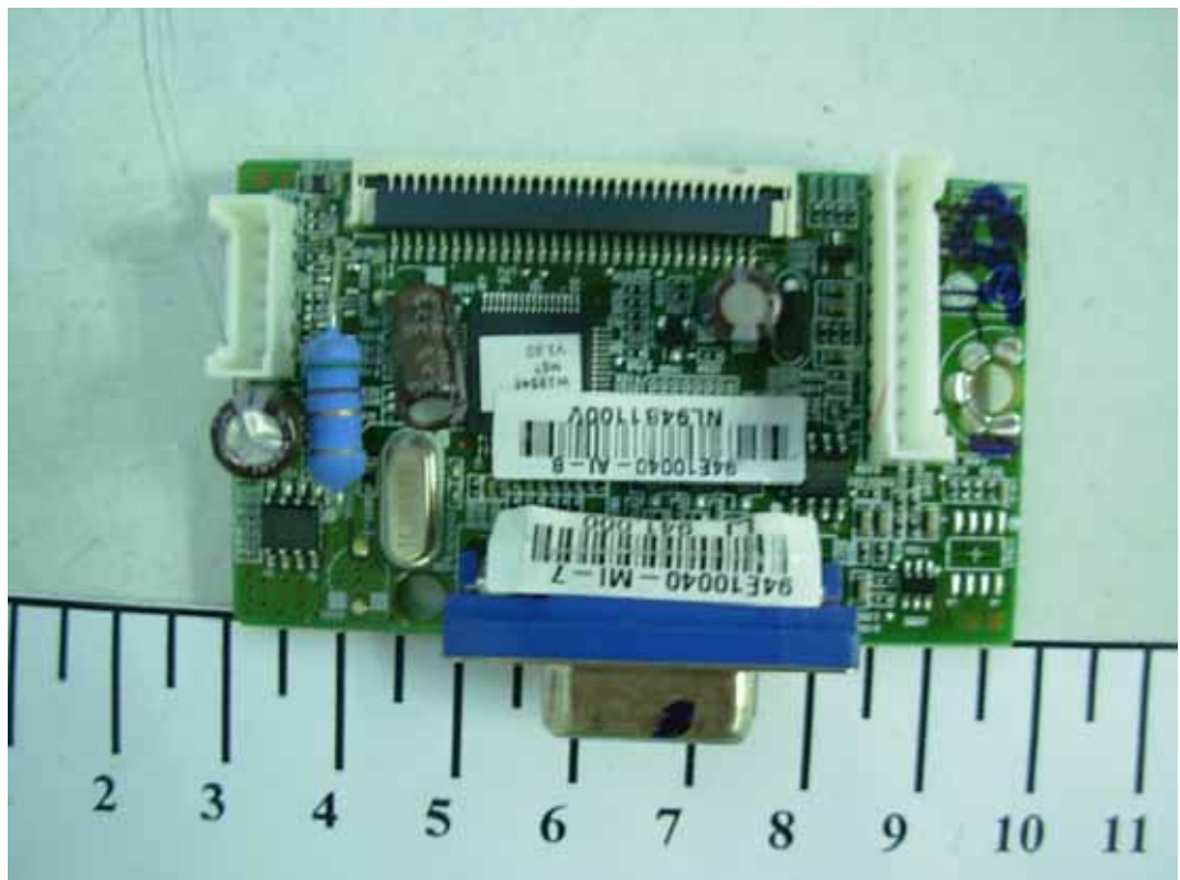
FIGURE 4 LCD MONITOR (M/N: W1954SEV) MAIN BOARD (COMPONENT SIDE)
