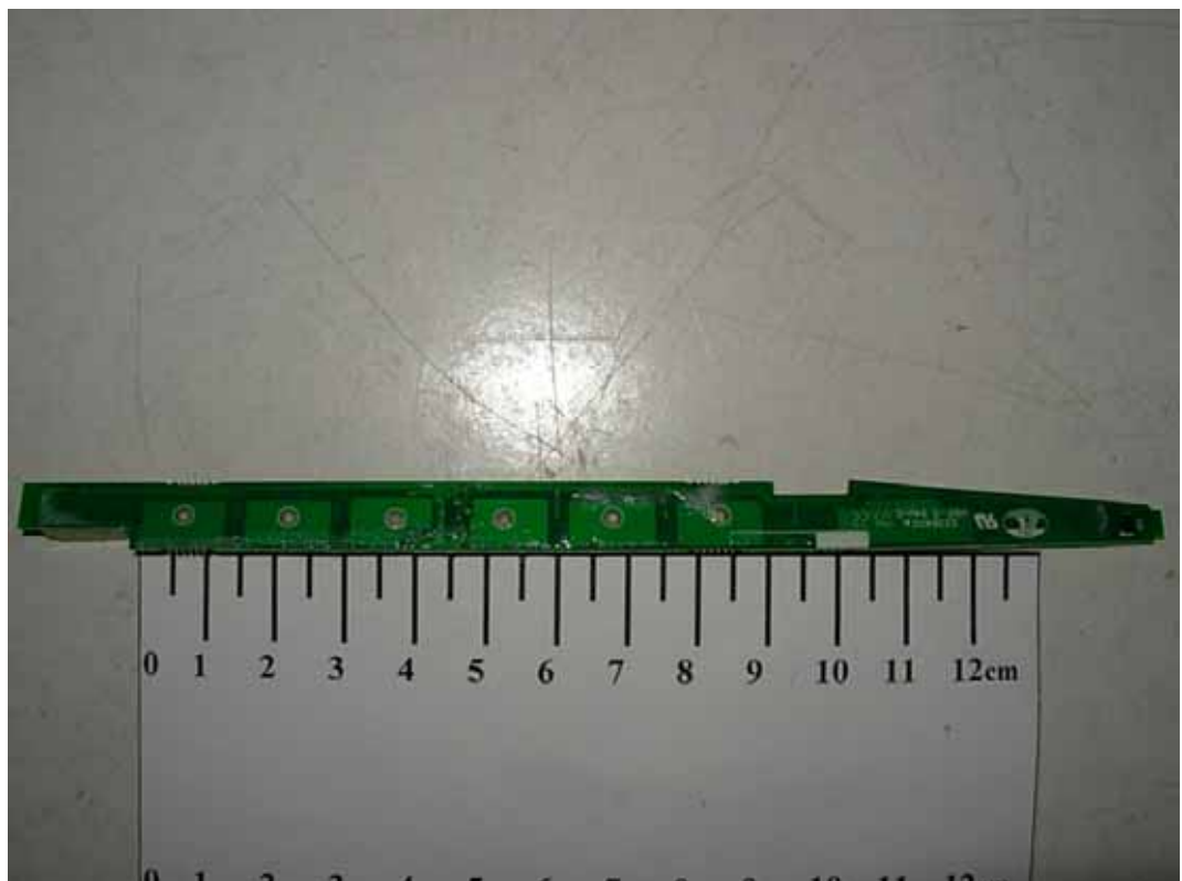
FIGURE 3 LCD MONITOR (M/N: W1954SEV) KEYBOARD (SOLDERED SIDE)
