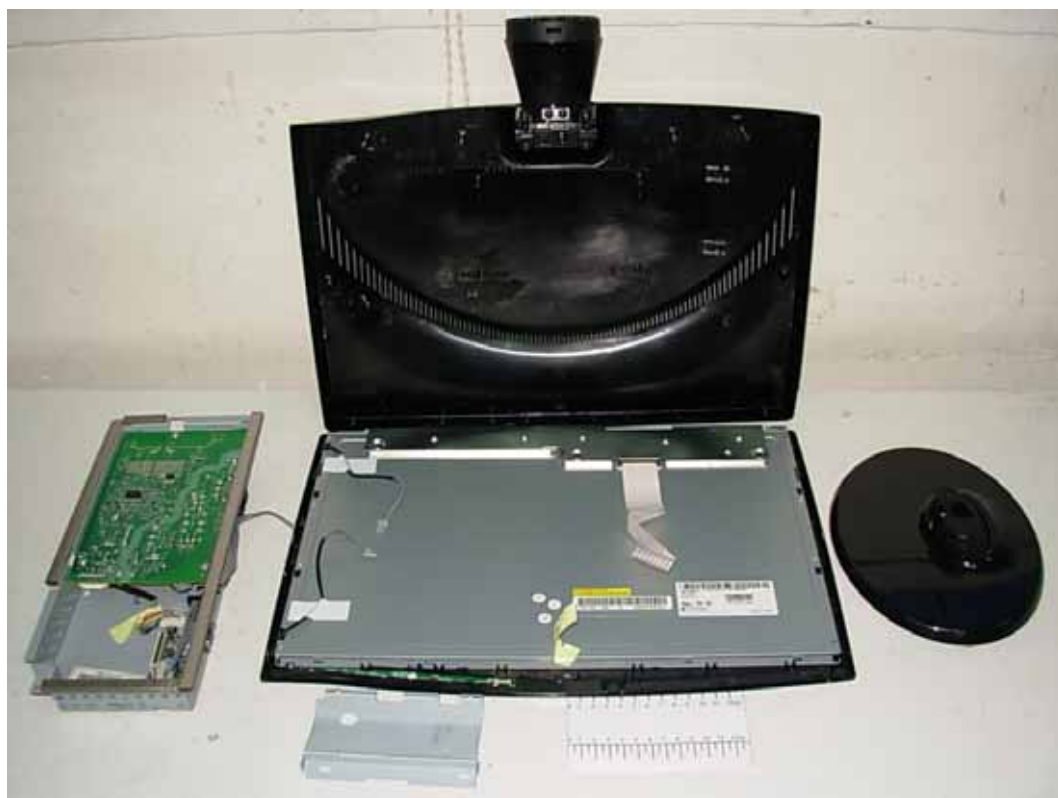
FIGURE 1 LCD MONITOR (M/N: W1954SEV) COVER REMOVED
