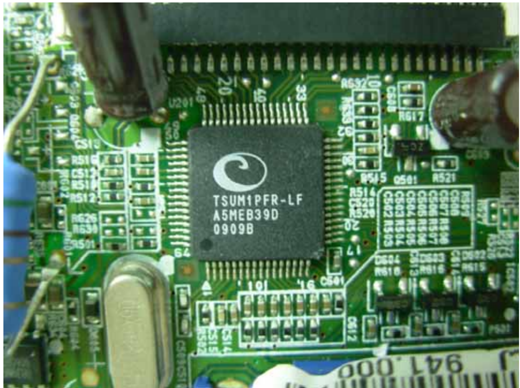
FIGURE 6 LCD MONITOR (M/N: W1954SEV) CHIP ON MAIN BOARD
