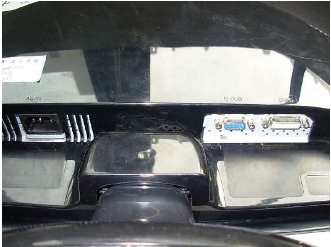
FIGURE 3 LCD MONITOR (M/N: W1953TV) PORTS VIEW
