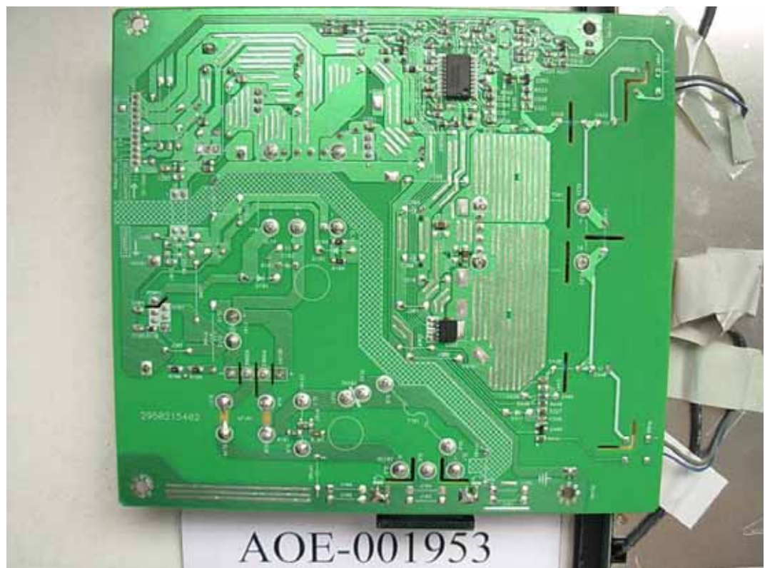
FIGURE 11 LCD MONITOR (M/N: W1952TET) POWER BOARD (SOLDERED SIDE)
