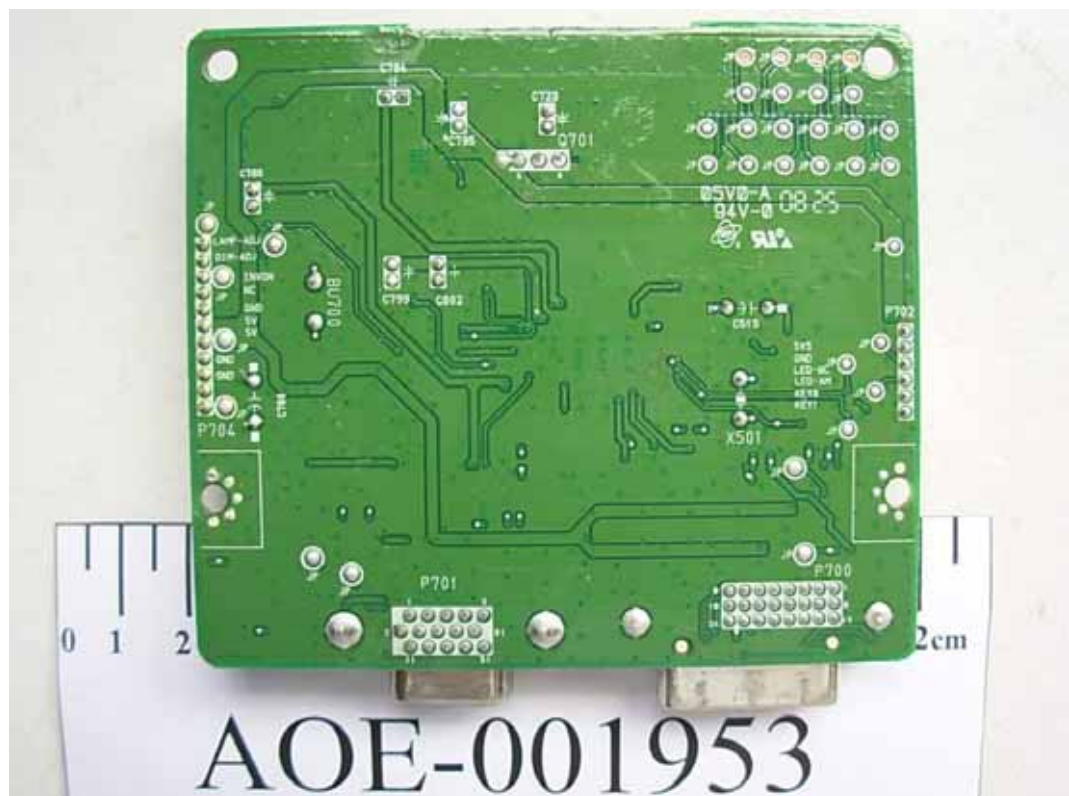
FIGURE 8 LCD MONITOR (M/N: W1952TET) MAIN BOARD (SOLDERED SIDE)
