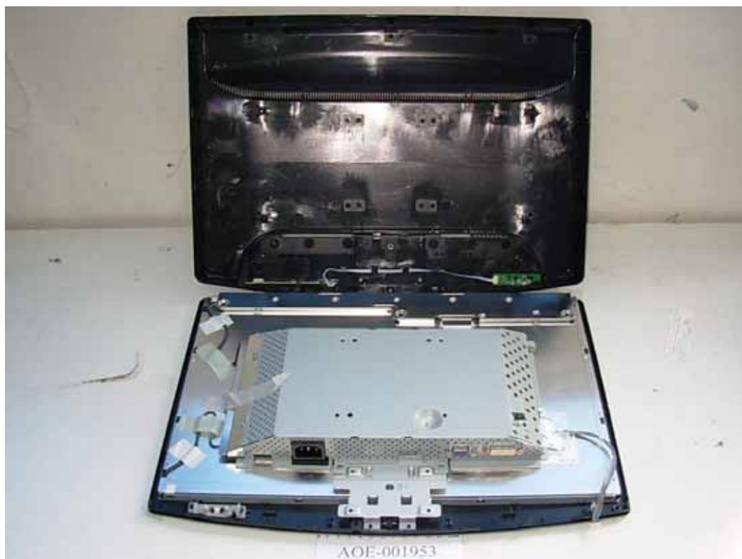
FIGURE 1 LCD MONITOR (M/N: W1952TET) COVER REMOVED
