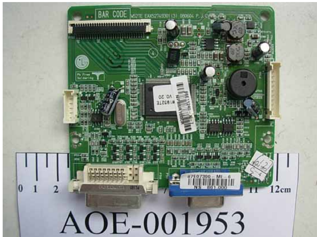
FIGURE 7 LCD MONITOR (M/N: W1952TET) MAIN BOARD (COMPONENT SIDE)
