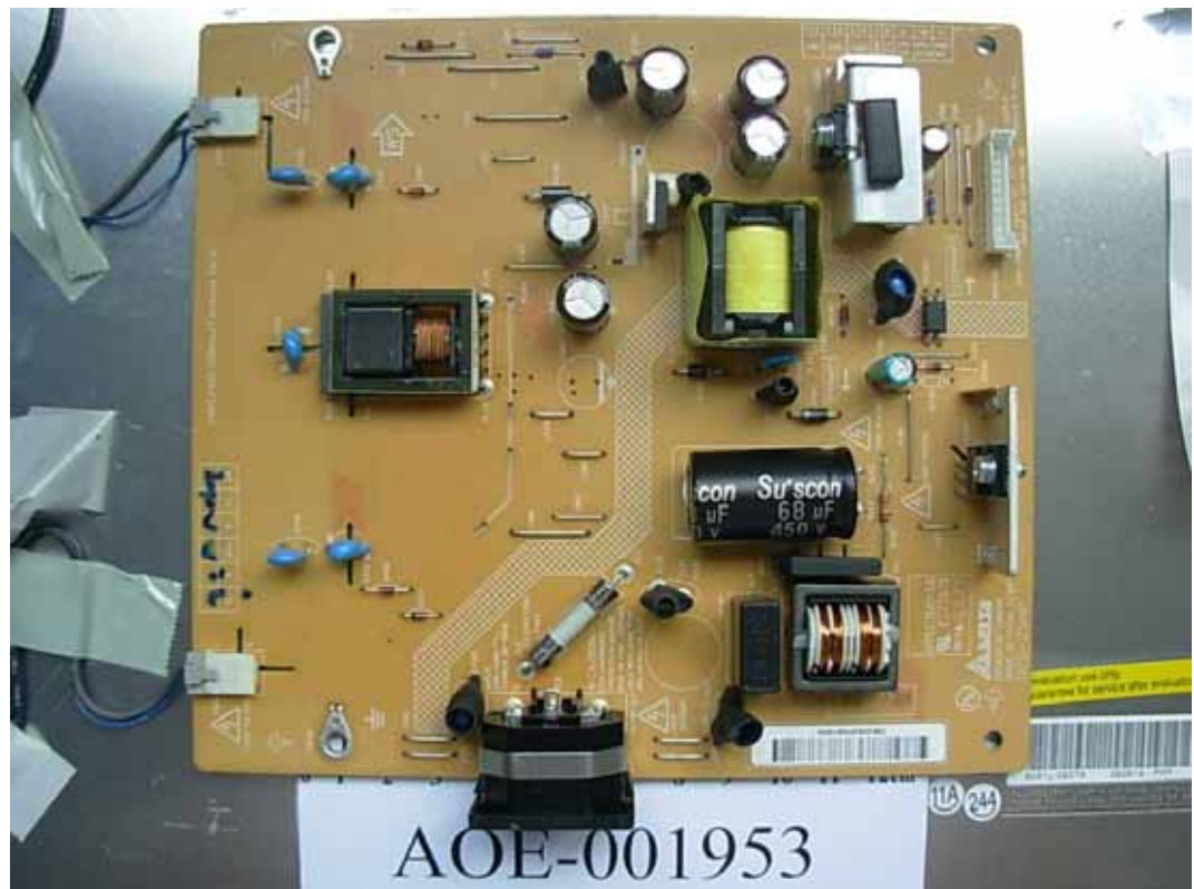
FIGURE 10 LCD MONITOR (M/N: W1952TET) POWER BOARD (COMPONENT SIDE)
