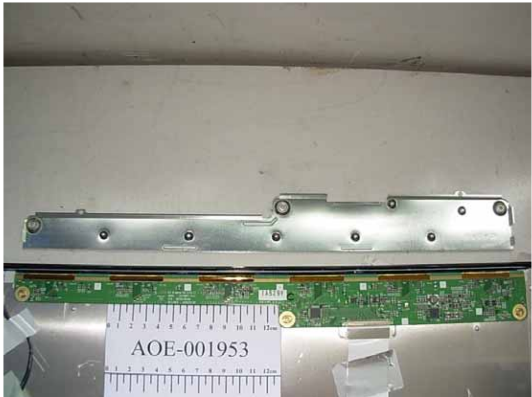
FIGURE 14 LCD MONITOR (M/N: W1952TET) LCD PANEL MAIN BOARD SHIELDED SHELL REMOVED
