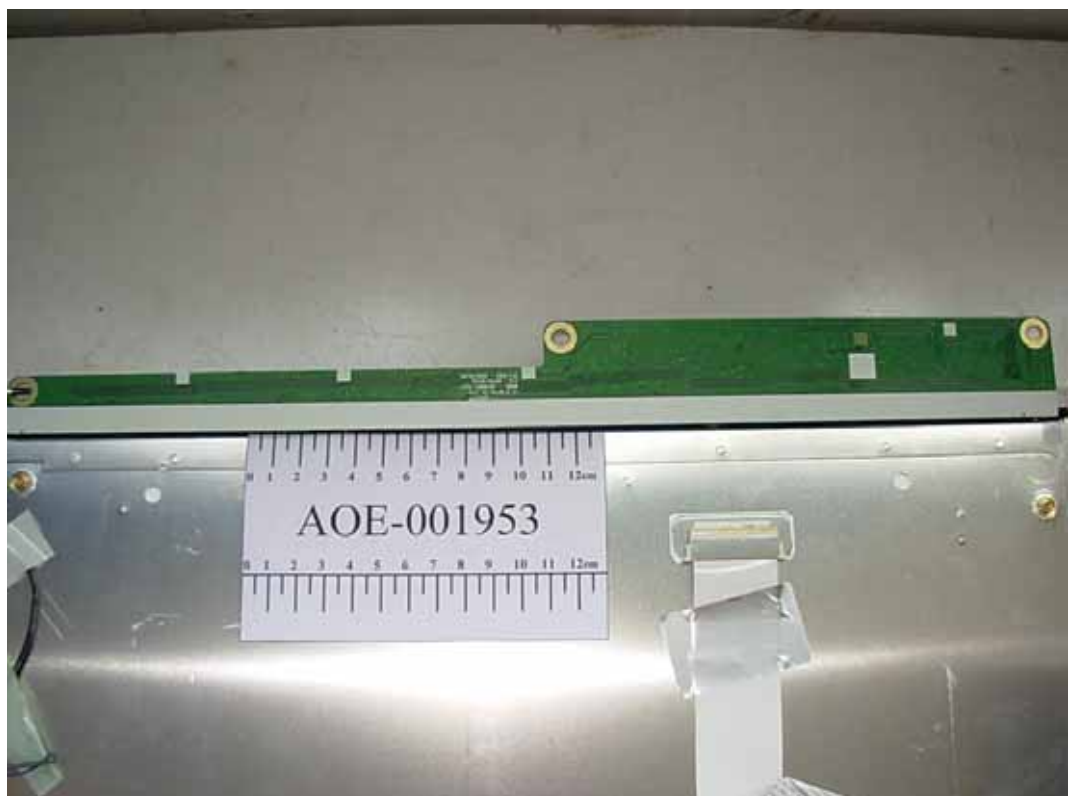
FIGURE 16 LCD MONITOR (M/N: W1952TET) LCD PANEL MAIN BOARD (SOLDERED SIDE)
