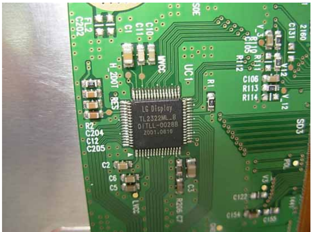
FIGURE 18 LCD MONITOR (M/N: W1952TET) LCD PANEL MAIN BOARD CHIP
