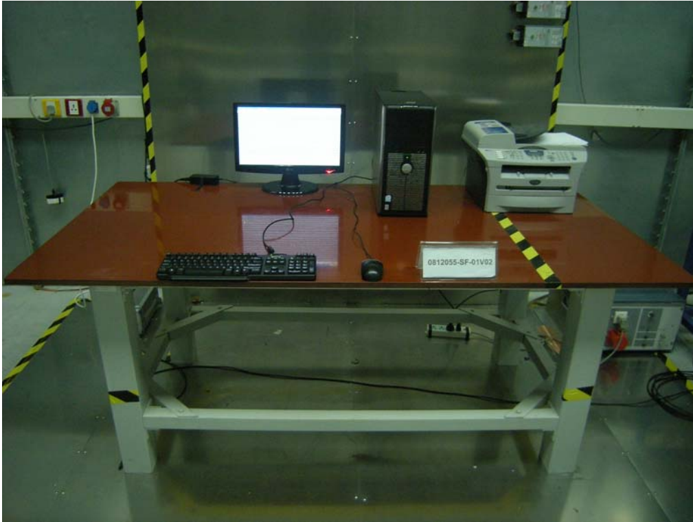
Front View of Conducted Emission Test
