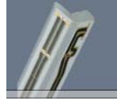
Figure 5-1 E-field Free-space Probe
