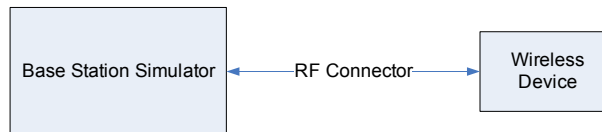
Figure 14-1 Power Measurement Setup
