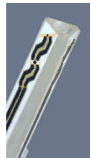
Figure 3.2 Probe Thick-Film Technique
