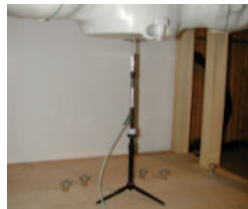
Figure 12.1 Dipole Validation Test Setup
