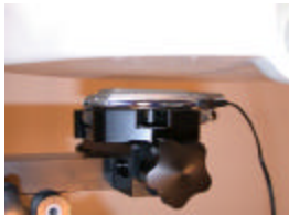
Figure 14.9 Body SAR Test Setup -- w/o Holster --
