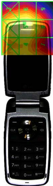
Figure 17-4 E-Field WD Scan overlay
