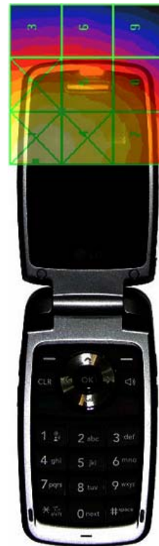
Figure 17-5 H-Field WD Scan overlay
