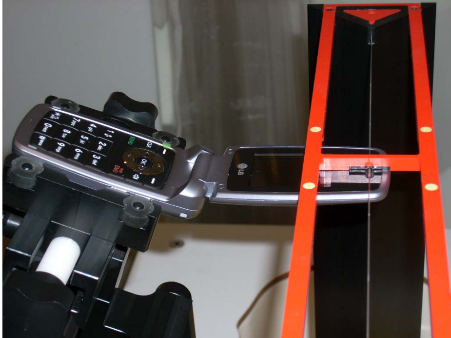
Figure 17-1 Ear Reference Point HAC Phantom Alignment
