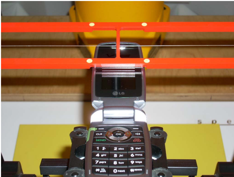
Figure 17-2 HAC Phantom Plane Alignment
