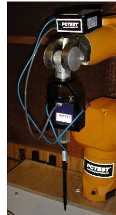
Figure 6 SPEAG Robotic System
