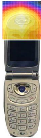
Figure 15 Sample E-field Scan Overlay
