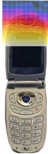
Figure 16 Sample H-field Scan Overlay
