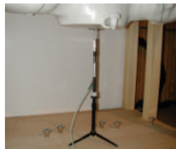
Figure 12.1 Dipole Validation Test Setup
