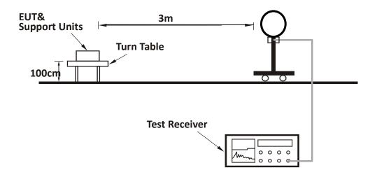
For Radiated emission 30MHz to 1GHz:
