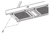
**4** To remove, slide the grease filter forward slightly and pull it downward.
