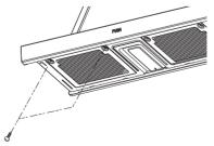
**4** To remove, slide the grease filter forward slightly and pull it downward.
