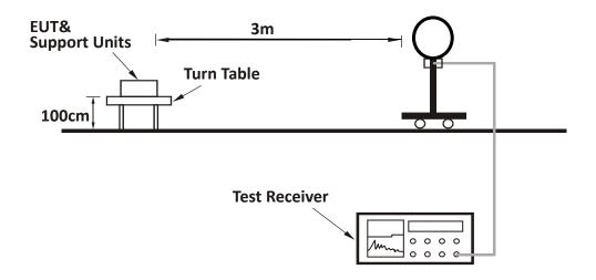
For Radiated emission 30MHz to 1GHz:
