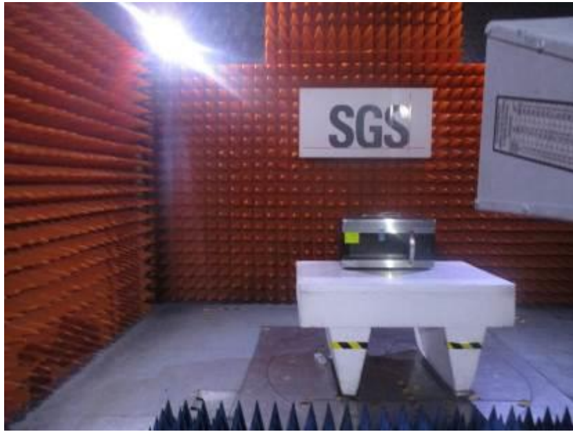
Radiated Emissions (above 1GHz) Test Setup
