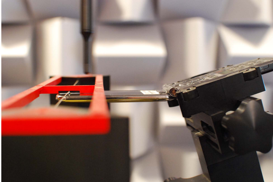
Figure 17-1 Ear Reference Point HAC Phantom Alignment
