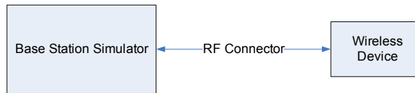
Figure 15-1 Power Measurement Setup
