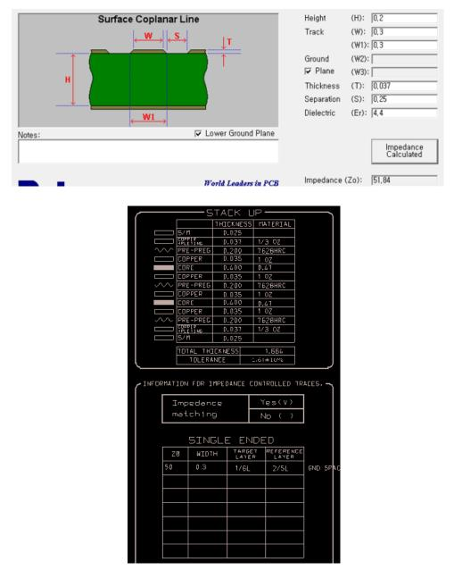
Note1. Measurement results delivered with boards. Controlled impedence shall be 50 Ohms +/-15% on layer TOP 0.3mm microstrip traces referenced to layer 2 plane and with a copper clearance of 0.25mm.
