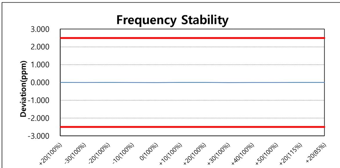
**Note.** Based on the results of the frequency stability test at the center channel the frequency deviation results measured are very small. As such it is determined that the channels at the band edge would remain in band when the maximum measured frequency deviation noted during the frequency stability tests is applied. Therefore the device is determined to remain operating in band over the temperature and voltage range as tested.
