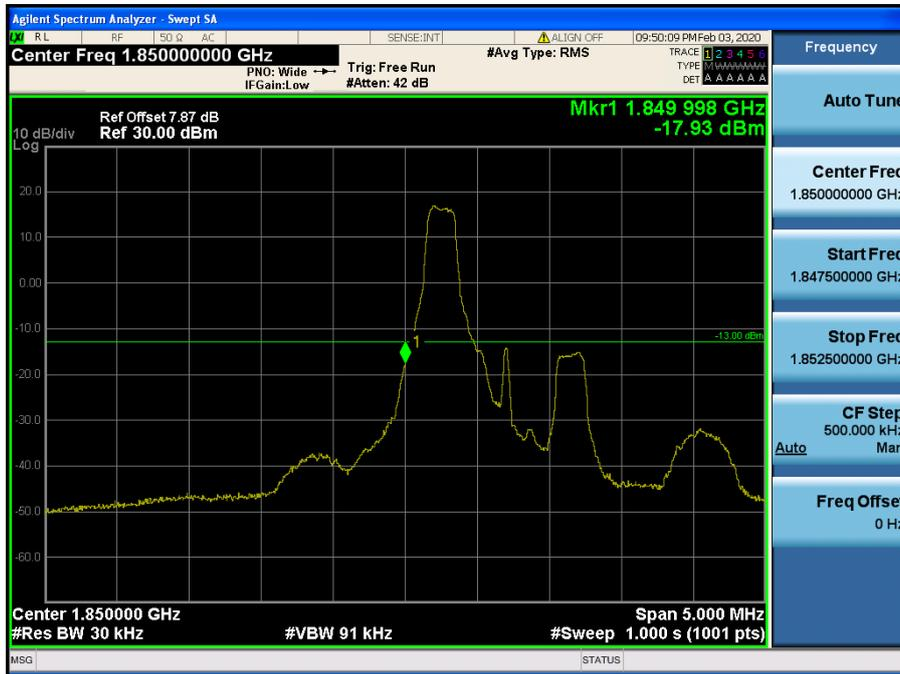
LTE Band 2 / 1.4MHz / 16QAM - RB Size/Offset (1/0)
