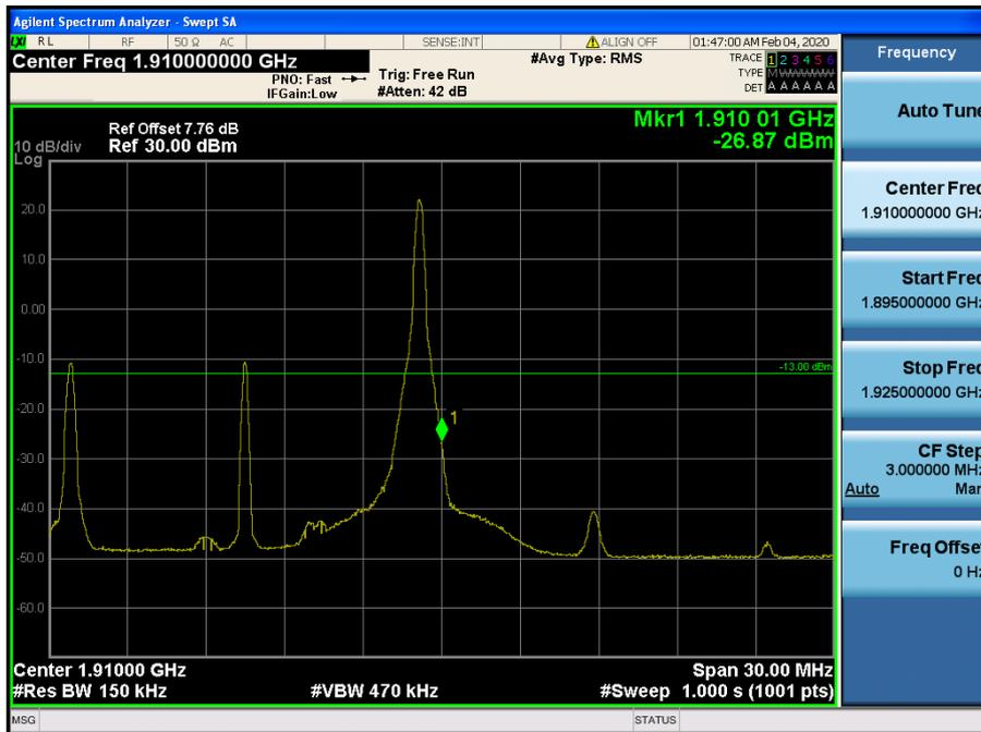
LTE Band 2 / 15MHz / 16QAM - RB Size/Offset (1/74)
