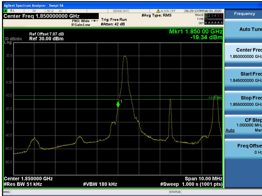
LTE Band 2 / 5MHz / QPSK - RB Size/Offset (1/0)
