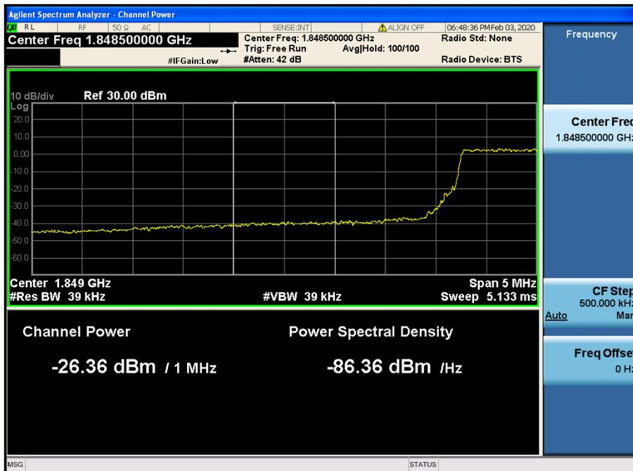
LTE Band 2 / 5MHz / QPSK - RB Size/Offset (25/0)
