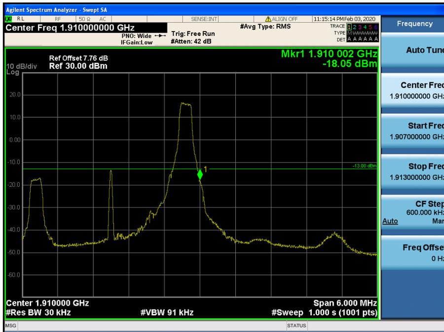
LTE Band 2 / 3MHz / 16QAM - RB Size/Offset (1/14)
