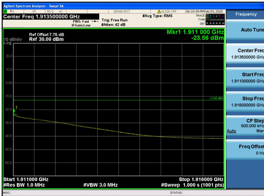
LTE Band 2 / 3MHz / QPSK - RB Size/Offset (8/4)
