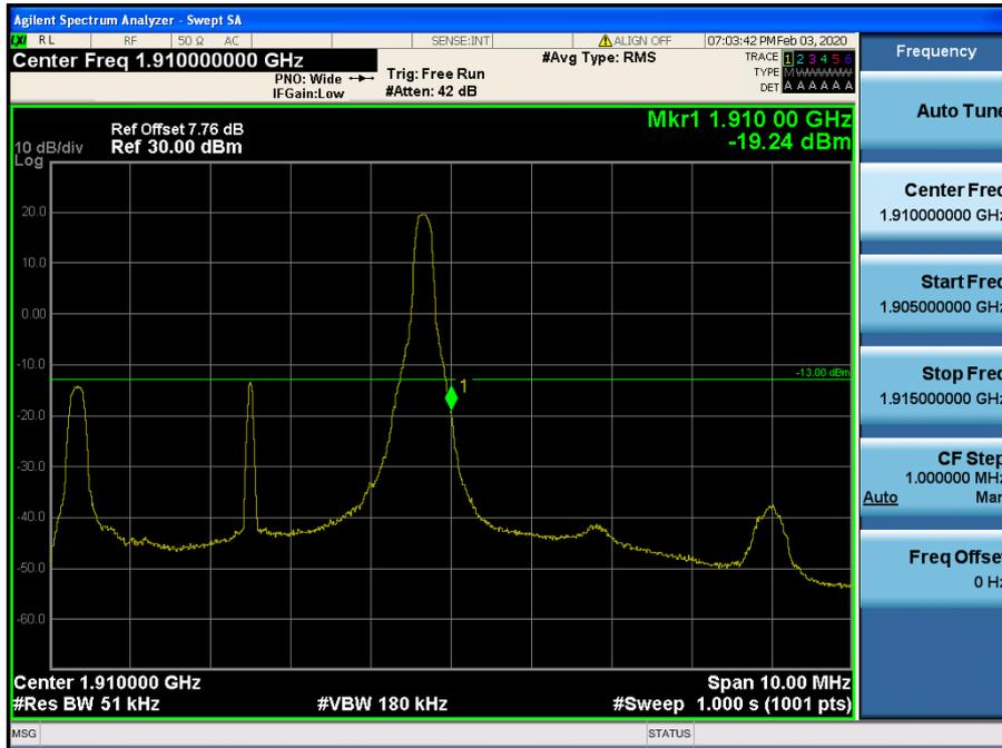
LTE Band 2 / 5MHz / QPSK - RB Size/Offset (1/24)
