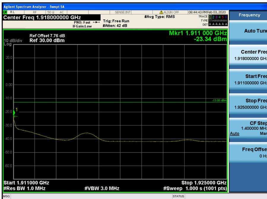
LTE Band 2 / 15MHz / QPSK - RB Size/Offset (1/74)
