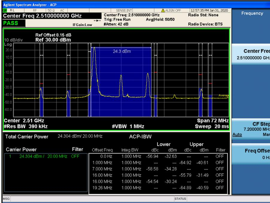
LTE Band 7 / 20MHz / QPSK - RB Size/Offset (1/0)
