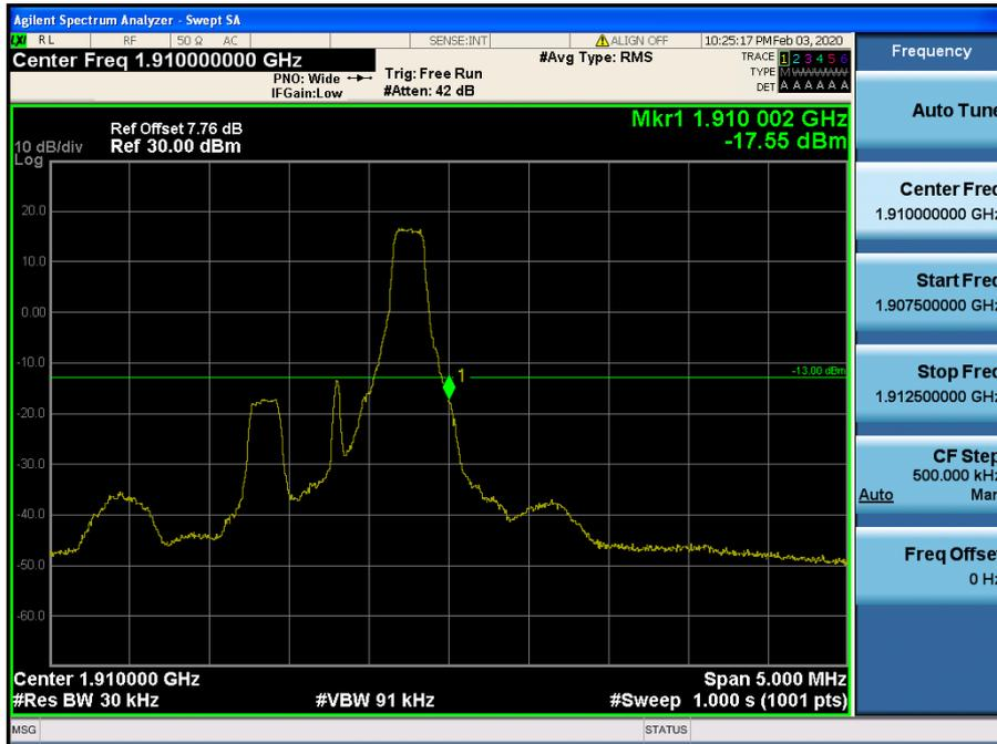
LTE Band 2 / 1.4MHz / 16QAM - RB Size/Offset (1/5)
