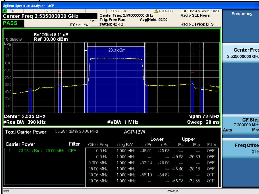
LTE Band 7 / 20MHz / QPSK- RB Size/Offset (100/0)
