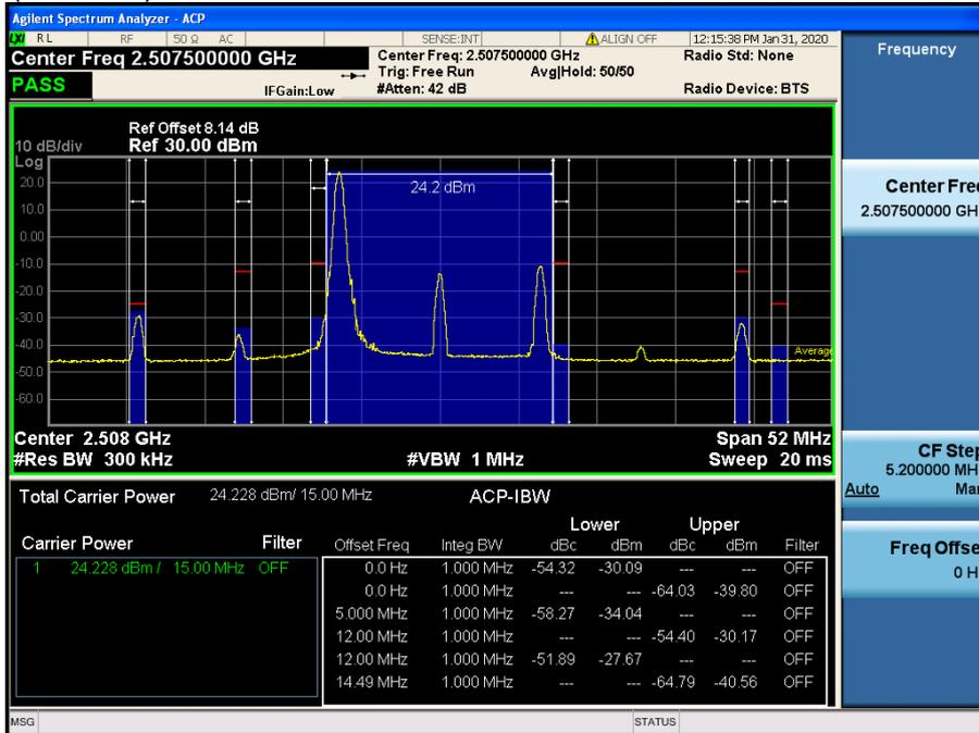
LTE Band 7 / 15MHz / QPSK - RB Size/Offset (1/0)
