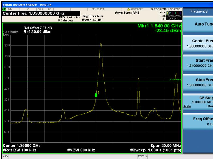
LTE Band 2 / 10MHz / QPSK - RB Size/Offset (1/0)
