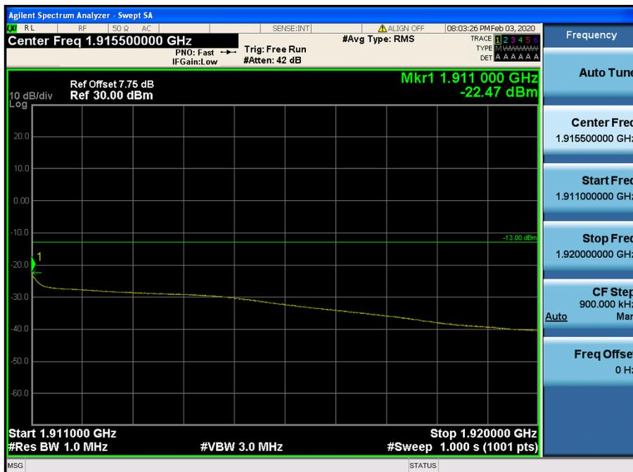
LTE Band 2 / 10MHz / QPSK - RB Size/Offset (25/25)
