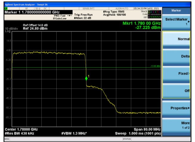
DFT-S-OFDM 16QAM - High Channel - Full RB
