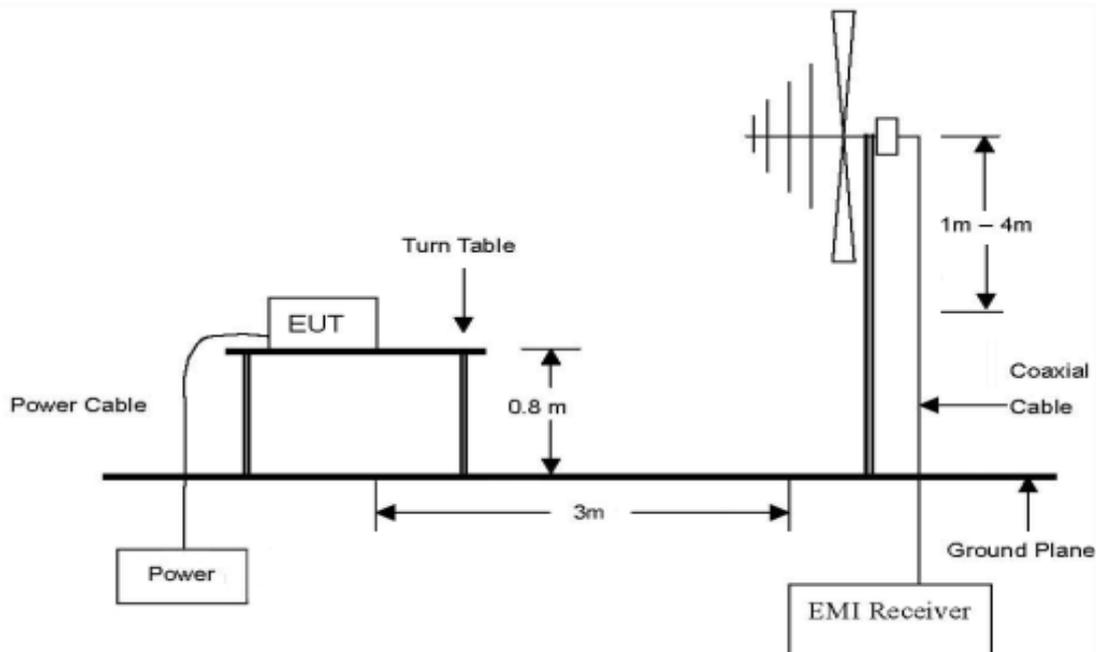
The diagram below shows the test setup that is utilized to make the measurements for emission. The spurious emissions were investigated from 1 GHz to the 10th harmonic of the highest fundamental frequency or 40 GHz, whichever is lower.
