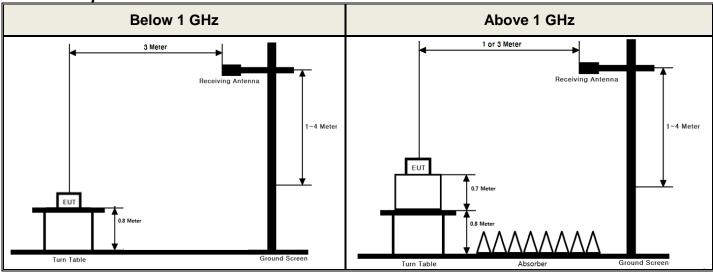
These measurements were performed at 3 m test site. The equipment under test is placed on a non-conductive table 0.8 meter or 1.5 meters above a turntable which is flush with the ground plane and 3 meters from the receive antenna. For measurements above 1 GHz absorbers are placed on the floor between the turn table and the antenna mast in such a way so as to maximize the reduction of reflections. For measurements below 1 GHz, the absorbers are removed.
