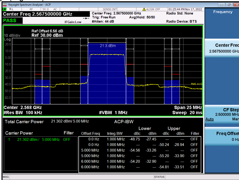
LTE Band 7 / 5 MHz / QPSK - RB Size/Offset (25/0)
