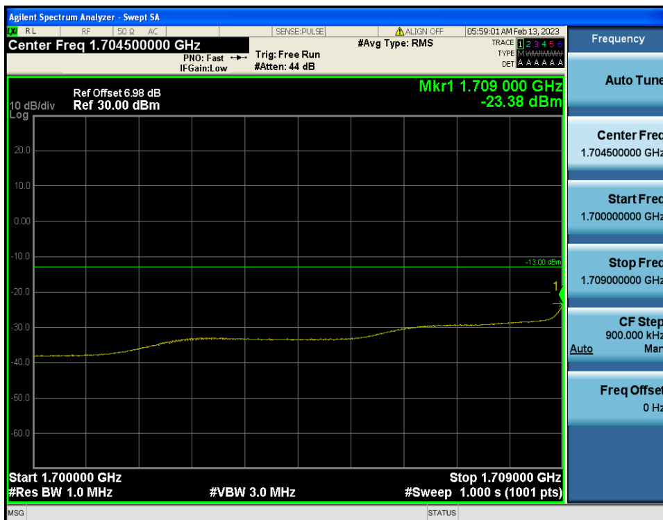
LTE Band 4 / 10MHz / QPSK - RB Size/Offset (25/0)
