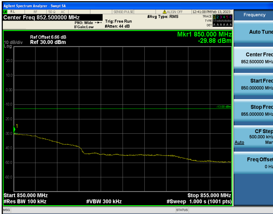
LTE Band 5 / 3MHz / QPSK - RB Size/Offset (15/0)
