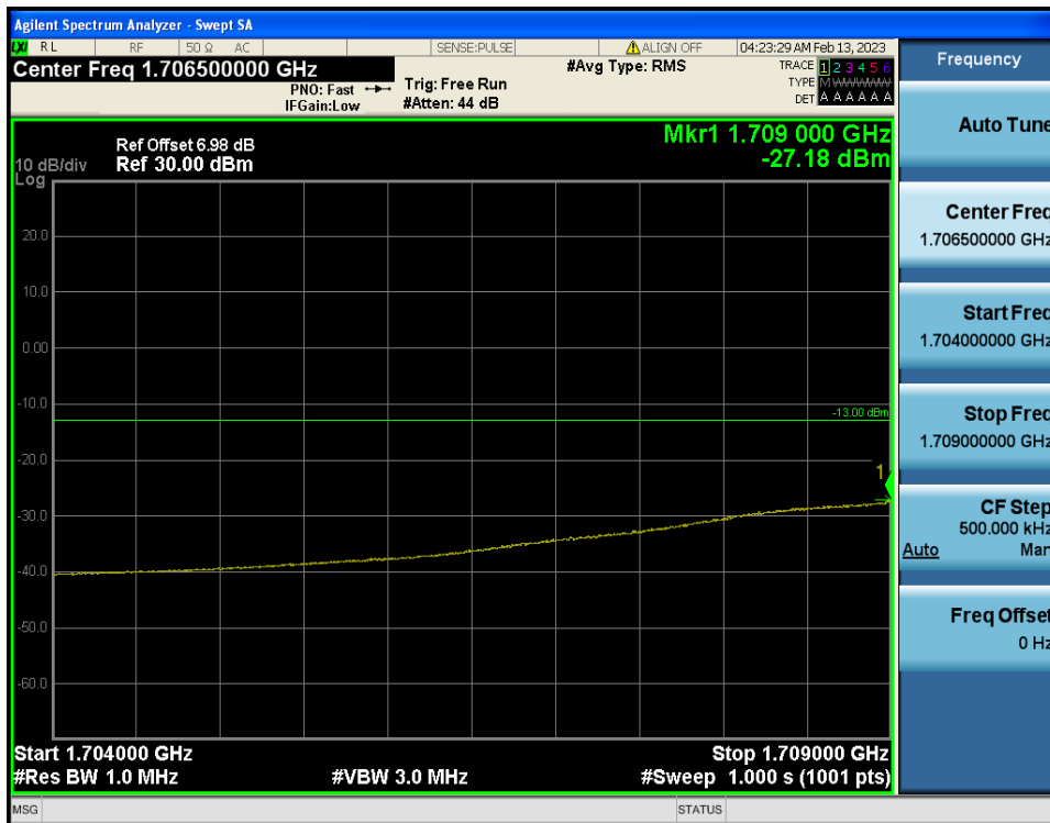
LTE Band 4 / 3MHz / QPSK - RB Size/Offset (8/4)
