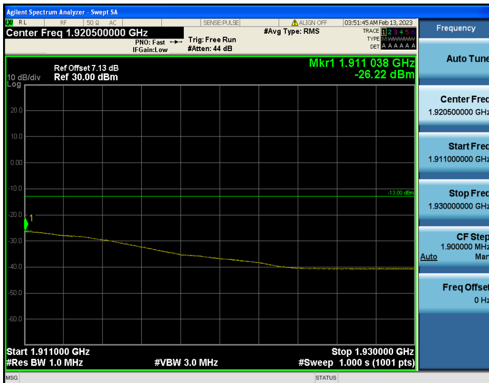
LTE Band 2 / 20MHz / 16QAM - RB Size/Offset (50/50)
