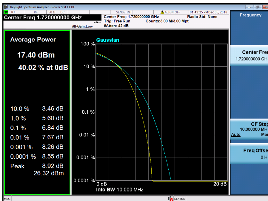
LTE Band 4 / 20 MHz / 16QAM - RB Size 100
