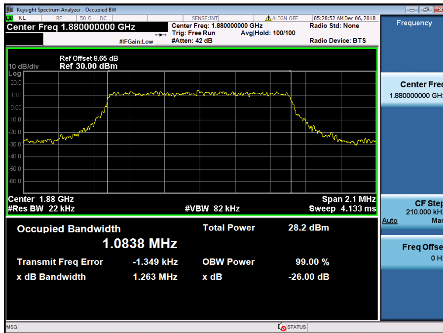
LTE Band 2 / 1.4 MHz / QPSK - RB Size 6
