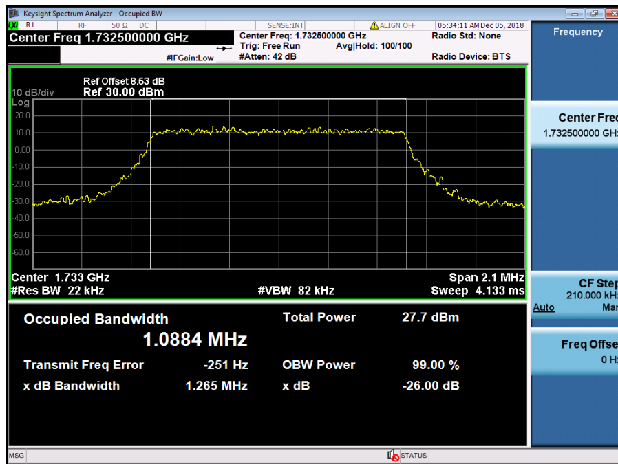
LTE Band 4 / 1.4 MHz / QPSK - RB Size 6
