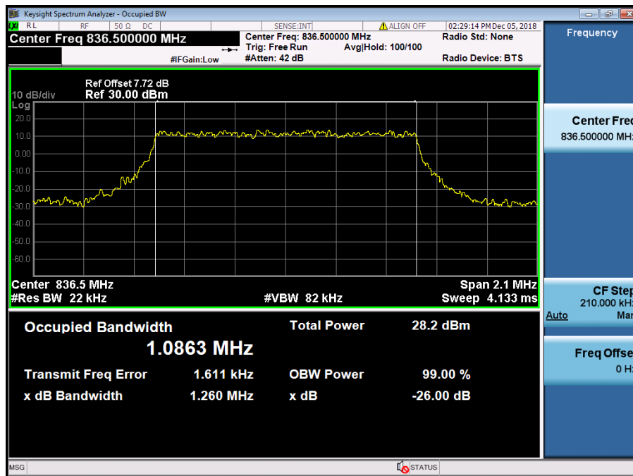
LTE Band 5 / 1.4 MHz / QPSK - RB Size 6
