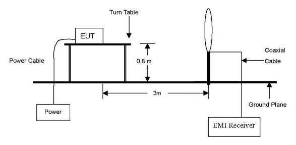
The diagram below shows the test setup that is utilized to make the measurements for emission from 30  $\,\mathrm{Mb}$  to 1  $\,\mathrm{GHz}$ .
