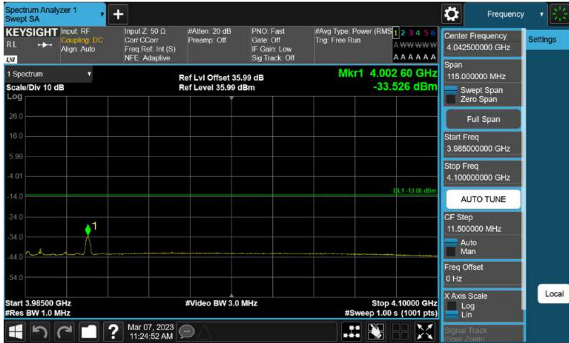
Sub6 n77(78). High Band Edge Plot (50 M BW Ch.663666 BPSK 1RB)(3)
