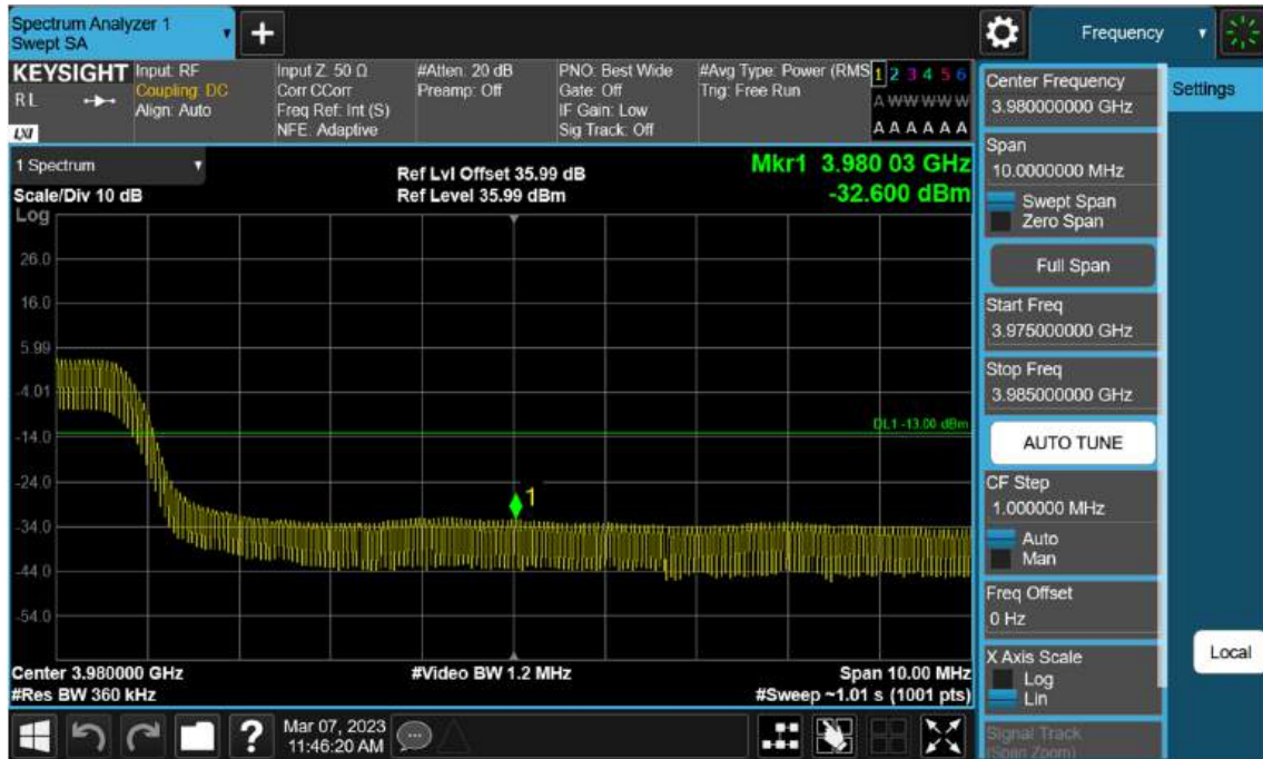
Sub6 n77(78). High Band Edge Plot (70 M BW Ch.663000 BPSK FullRB)(1)
