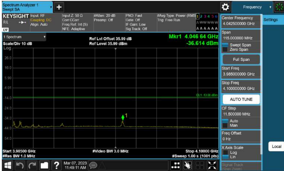
Sub6 n77(78). High Band Edge Plot (70 M BW Ch.663000 BPSK 1RB)(3)
