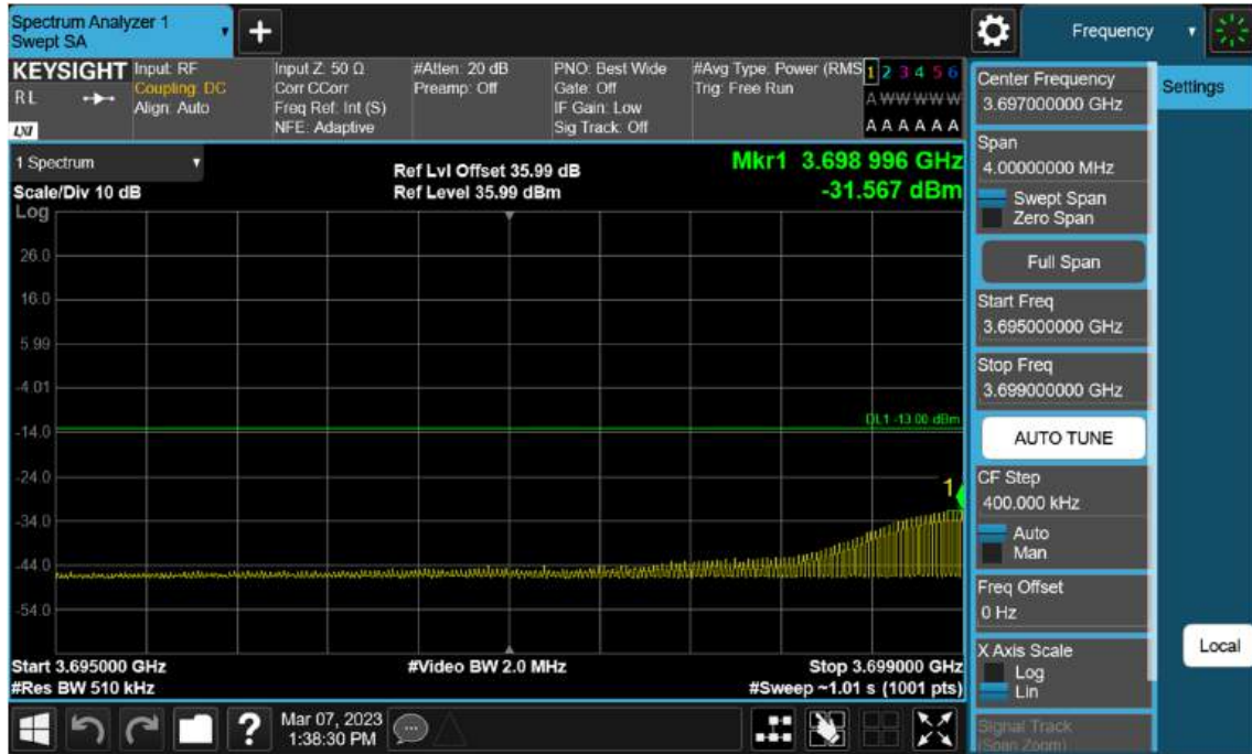
Sub6 n77(78). Low Band Edge Plot (90 M BW Ch.649668 BPSK 1RB)(2)
