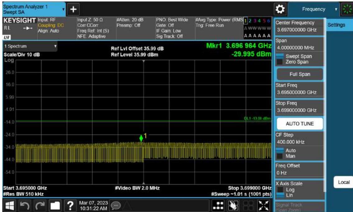
Sub6 n77(78). Low Band Edge Plot (40 M BW Ch.648000 BPSK FullRB)(2)
