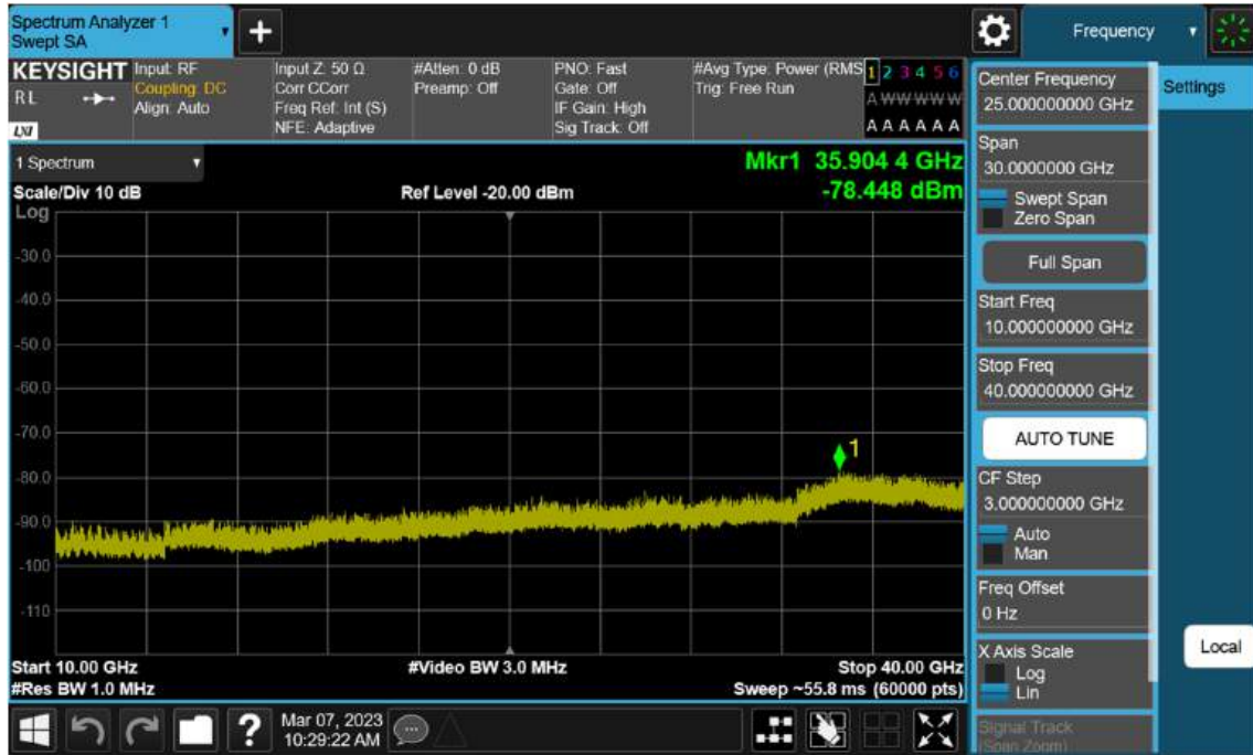
Sub6 n77(78). Conducted Spurious Plot_2 (664332ch_30 MHz_BPSK)
