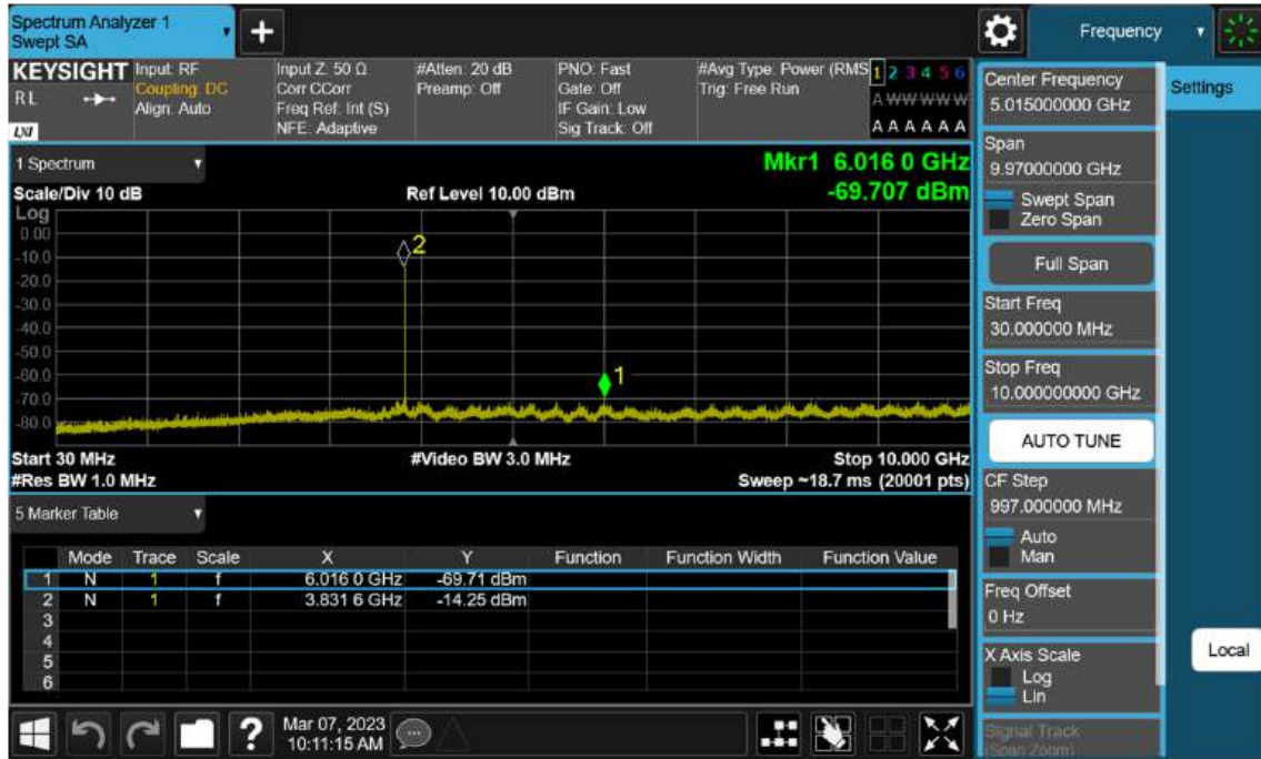
Sub6 n77(78). Conducted Spurious Plot_1 (656000ch_20 MHz_BPSK)
