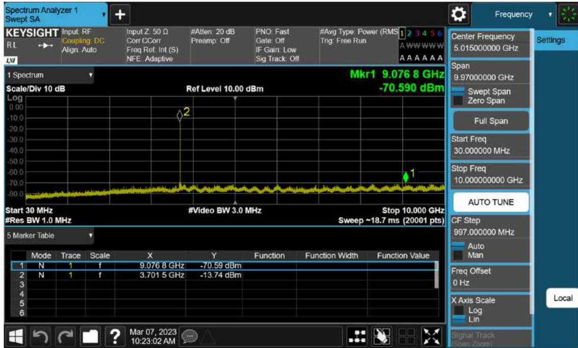
Sub6 n77(78). Conducted Spurious Plot_1 (647668ch_30 MHz_BPSK)
