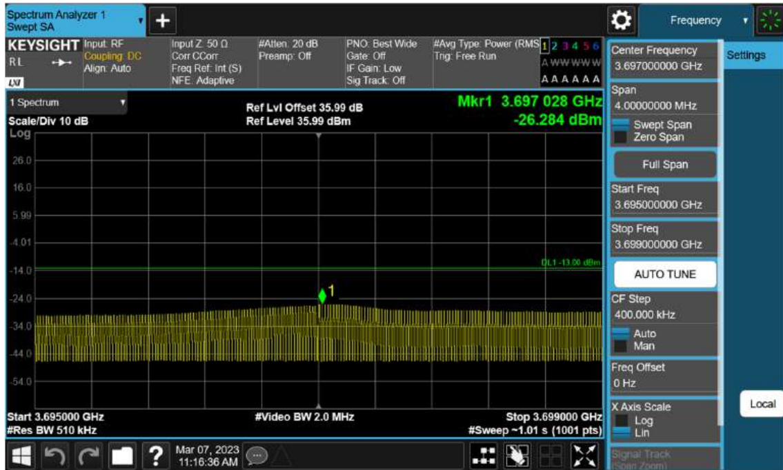
Sub6 n77(78). Low Band Edge Plot (50 M BW Ch.648334 BPSK FullRB)(2)
