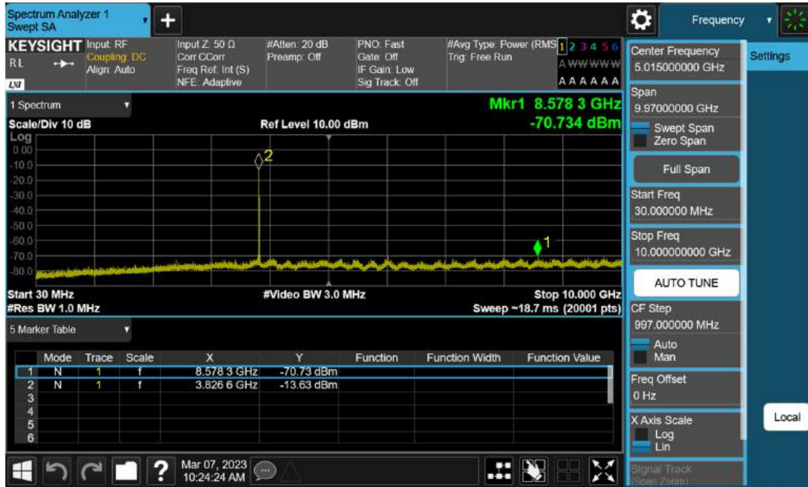
Sub6 n77(78). Conducted Spurious Plot_1 (656000ch_30 MHz_BPSK)
