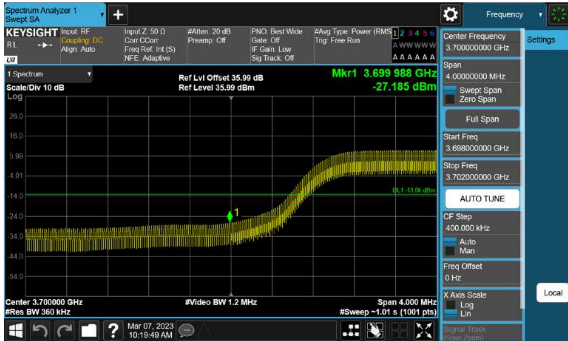
Sub6 n77(78). Low Band Edge Plot (30 M BW Ch.647668 BPSK FullRB)(1)
