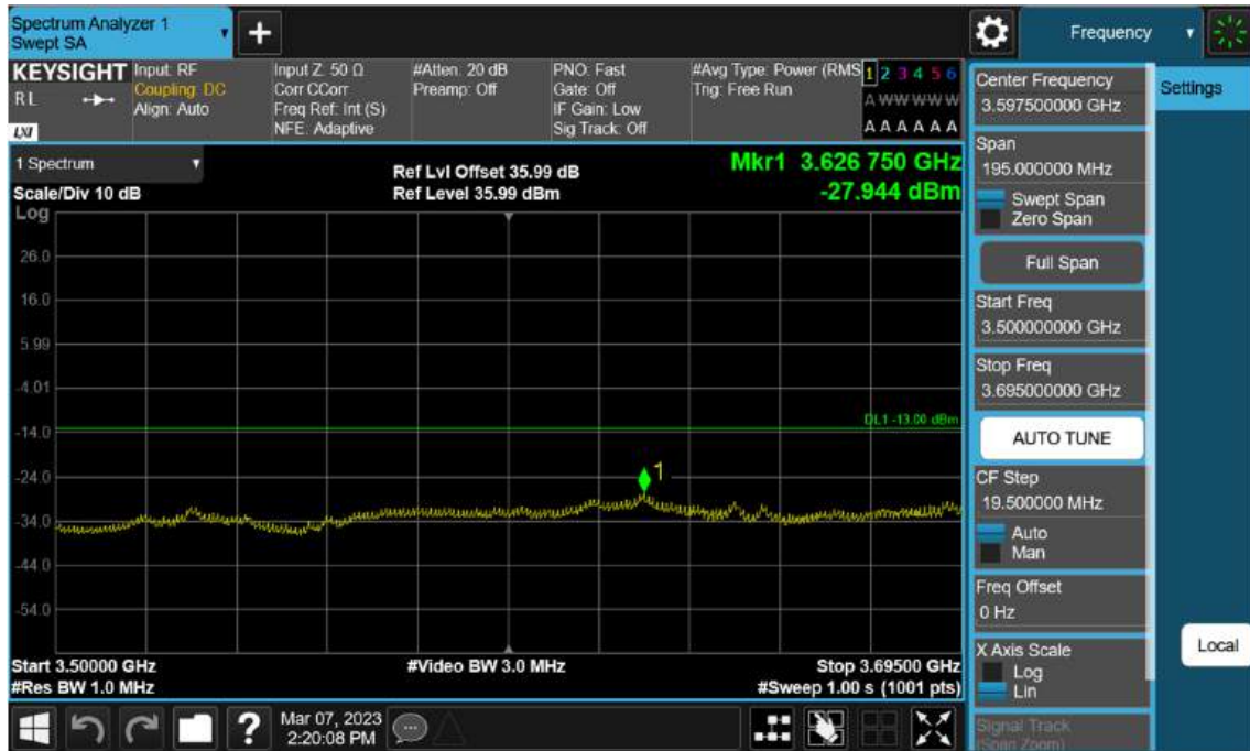
Sub6 n77(78). Low Band Edge Plot (100 M BW Ch.650000 BPSK FullRB)(3)
