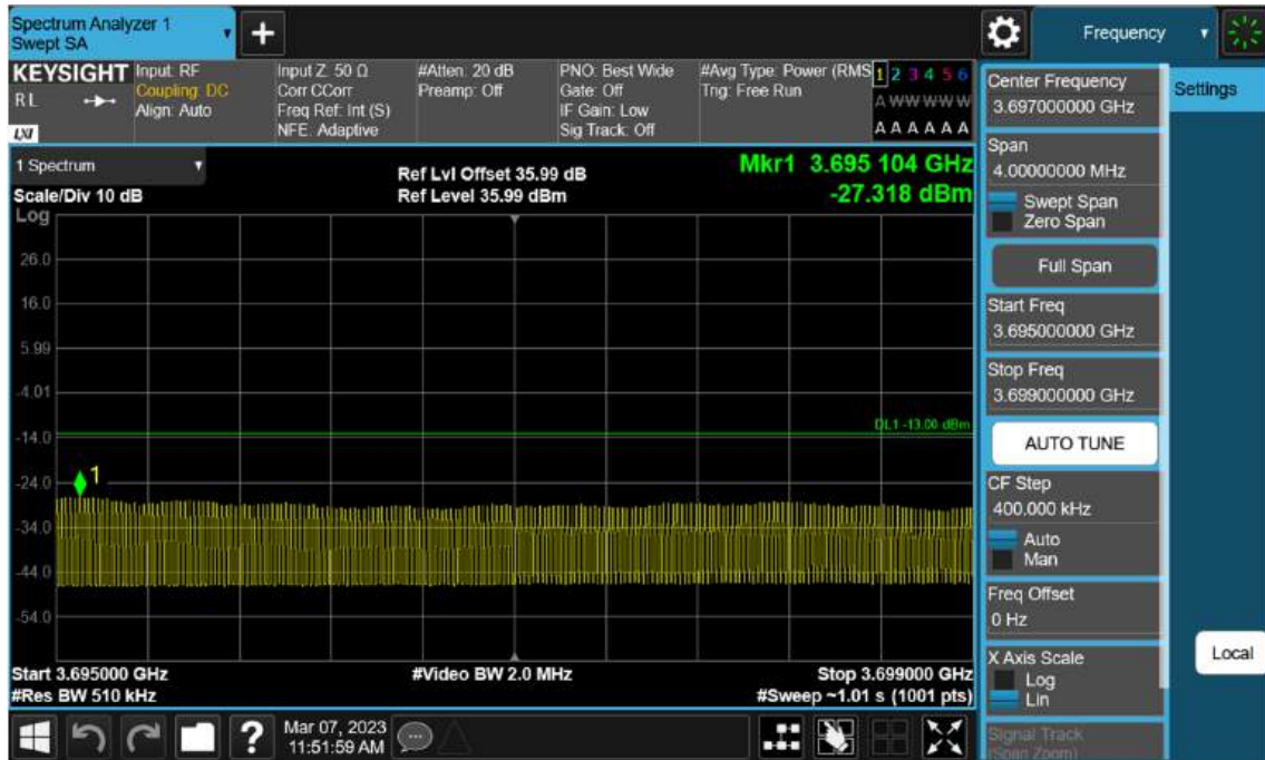
Sub6 n77(78). Low Band Edge Plot (80 M BW Ch.649334 BPSK FullRB)(2)
