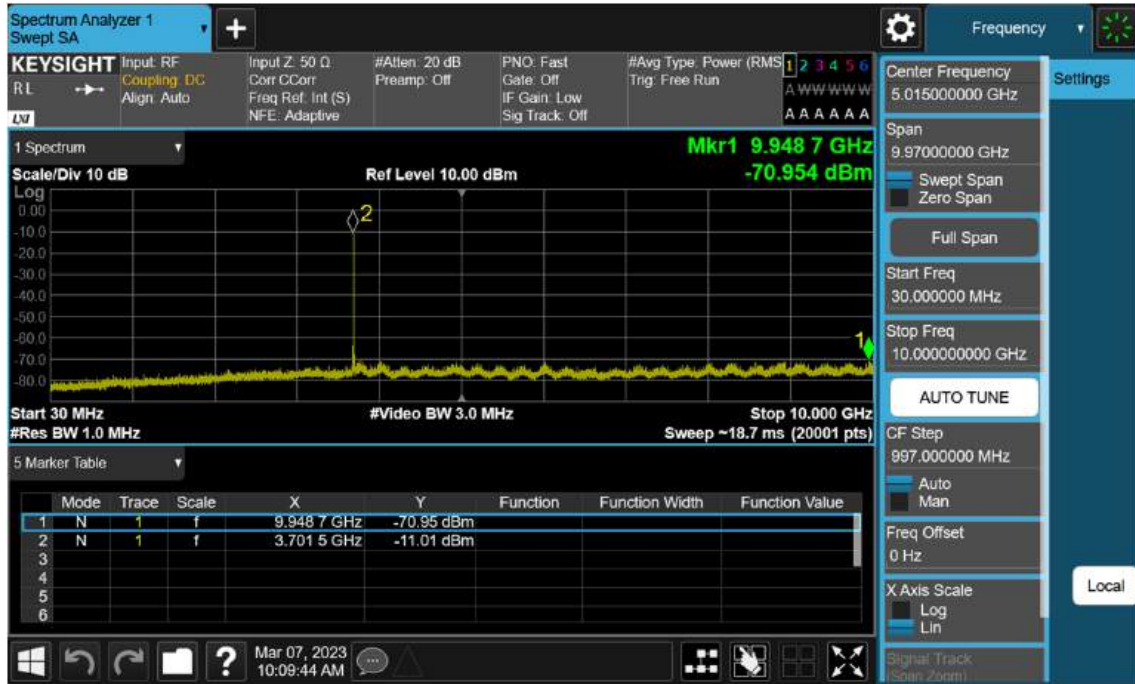
Sub6 n77(78). Conducted Spurious Plot_1 (647334ch_20 MHz_BPSK)
