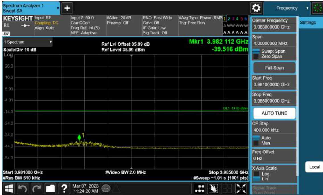
Sub6 n77(78). High Band Edge Plot (50 M BW Ch.663666 BPSK 1RB)(2)
