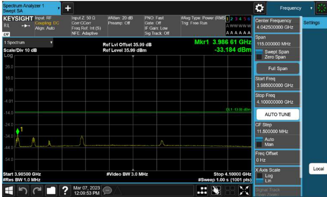
Sub6 n77(78). High Band Edge Plot (80 M BW Ch.662666 BPSK 1RB)(3)
