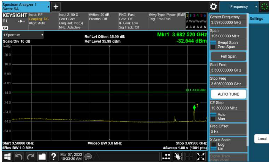
Sub6 n77(78). Low Band Edge Plot (40 M BW Ch.648000 BPSK 1RB)(3)
