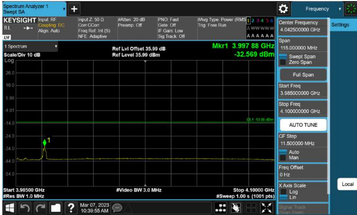
Sub6 n77(78). High Band Edge Plot (40 M BW Ch.664000 BPSK 1RB)(3)
