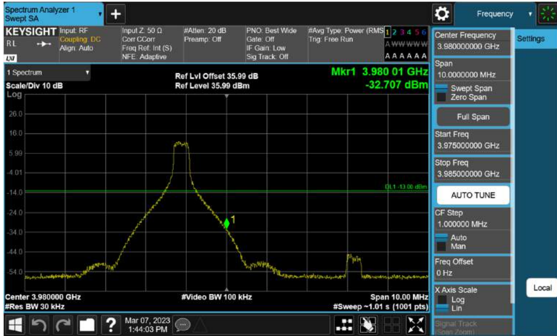
Sub6 n77(78). High Band Edge Plot (90 M BW Ch.662332 BPSK 1RB)(1)
