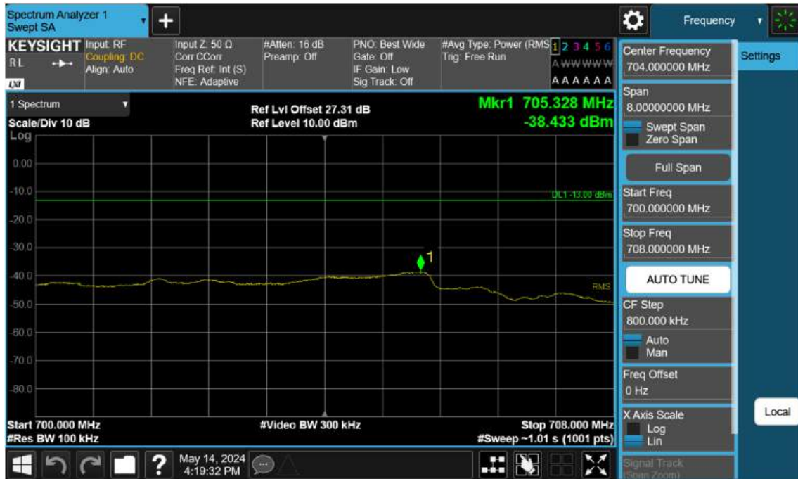
Sub6 n71. Upper Extended Band Edge Plot (20 M BW Ch.137600 BPSK_ Full RB)
