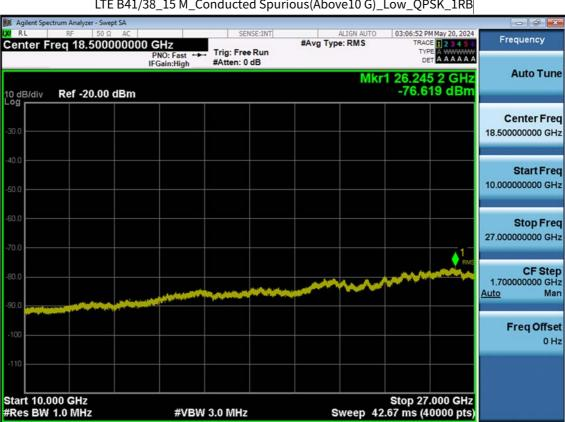
LTE B41/38\_15 M\_Conducted Spurious(Above10 G)\_Low\_QPSK\_1RB
