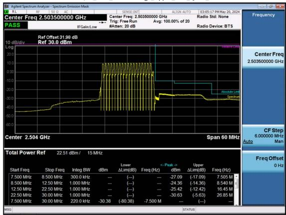
LTE B41/38\_15 M\_Channel Edge\_Upper\_Low\_QPSK\_FullRB
