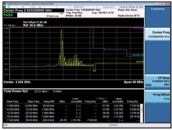
LTE B41/38\_15 M\_Channel Edge\_Upper\_Low\_QPSK\_1RB
