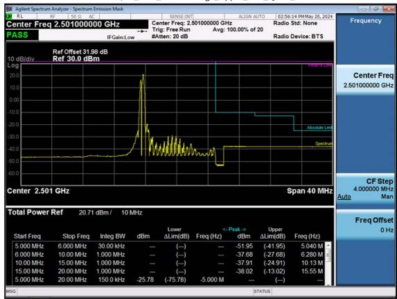
LTE B41/38\_10 M\_Channel Edge\_Upper\_Low\_QPSK\_1RB
