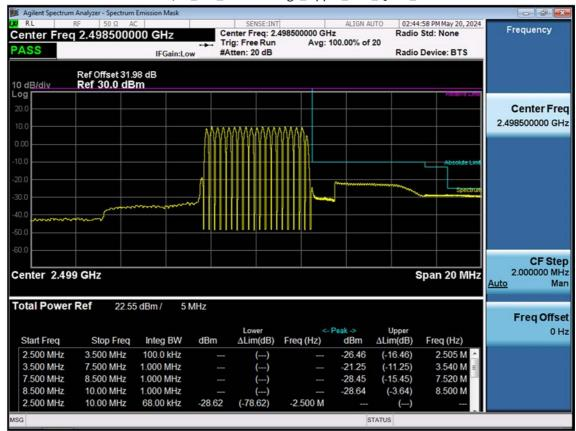
LTE B41/38\_5 M\_Channel Edge\_Upper\_Low\_QPSK\_FullRB
