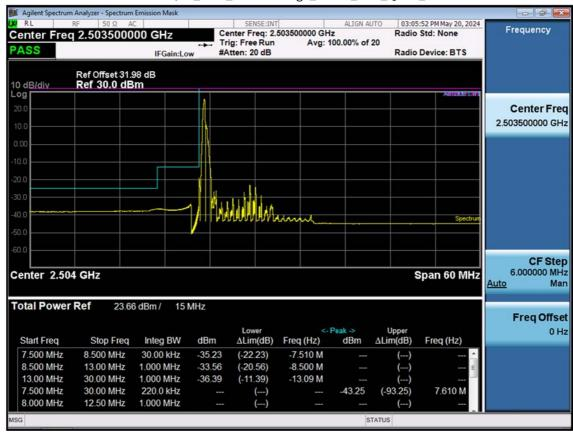
LTE B41/38\_15 M\_Channel Edge\_Lower\_Low\_QPSK\_1RB
