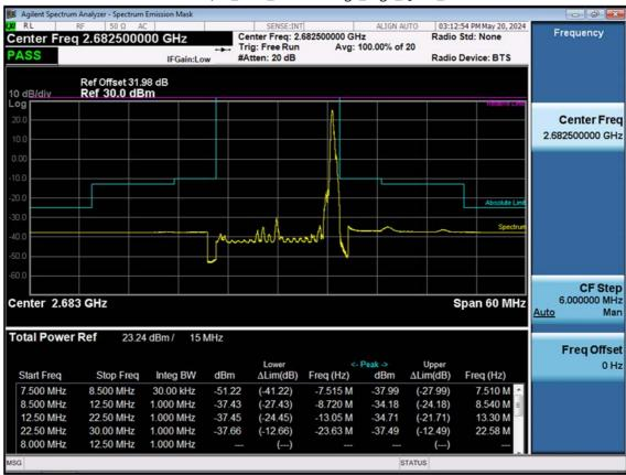
LTE B41/38\_15 M\_Channel Edge\_High\_QPSK\_1RB
