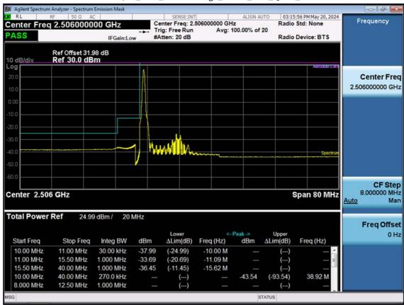
LTE B41/38\_20 M\_Channel Edge\_Lower\_Low\_QPSK\_1RB
