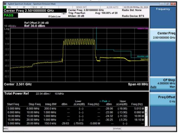
LTE B41/38\_10 M\_Channel Edge\_Upper\_Low\_QPSK\_FullRB
