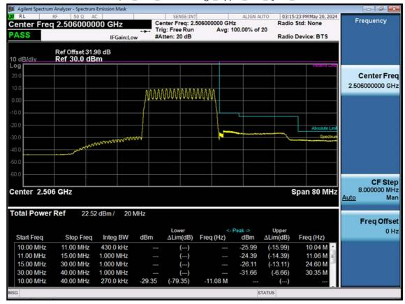
LTE B41/38\_20 M\_Channel Edge\_Upper\_Low\_QPSK\_FullRB
