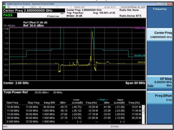
LTE B41/38\_20 M\_Channel Edge\_High\_QPSK\_1RB
