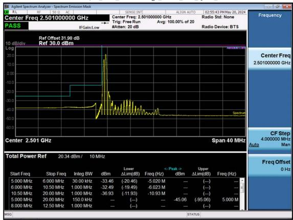
LTE B41/38\_10 M\_Channel Edge\_Lower\_Low\_QPSK\_1RB
