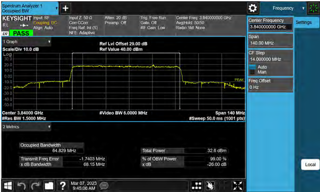
Sub6 n77(78). Occupied Bandwidth Plot (70 M BW Ch.656000 BPSK)
