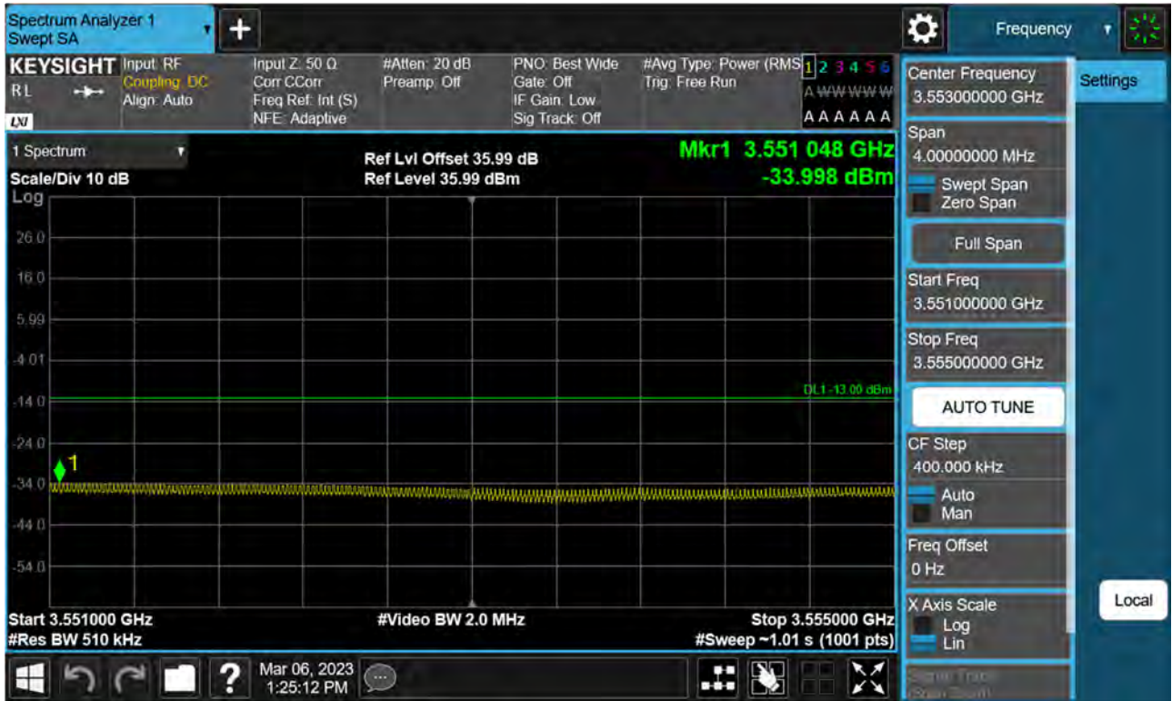
Sub6 n77(78). High Band Edge Plot (60 M BW Ch.634666 BPSK FullRB)(2)
