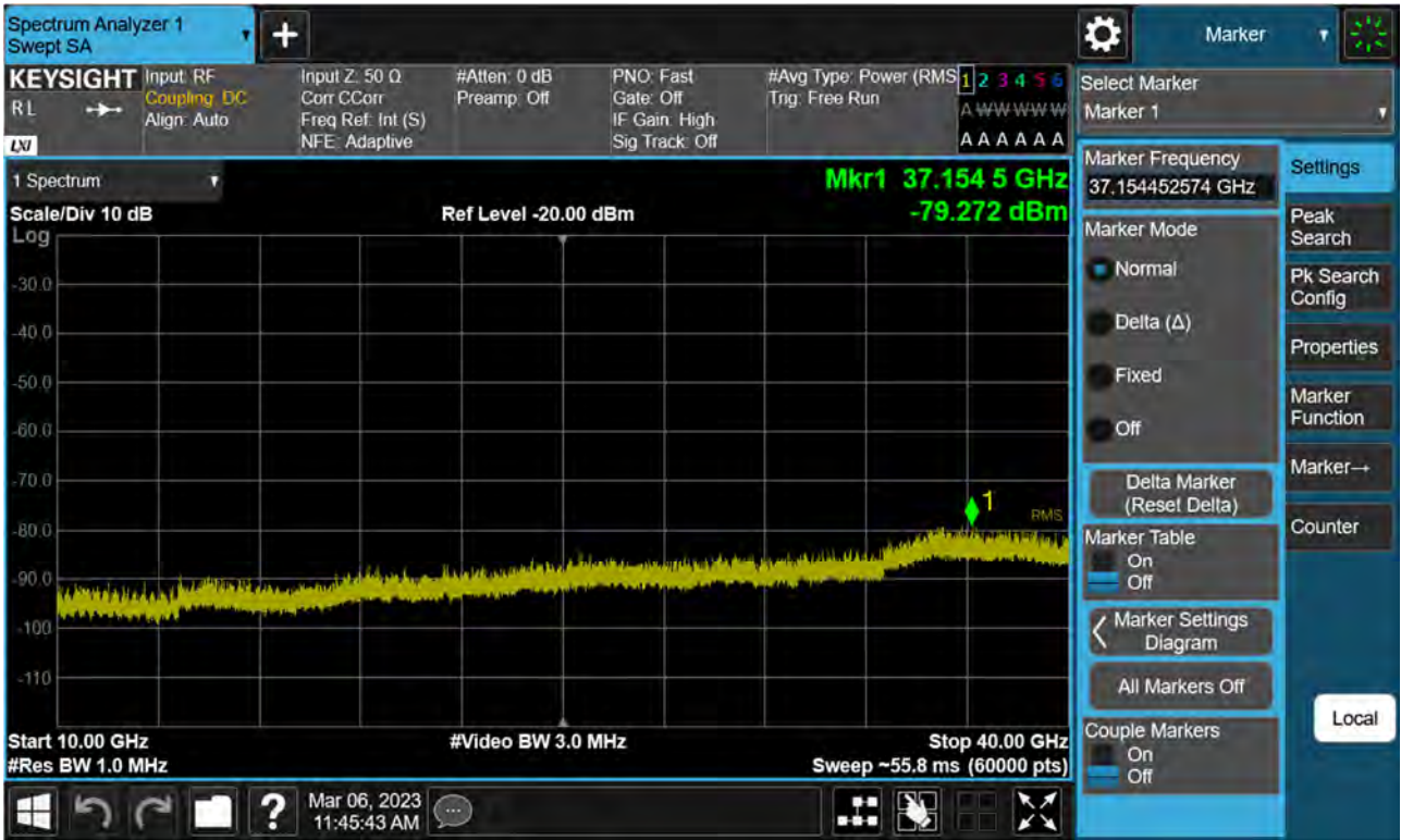
Sub6 n77(78). Conducted Spurious Plot_2 (633334ch_20 MHz_BPSK)
