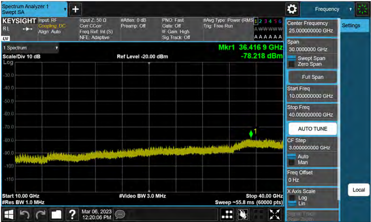
Sub6 n77(78). Conducted Spurious Plot_2 (635332ch_40 MHz_BPSK)
