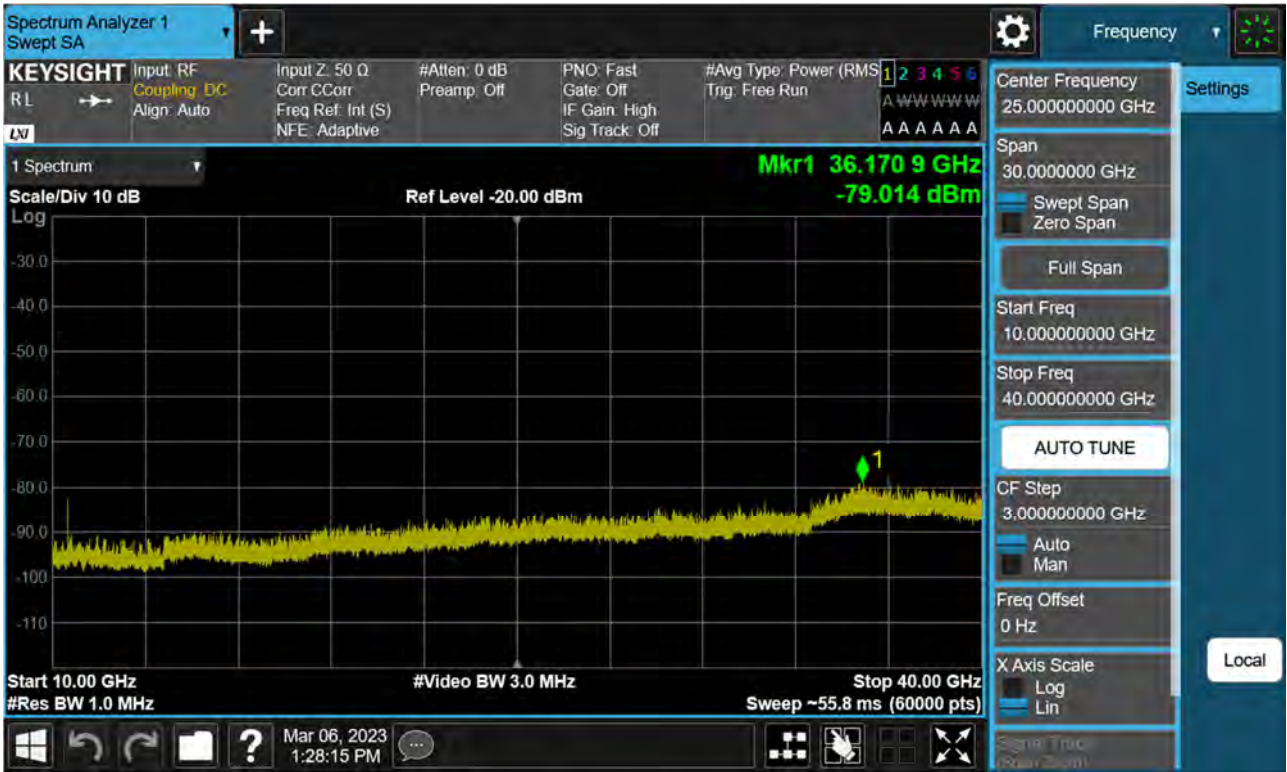
Sub6 n77(78). Conducted Spurious Plot_2 (634666ch_60 MHz_BPSK)
