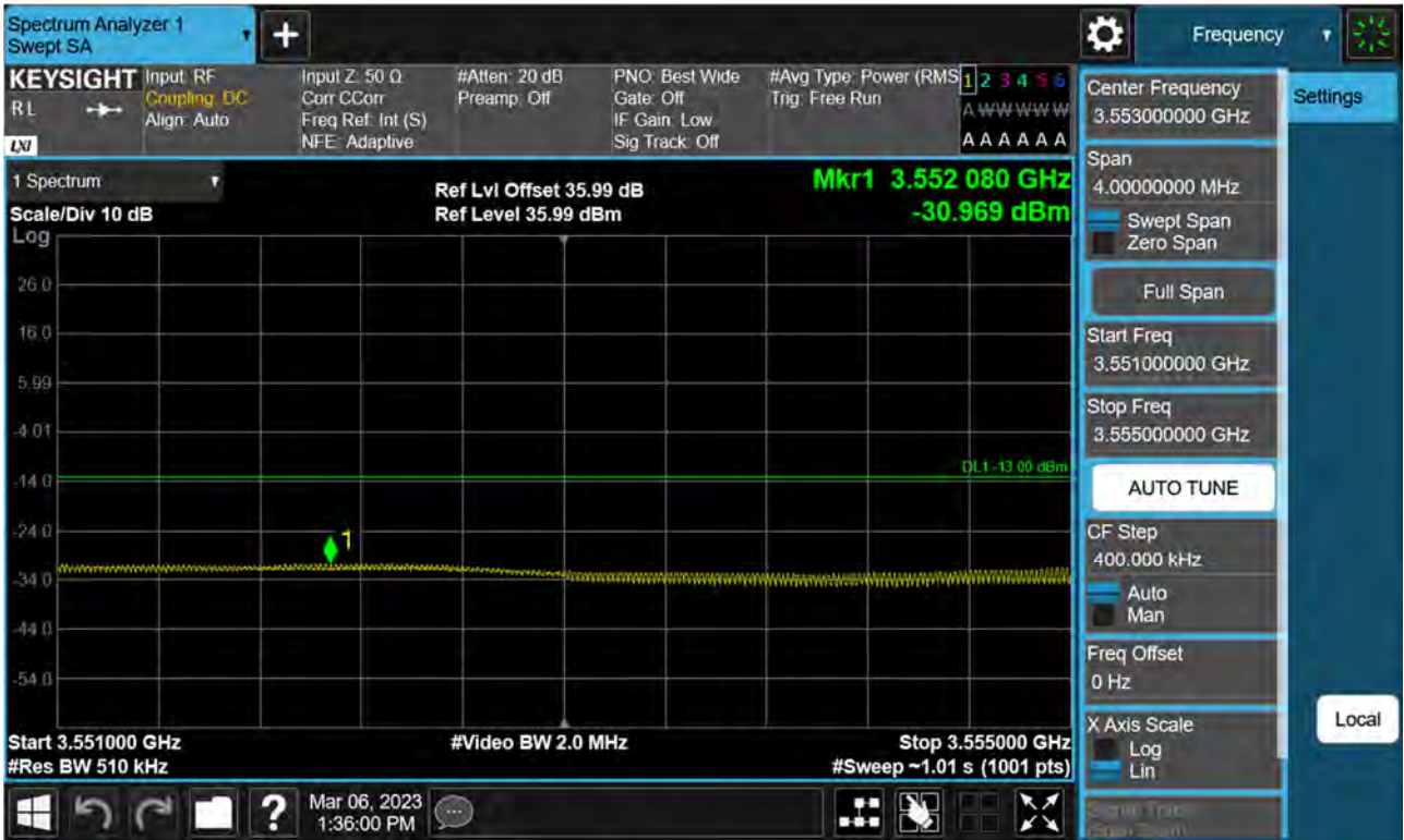
Sub6 n77(78). High Band Edge Plot (70 M BW Ch.634332 BPSK FullRB)(2)
