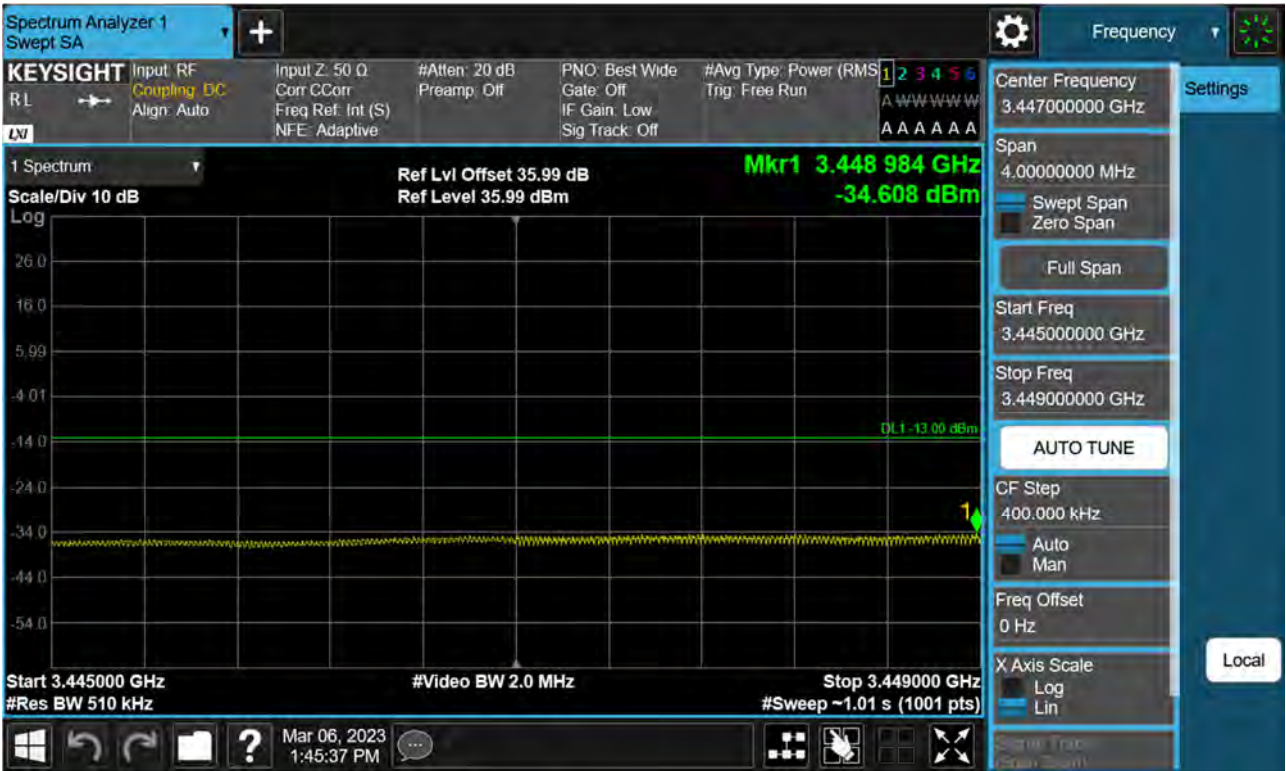
Sub6 n77(78). Low Band Edge Plot (80 M BW Ch.632668 BPSK FullRB)(2)
