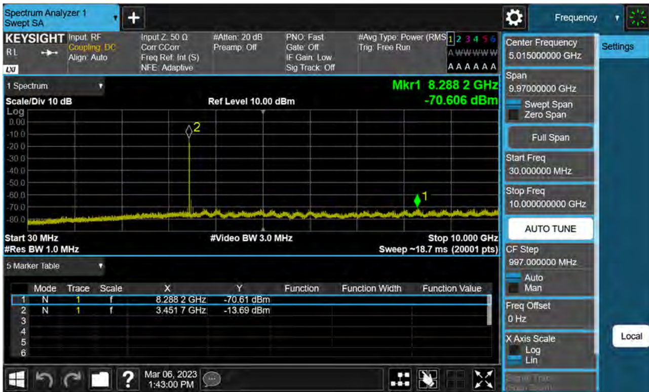
Sub6 n77(78). Conducted Spurious Plot_1 (632668ch_80 MHz_BPSK)
