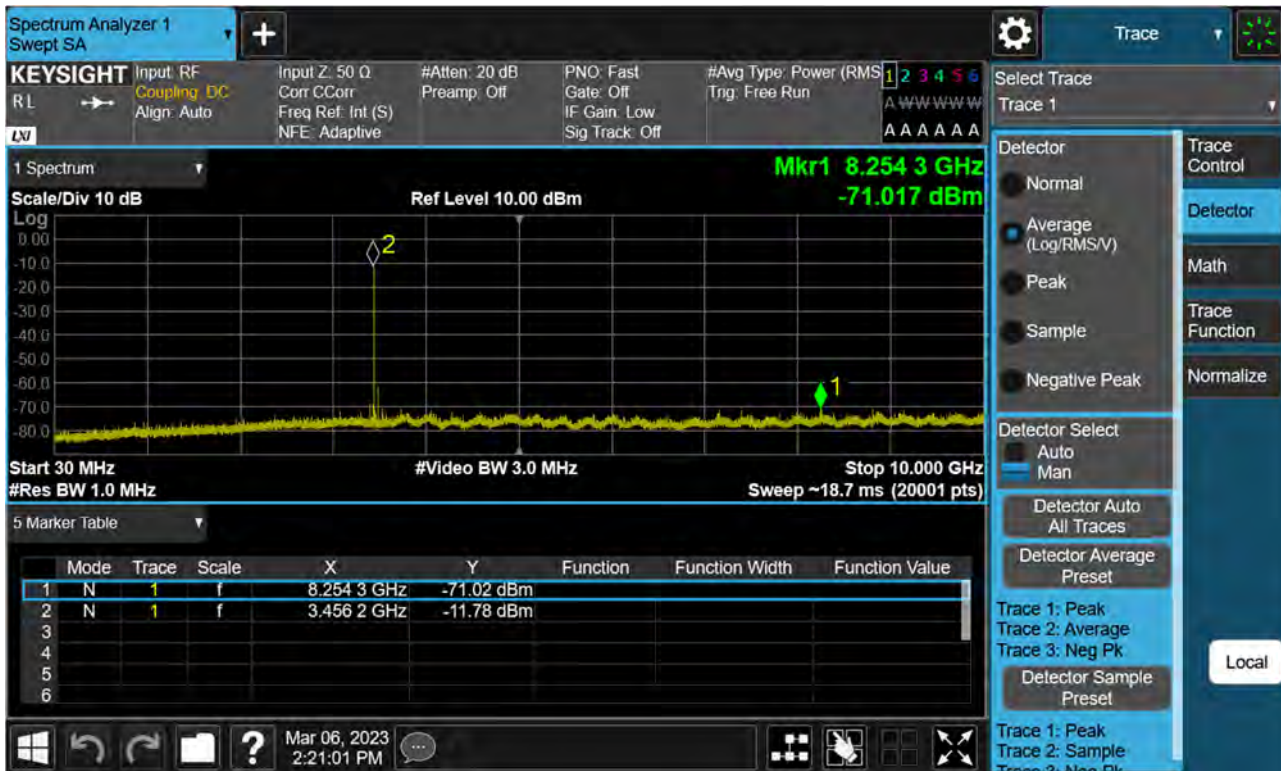
Sub6 n77(78). Conducted Spurious Plot_1 (633334ch_90 MHz_BPSK)
