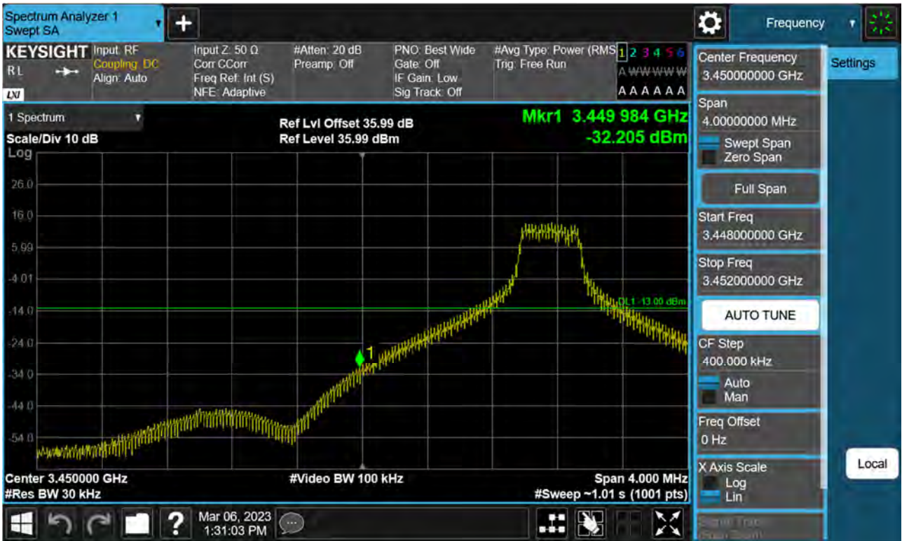
Sub6 n77(78). Low Band Edge Plot (70 M BW Ch.632334 BPSK 1RB)(1)
