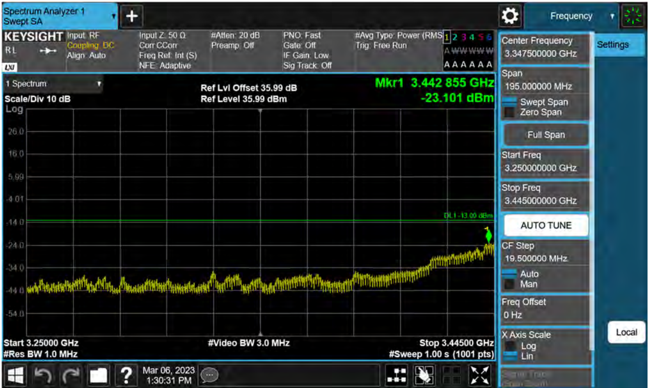
Sub6 n77(78). Low Band Edge Plot (70 M BW Ch.632334 BPSK FullRB)(3)
