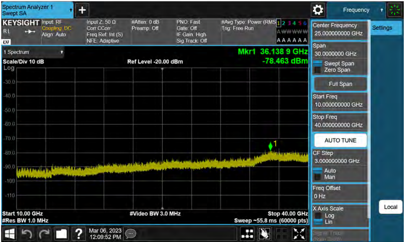
Sub6 n77(78). Conducted Spurious Plot_2 (635666ch_30 MHz_BPSK)
