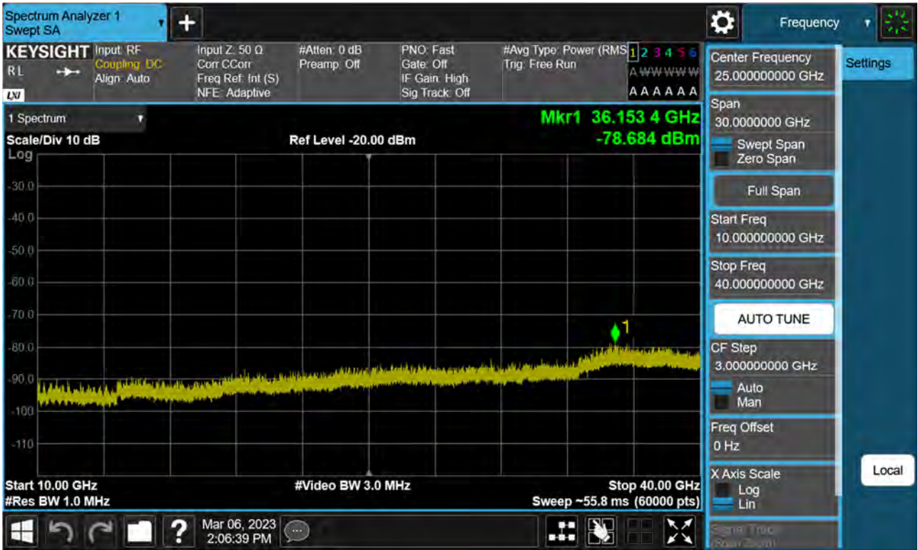
Sub6 n77(78). Conducted Spurious Plot_2 (634000ch_80 MHz_BPSK)
