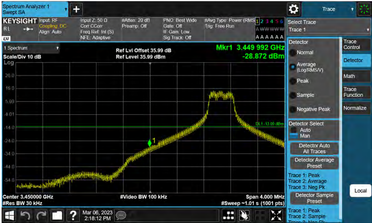
Sub6 n77(78). Low Band Edge Plot (90 M BW Ch.633000 BPSK 1RB)(1)
