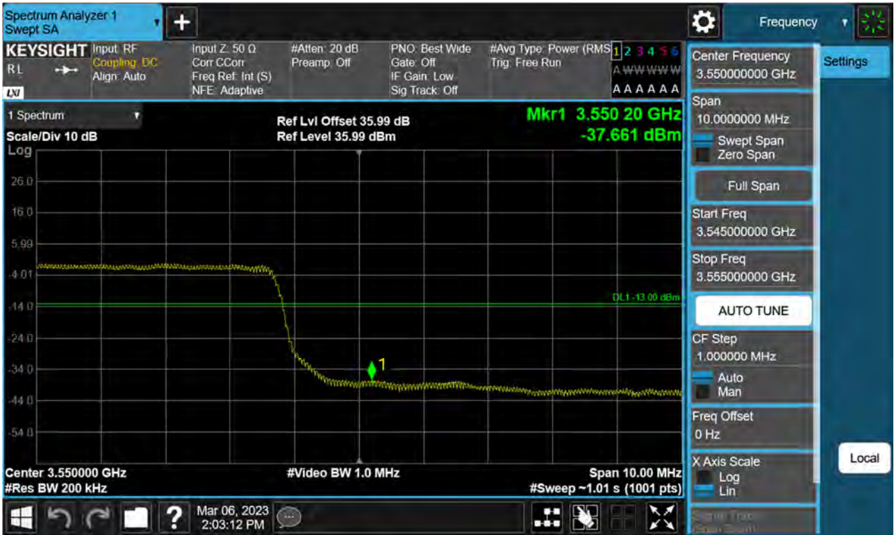
Sub6 n77(78). High Band Edge Plot (80 M BW Ch.634000 BPSK FullRB)(1)
