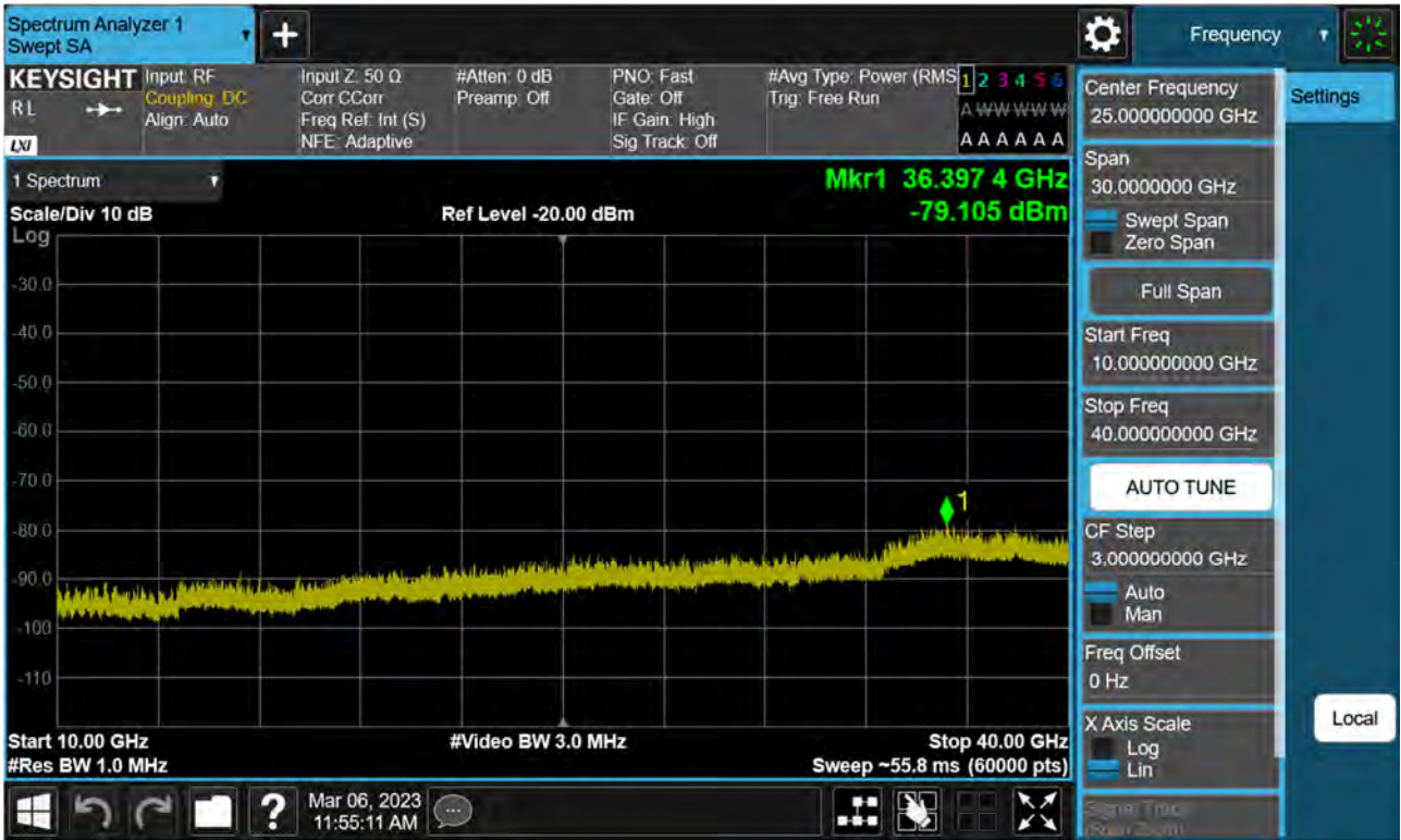
Sub6 n77(78). Conducted Spurious Plot_2 (631000ch_30 MHz_BPSK)
