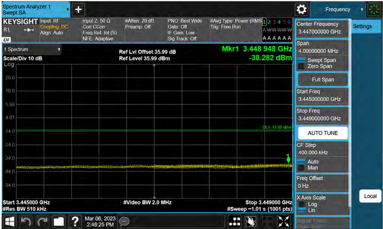
Sub6 n77(78). Low Band Edge Plot (100 M BW Ch.633334 BPSK FullRB)(2)
