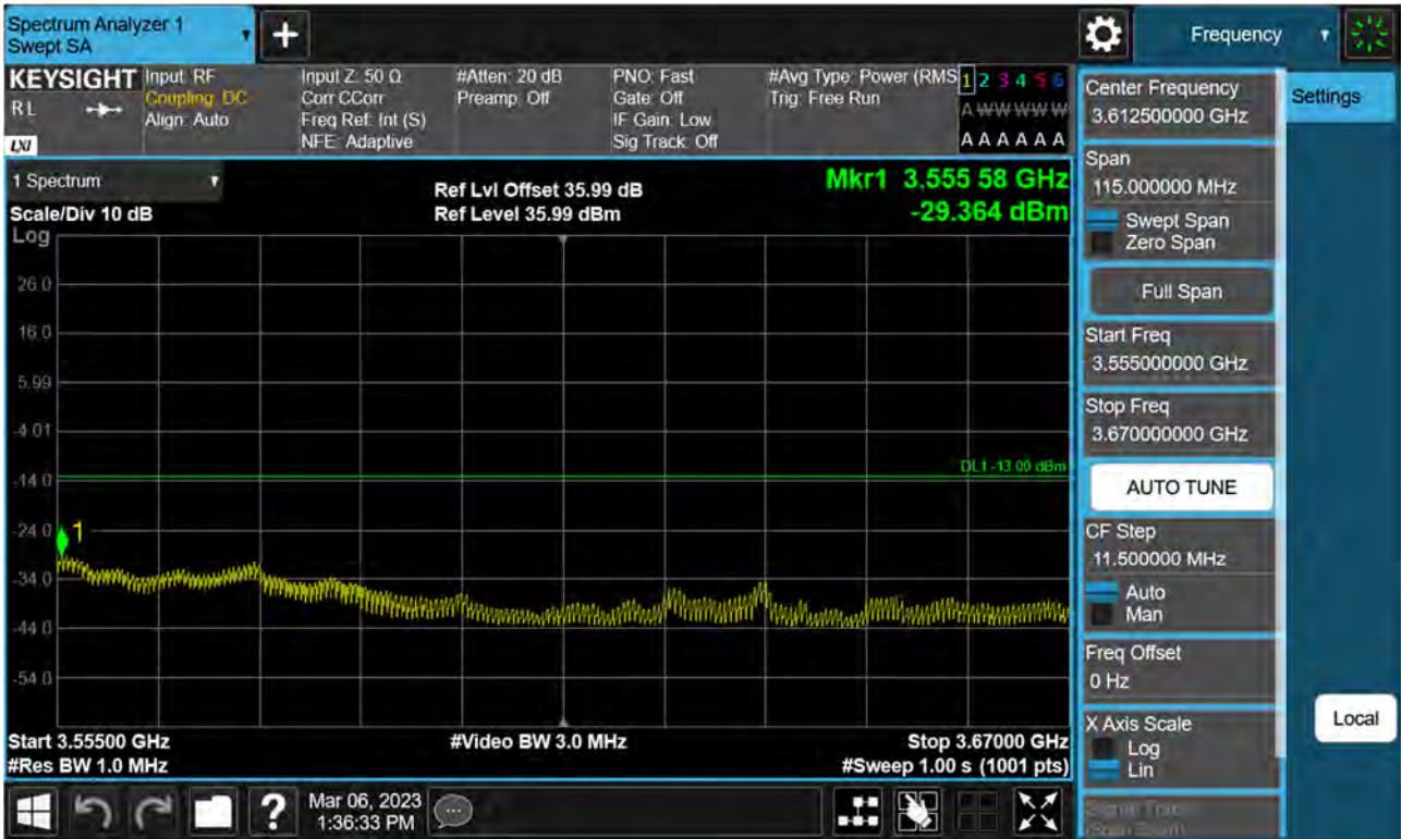
Sub6 n77(78). High Band Edge Plot (70 M BW Ch.634332 BPSK FullRB)(3)
