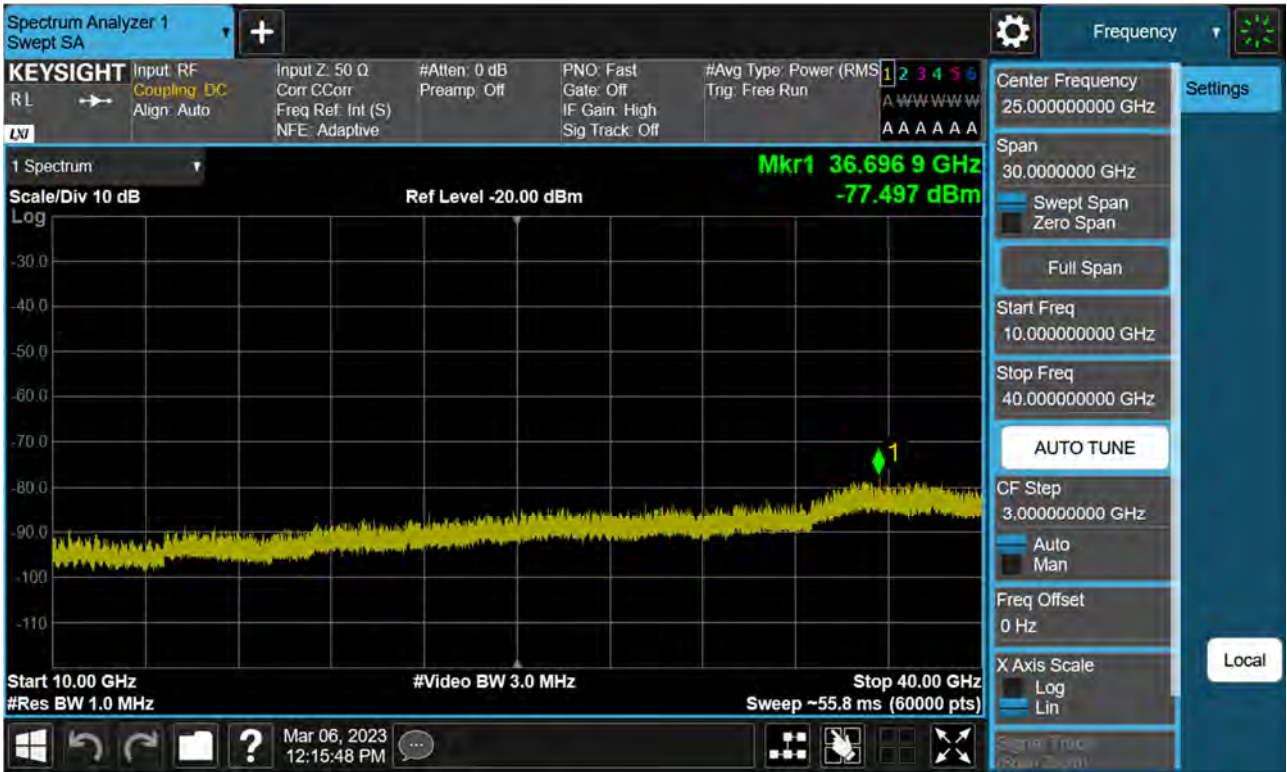
Sub6 n77(78). Conducted Spurious Plot_2 (633334ch_40 MHz_BPSK)
