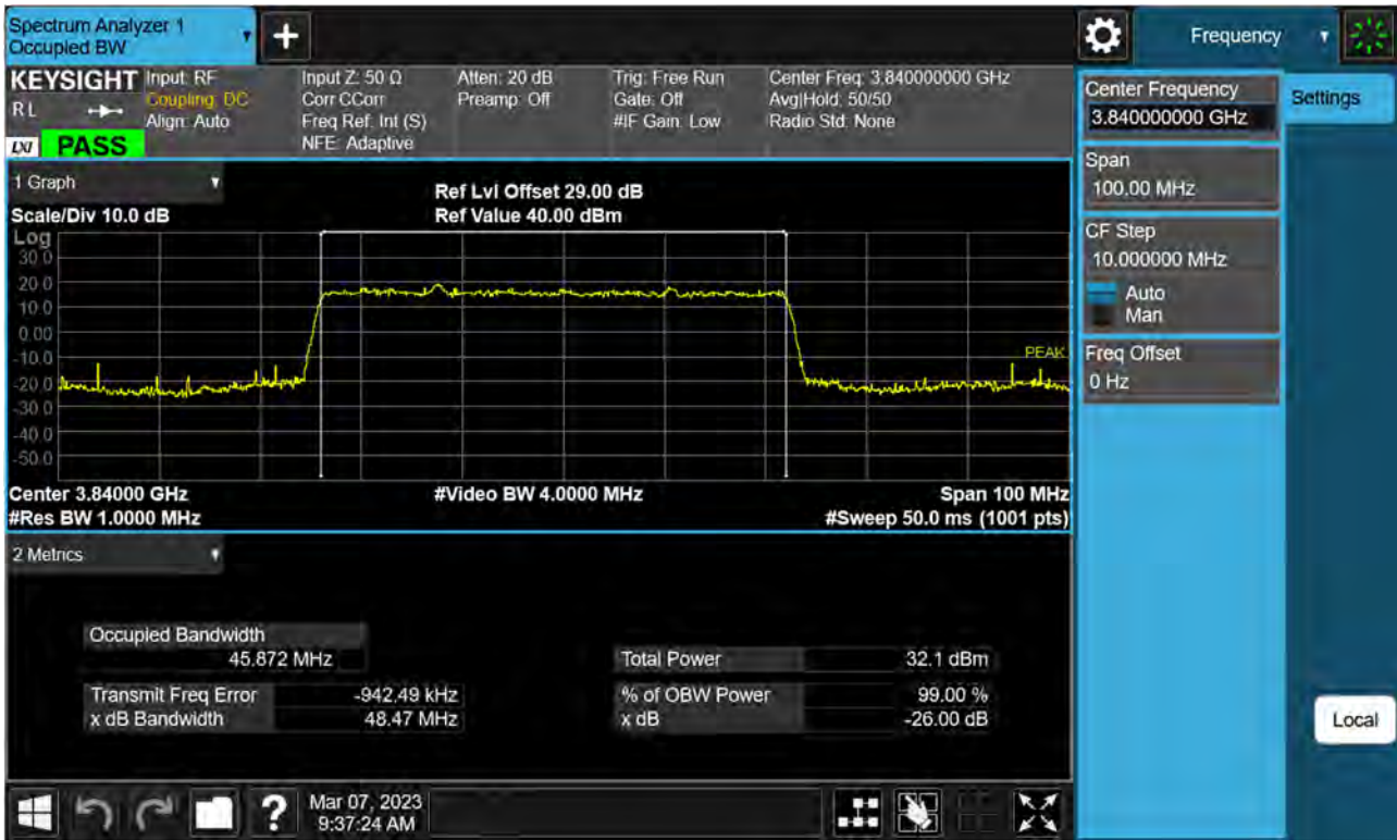
Sub6 n77(78). Occupied Bandwidth Plot (50 M BW Ch.656000 BPSK)
