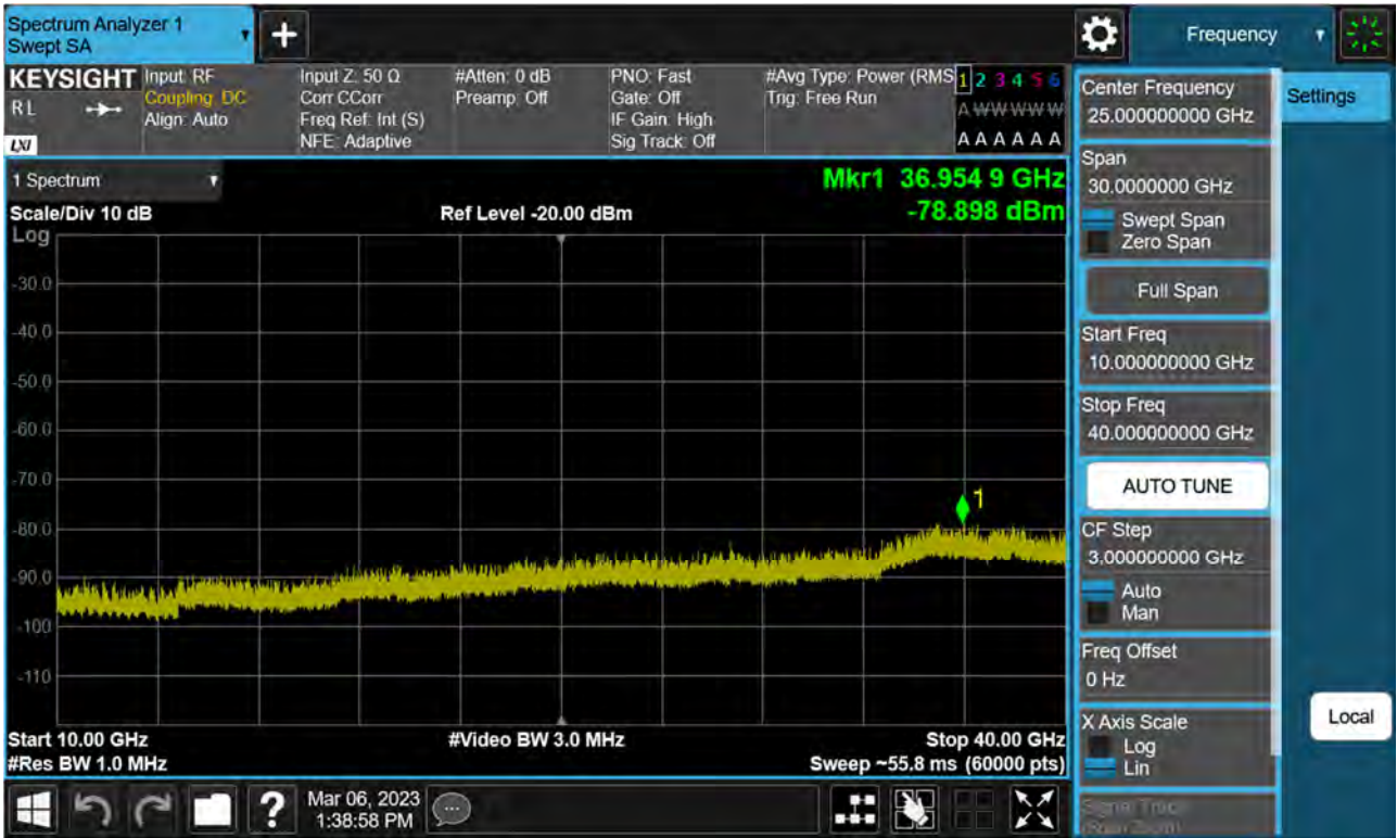
Sub6 n77(78). Conducted Spurious Plot_2 (634332ch_70 MHz_BPSK)
