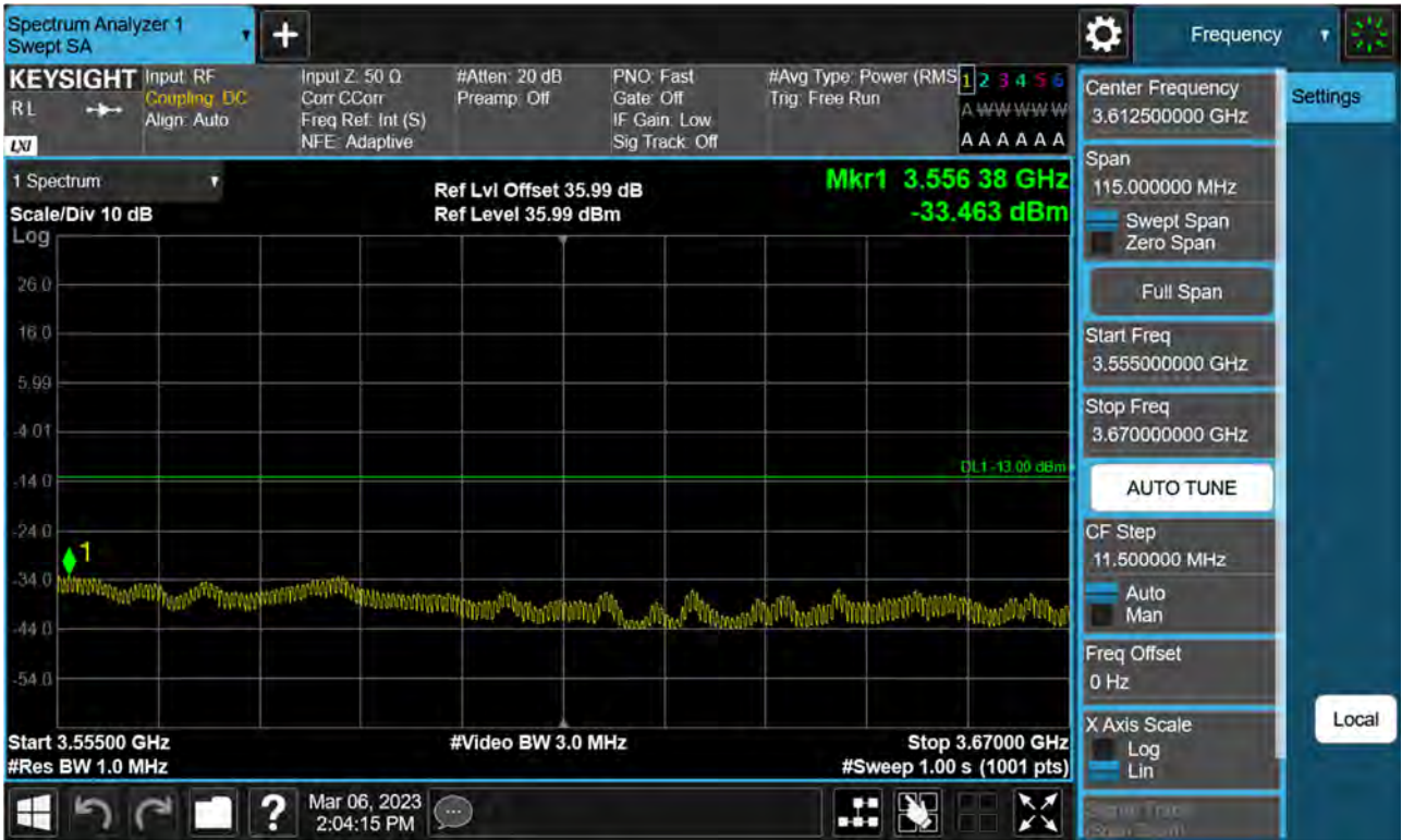
Sub6 n77(78). High Band Edge Plot (80 M BW Ch.634000 BPSK FullRB)(3)
