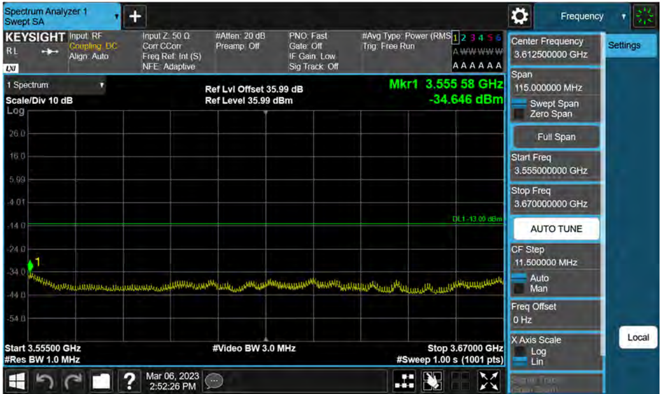
Sub6 n77(78). High Band Edge Plot (100 M BW Ch.633334 BPSK FullRB)(3)
