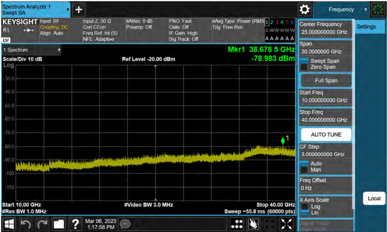
Sub6 n77(78). Conducted Spurious Plot_2 (635000ch_50 MHz_BPSK)
